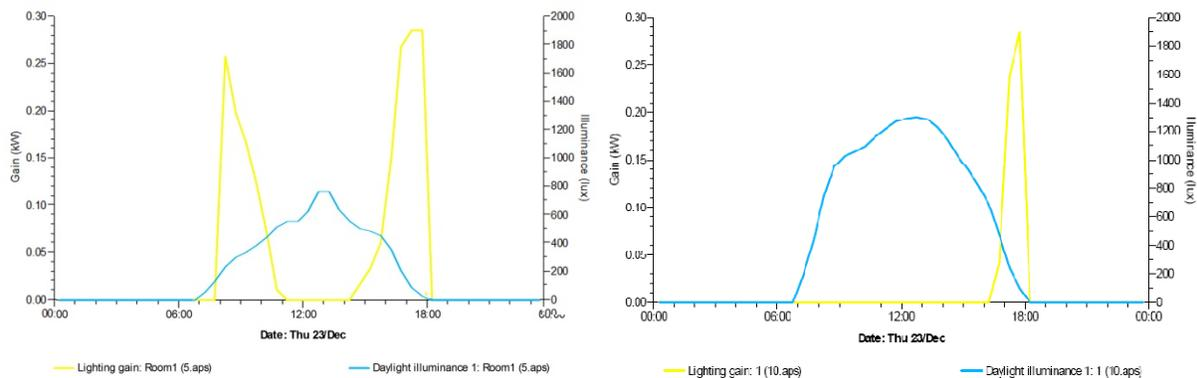
Figure 5.1 Lighting gain relative to daylight illuminance on December 23 for BIPV case no. 5 (left) and no. 10 (right)
