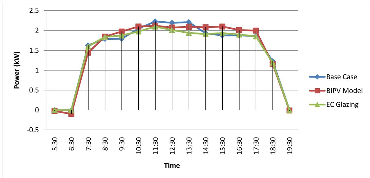
Figure A.17 Hourly Energy Consumption for all configurations for North façade in June 21 with glass of 0.27 shading coefficient and lighting sensor @ 2m
