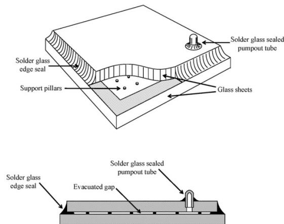
Figure 2.3 Schematic of evacuated glazing (Fang et al., 2007)
