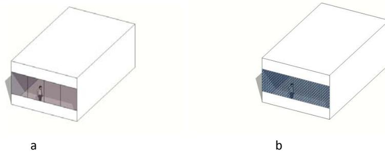
Figure 3.5 EC glazing replacing conventional glass (a); BIPV cells within the vision glass (b)
