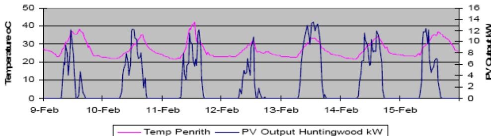
Figure 2.48 Effect of temperature on power output of PV array (Chaar et al., 2008)
