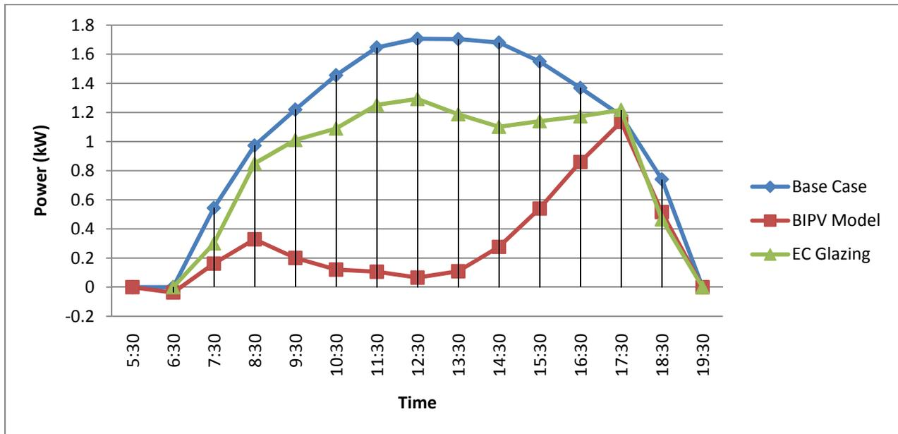
Figure A.6 Hourly Energy Consumption for all configurations for South façade in March 21 with glass of 0.27 shading coefficient and lighting sensor @ 4m
