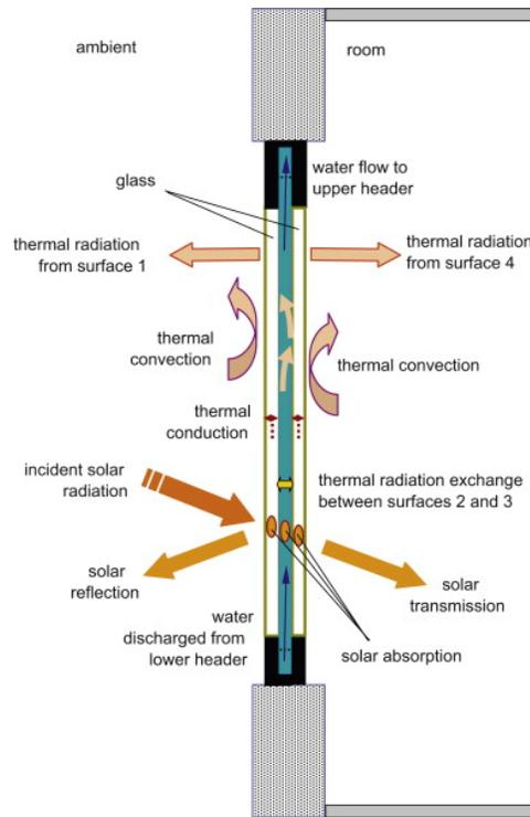
Figure 2.8 Energy flow paths at water-flow double-pane window (Chow, 2010)
