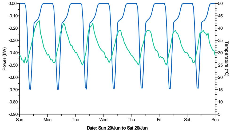
Figure 5.41 Effect of temperature on power output of PV for one week in June for East façade
