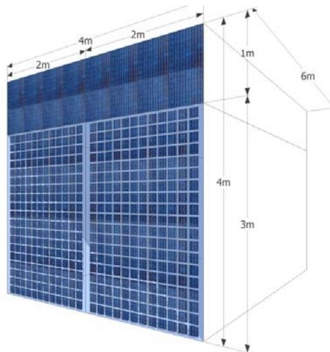
Figure 4.26 BIPV case 5 combines semitransparent and opaque mono-crystalline PV cells on facade
