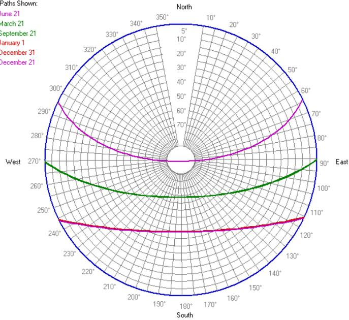
Figure 4.18 Sun Path diagram for Abu Dhabi (IES Database)
