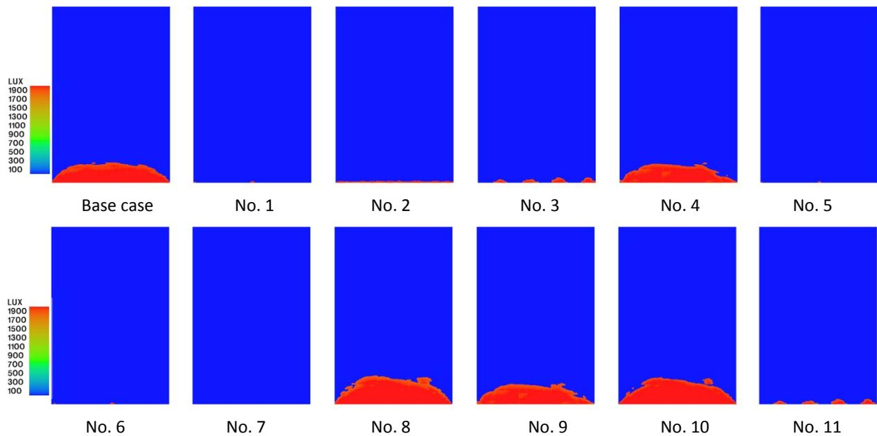
Figure 5.3 Working plane glare levels on December 23 at 12pm for ten BIPV cases and base case
