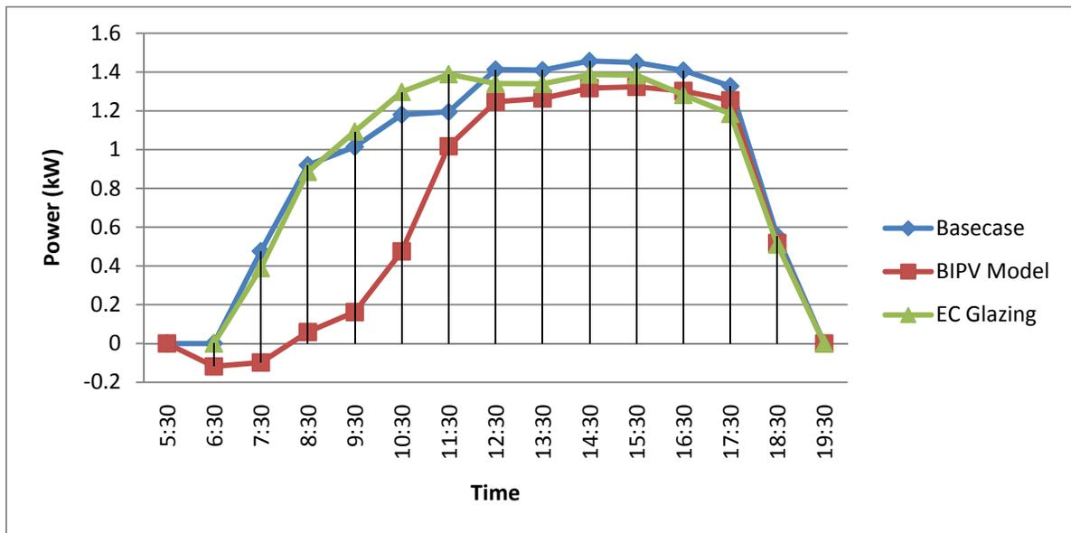
Figure A.8 Hourly Energy Consumption for all configurations for East façade in March 21 with glass of 0.27 shading coefficient and lighting sensor @ 2m
