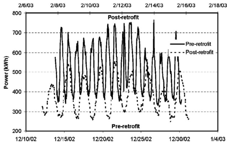
Figure 2.50 Pre- and post-retrofit period chiller power monitoring (Yalcintas and Kaya, 2009)
