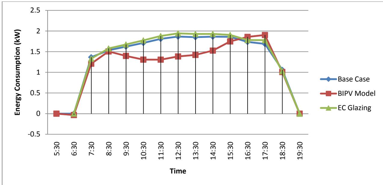
Figure 5.13 Hourly Energy Consumption for all configurations for South façade in September 21
