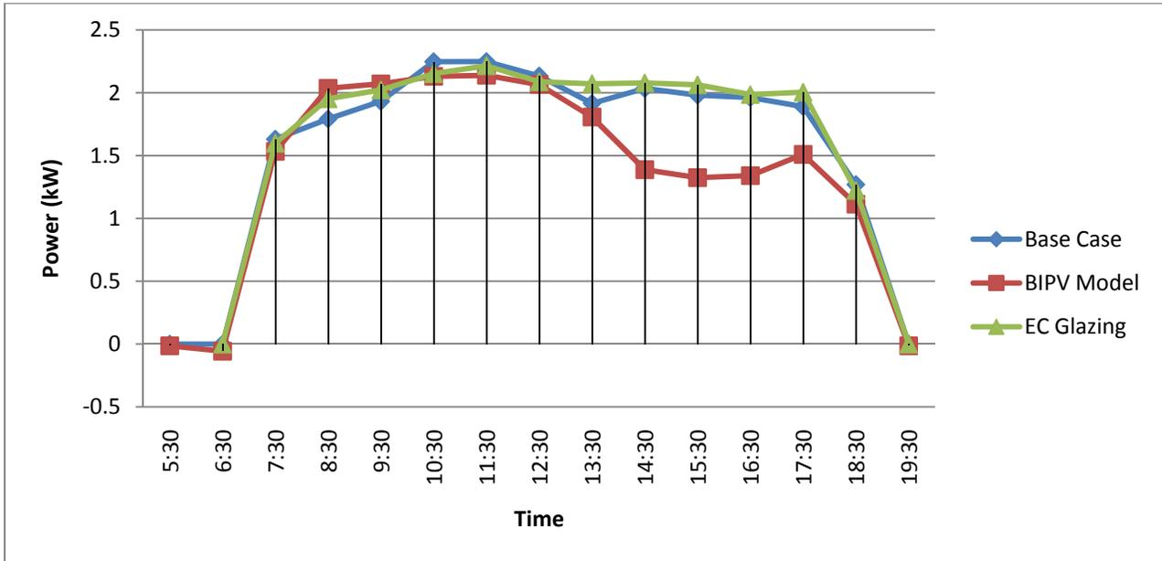
Figure A.13 Hourly Energy Consumption for all configurations for West façade in June 21 with glass of 0.27 shading coefficient and lighting sensor @ 2m
