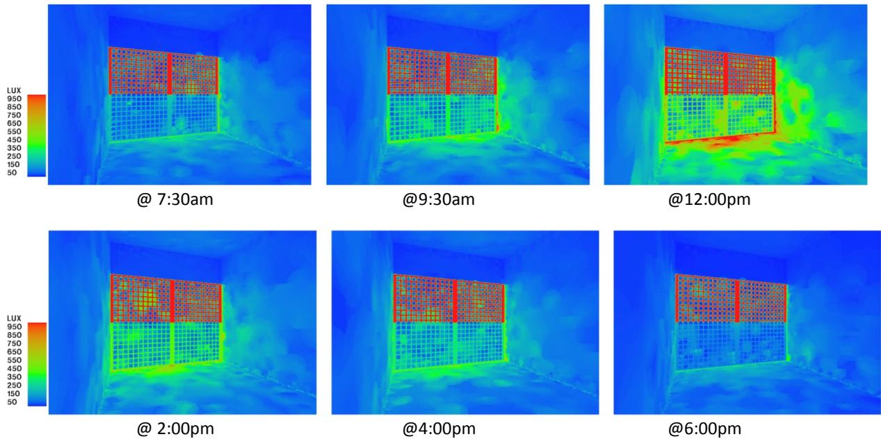
Figure 6.2 Illuminance levels of BIPV model South facing window on June 21 under clear skies
