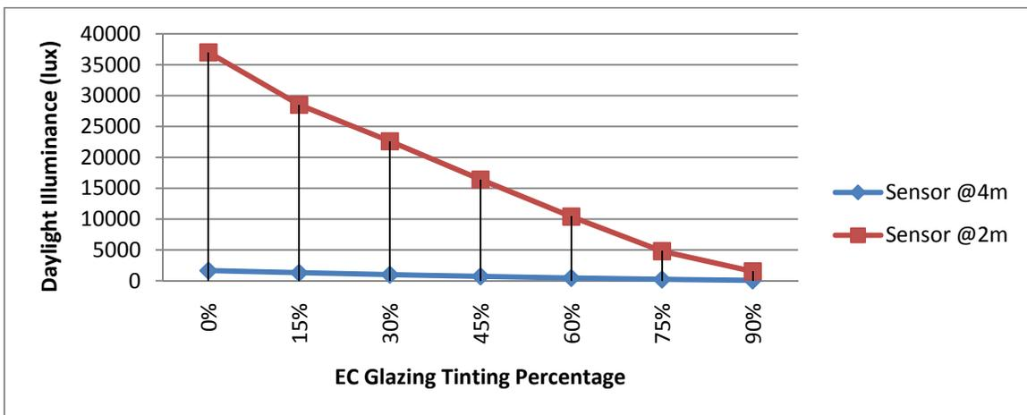
Figure 5.29 Daylight illuminance ratio compared to tinting percentage for South façade in September 21
