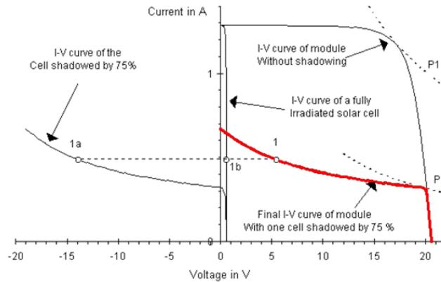
Figure 2.47 I-V curve of module with one cell shaded by 75% (Chaar et al., 2008)
