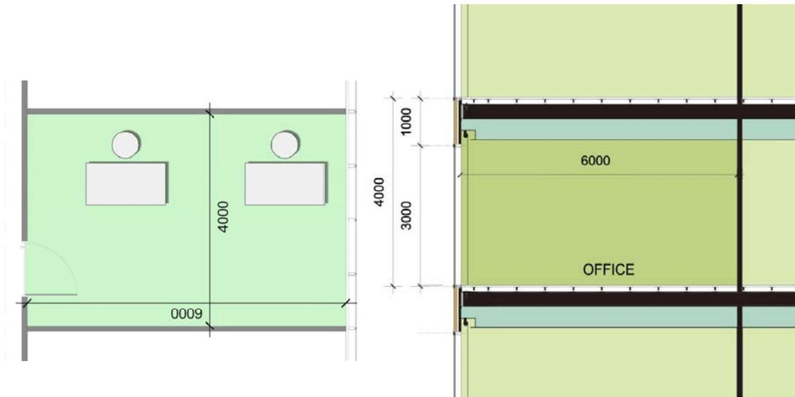
Figure 4.2 Floor Plan (left) and section (right) of the simulation model
