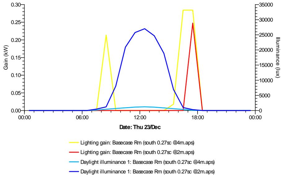
Figure 5.23 Comparison of effect of sensor relocation from 2m to 4m on the lighting gain in December
