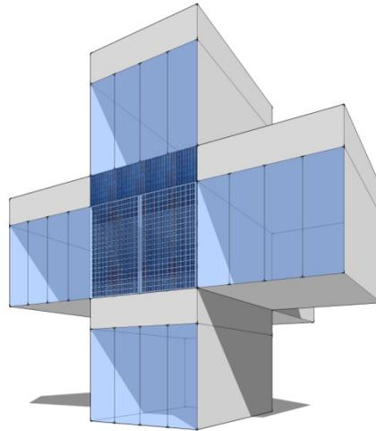
Figure 4.27 Model #3: Conventional façade replaced by BIPV
