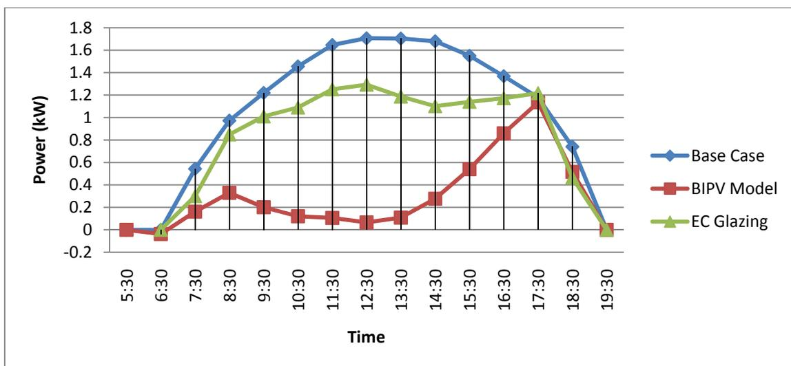
Figure A.1 Hourly Energy Consumption for all configurations for South façade in June 21 with glass of 0.6 shading coefficient and lighting sensor @ 2m
