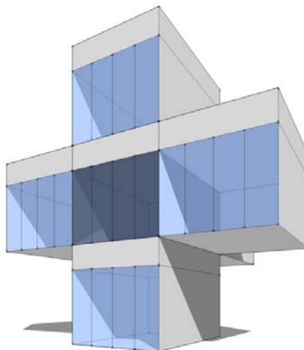
Figure 4.28 Model #2: Conventional glass replaced by EC glazing
