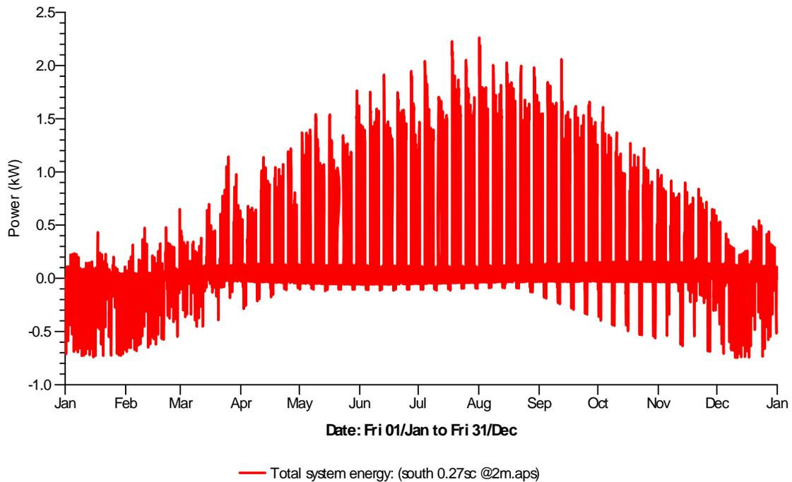
Figure 5.20 Annual BIPV model total system energy for the South façade with glass shading coefficient of 0.27
