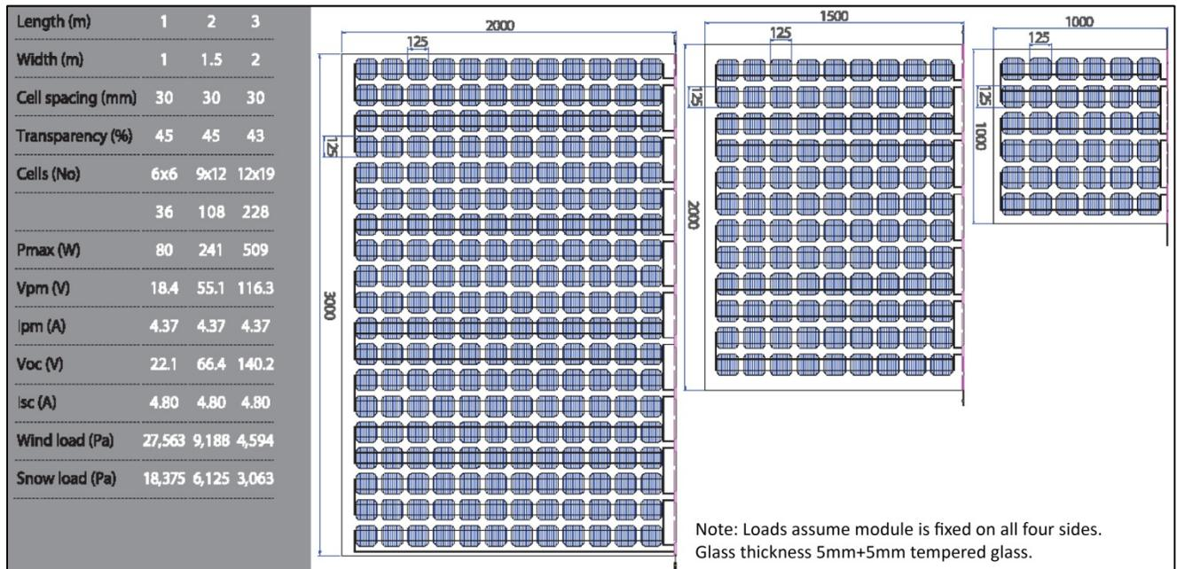
Figure 4.7 Technical specifications of semi-transparent mono-crystalline PV cells (Suntech, 2010)
