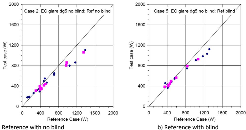
Figure 2.31 Field measured hourly peak cooling load due to heat gains compared to reference case without (a) or with (b) fully lowered Venetian blinds (Lee et al., 2006)
