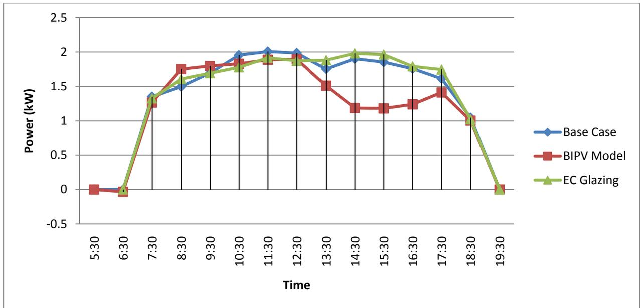
Figure A.14 Hourly Energy Consumption for all configurations for West façade in September 21 with glass of 0.27 shading coefficient and lighting sensor @ 2m
