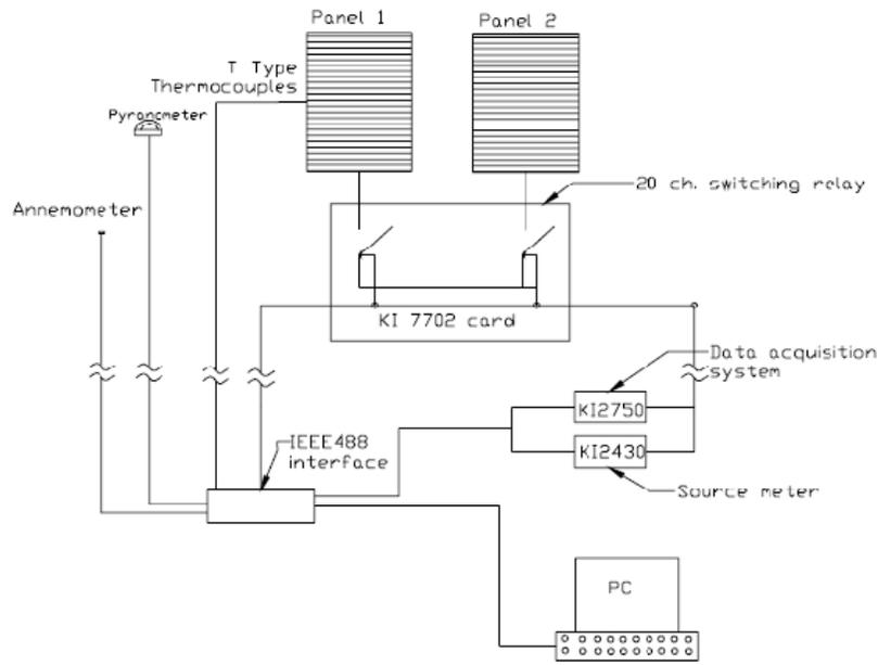
Figure 3.1 Block diagram of equipment used for characterizing PV systems (Mallick et al., 2005)
