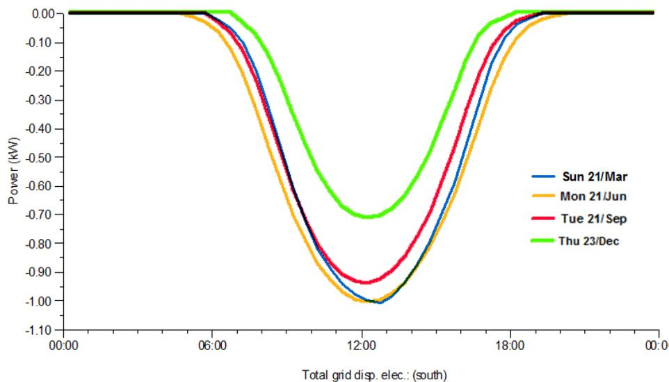
Figure 5.19 Power production of the BIPV model in the four design days for the South façade
