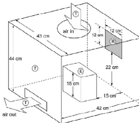
Figure 3.3 Schematic of the test-cell showing sensor locations (Piccolo, 2009)
