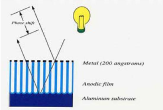
Figure 2.7 Schematic of interference coloring mechanism (Ball, 2005)
