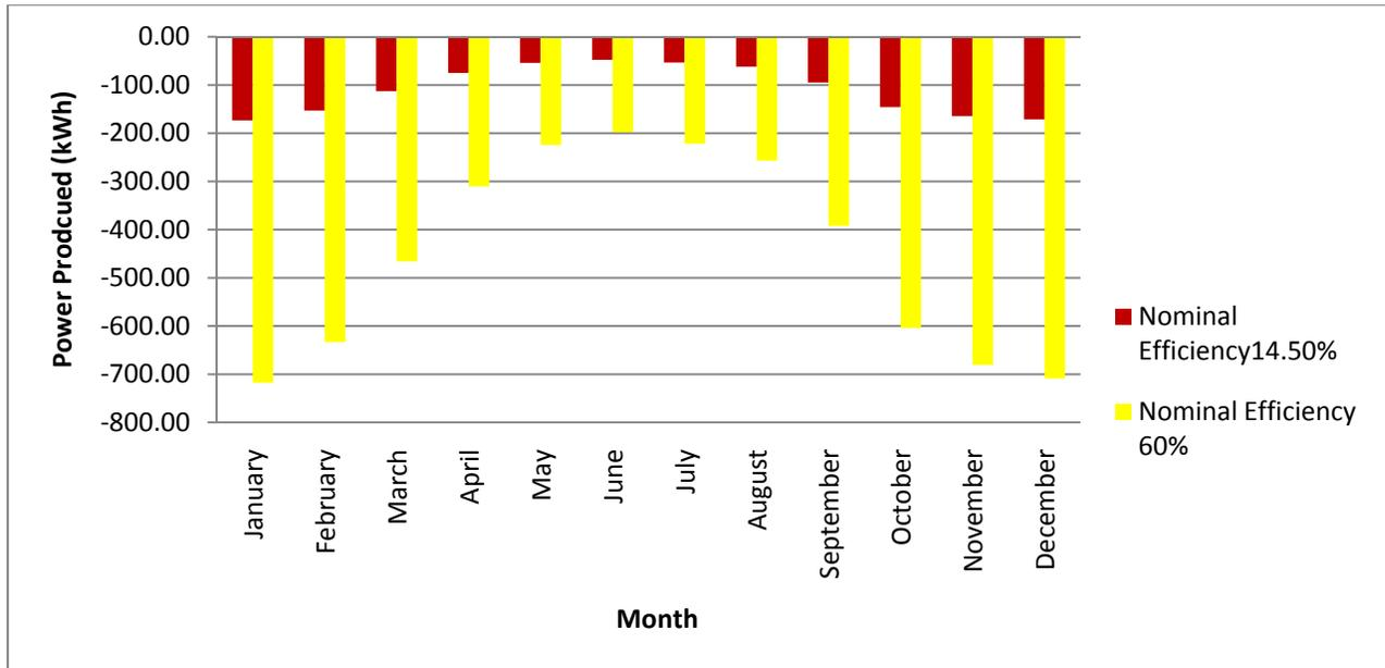
Figure 6.3 Annual power productions of BIPV models with different nominal efficiency for South orientation
