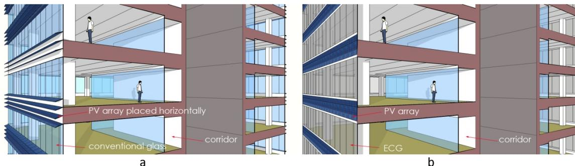
Figure 7.2 PV array placed horizontally on the façade (a) and combined with EC glazing (b)
