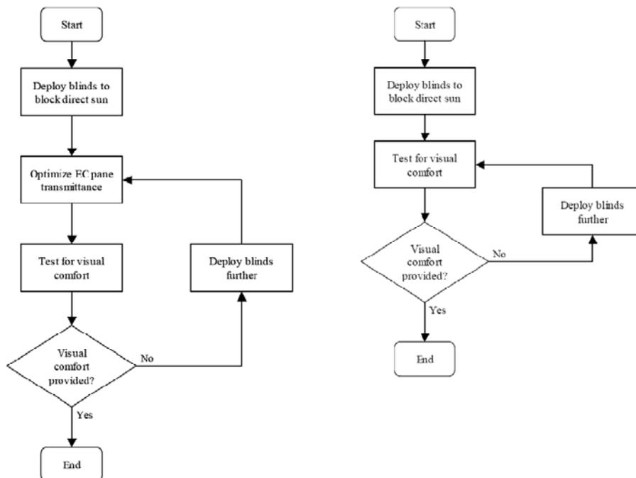
Figure 2.33 EC case (left) and reference case (right) control algorithm flow charts (Fernandes et al., 2006)
