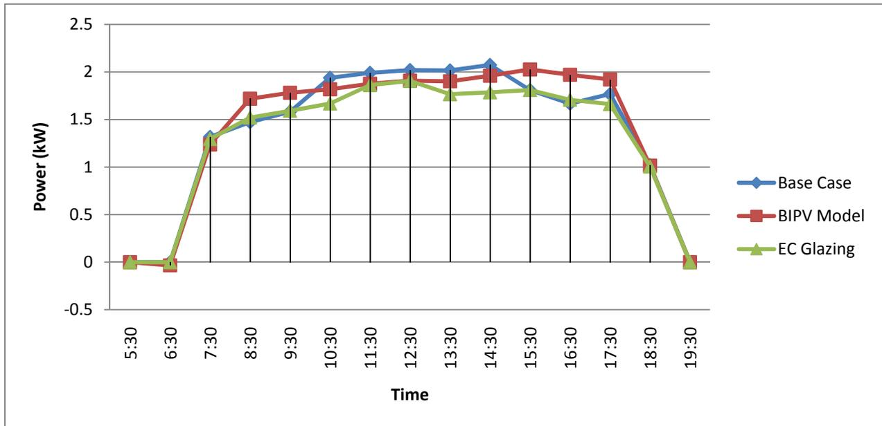
Figure A.18 Hourly Energy Consumption for all configurations for North façade in September 21 with glass of 0.27 shading coefficient and lighting sensor @ 2m
