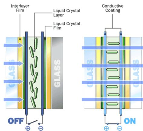
Figure 2.23 Liquid Crystal Window working mechanism (Bonsor, 2010)
