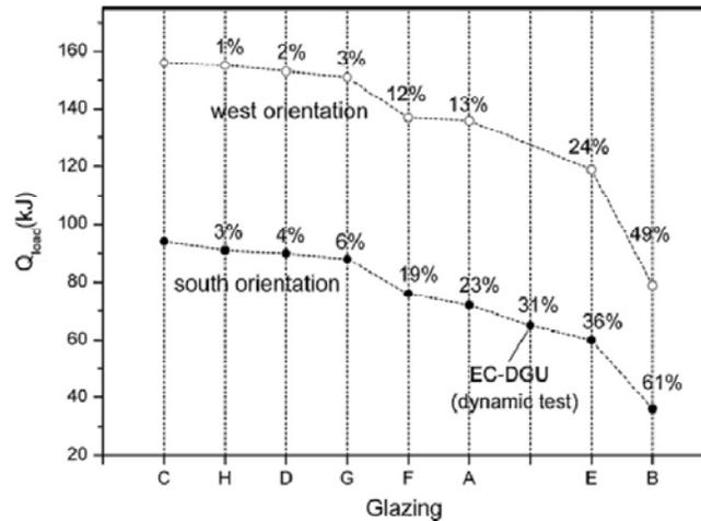
Figure 2.39 Heat loads affecting the test-cell for various glazing (Piccolo, 2010)
