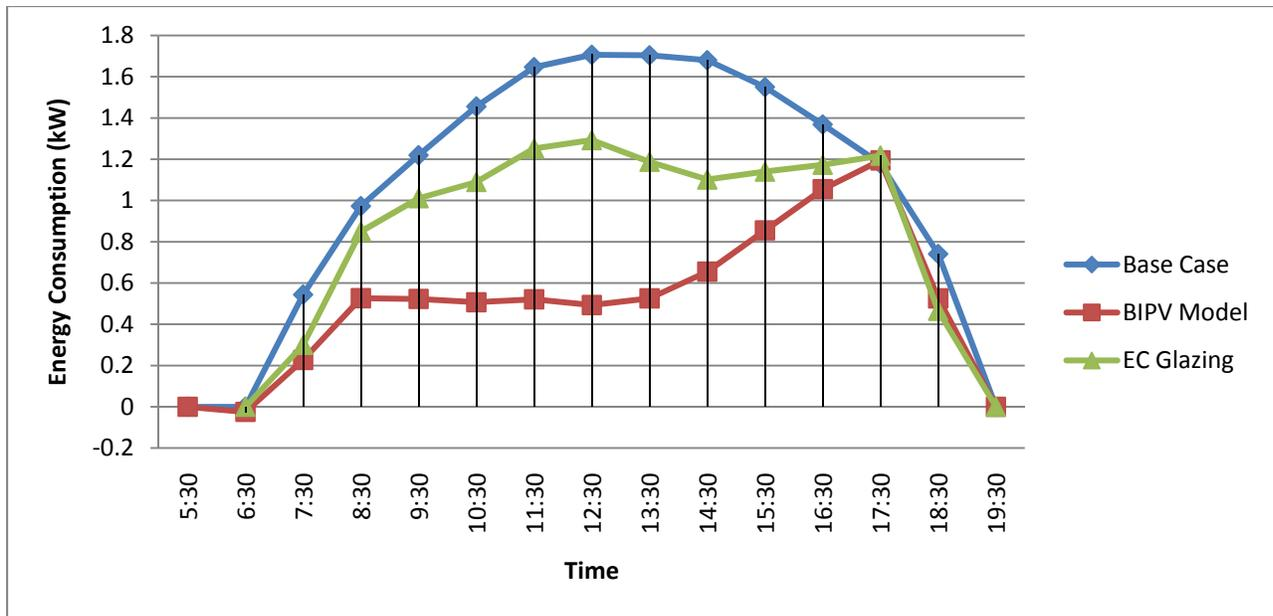
Figure 5.21 Hourly Energy Consumption for all configurations for South façade in March 21 with glass of 0.6 shading coefficient and lighting sensor @ 2m
