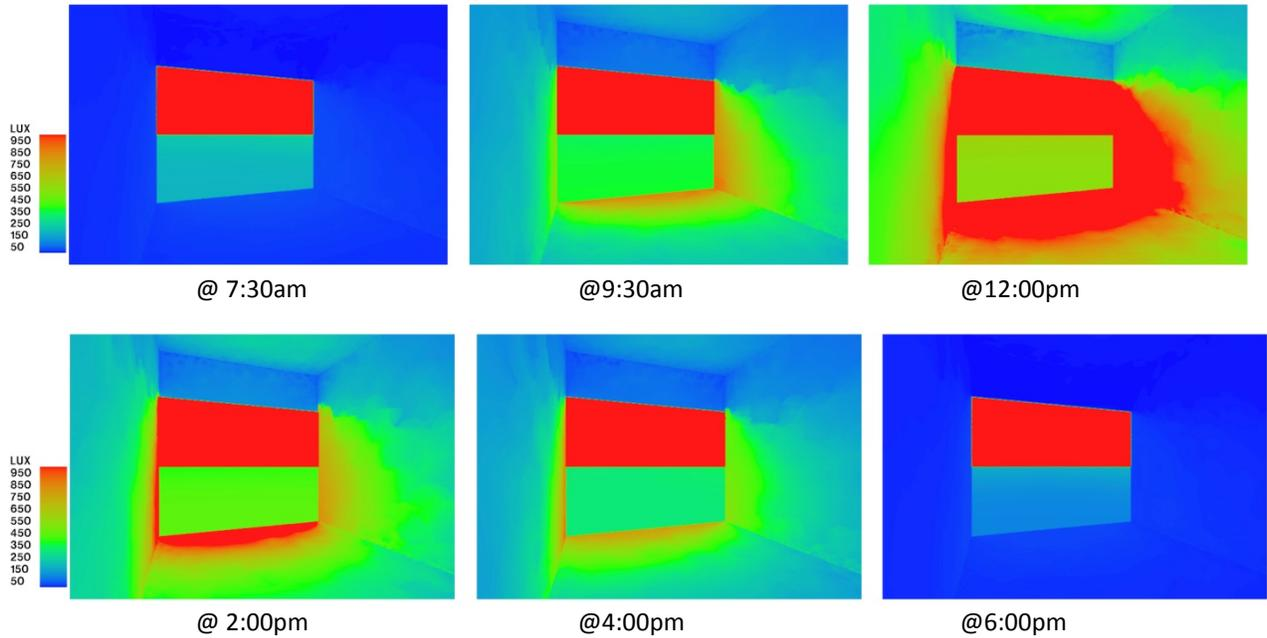
Figure 6.1 Illuminance levels of dynamic EC glazing model South facing window on June 21 under clear skies
