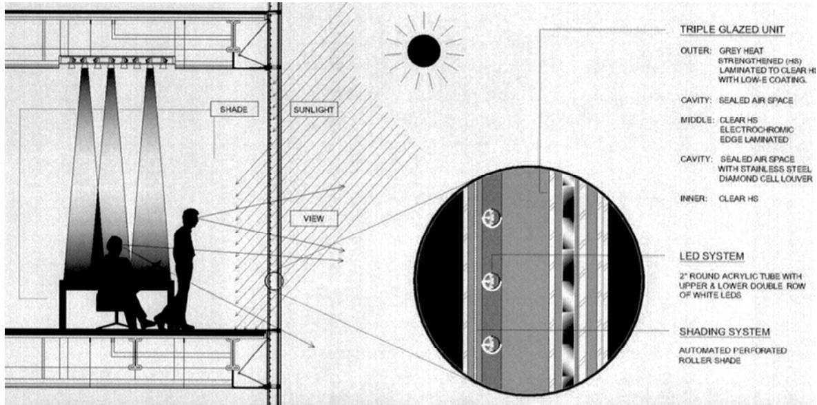
Figure 2.27 LED EC wall in daytime mode (Lighting Design + Application, 2006)
