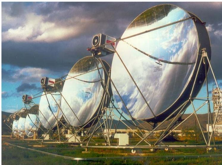
Figure 2.14 Dish engine systems eliminate the need to transfer heat to a boiler by placing a Stirling engine at the focal point (Wikipedia, 2010)
