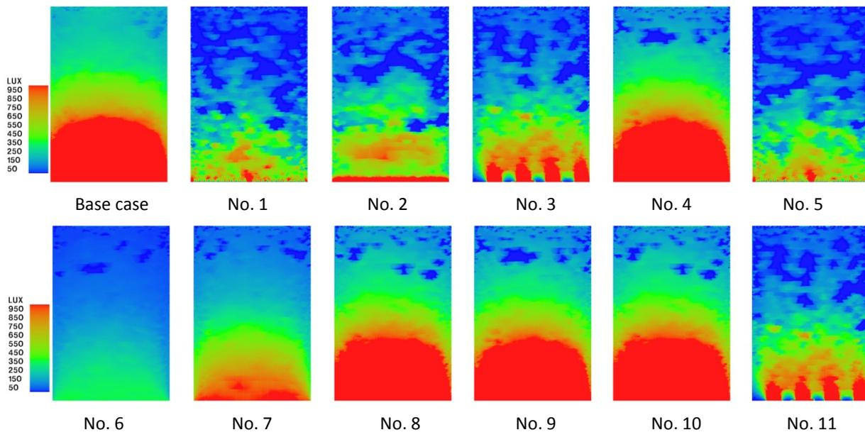
Figure 5.2 Working plane illuminance levels on December 23 at 12pm for BIPV cases and base case
