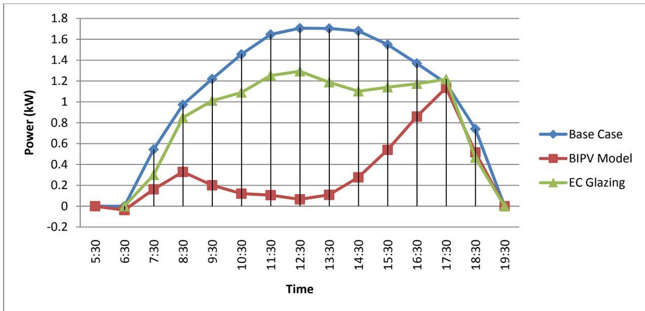
Figure A.7 Hourly Energy Consumption for all configurations for South façade in December 23 with glass of 0.27 shading coefficient and lighting sensor @ 4m
