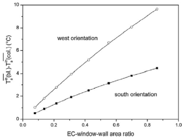
Figure 2.38 Mean differences between the internal air temperatures relative to full bleached and full colored states as a function of window/front-wall ratio (Piccolo, 2010)
