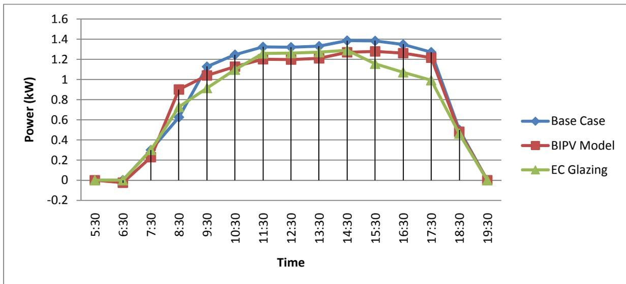
Figure A.16 Hourly Energy Consumption for all configurations for North façade in March 21 with glass of 0.27 shading coefficient and lighting sensor @ 2m
