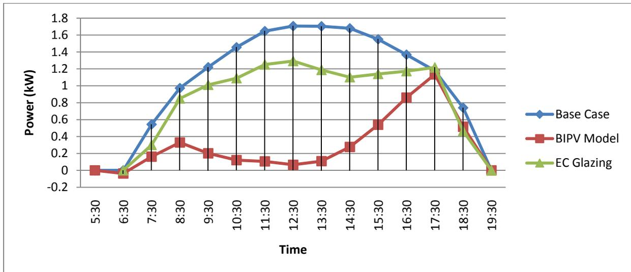
Figure A.4 Hourly Energy Consumption for all configurations for South façade in March 21 with glass of 0.27 shading coefficient and lighting sensor @ 4m
