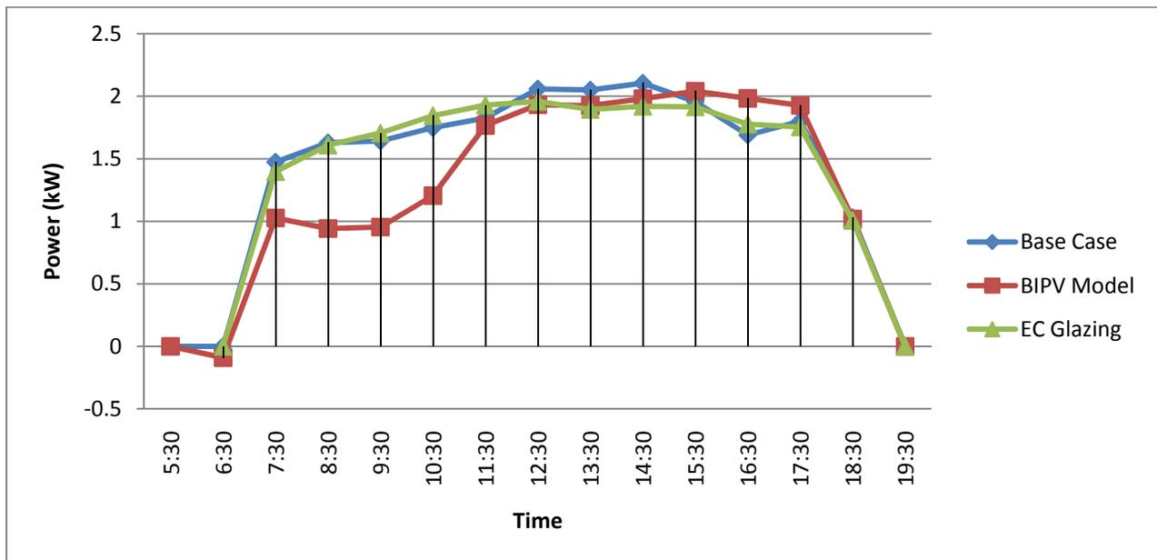
Figure A.10 Hourly Energy Consumption for all configurations for East façade in September 21 with glass of 0.27 shading coefficient and lighting sensor @ 2m
