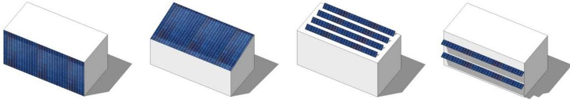
Figure 2.17 Applications of PV in buildings: façade (a), Sloped roof(b), Flat roof (c), and Awning (d)
