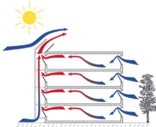
Figure 2.1 Schematic of double-façade system (Dyer Environmental Controls Ltd., 2010)
