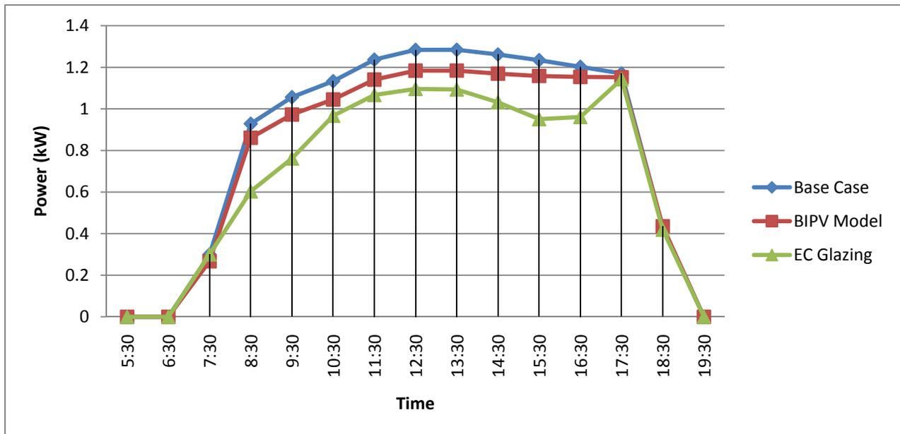
Figure A.19 Hourly Energy Consumption for all configurations for North façade in December 23 with glass of 0.27 shading coefficient and lighting sensor @ 2m
