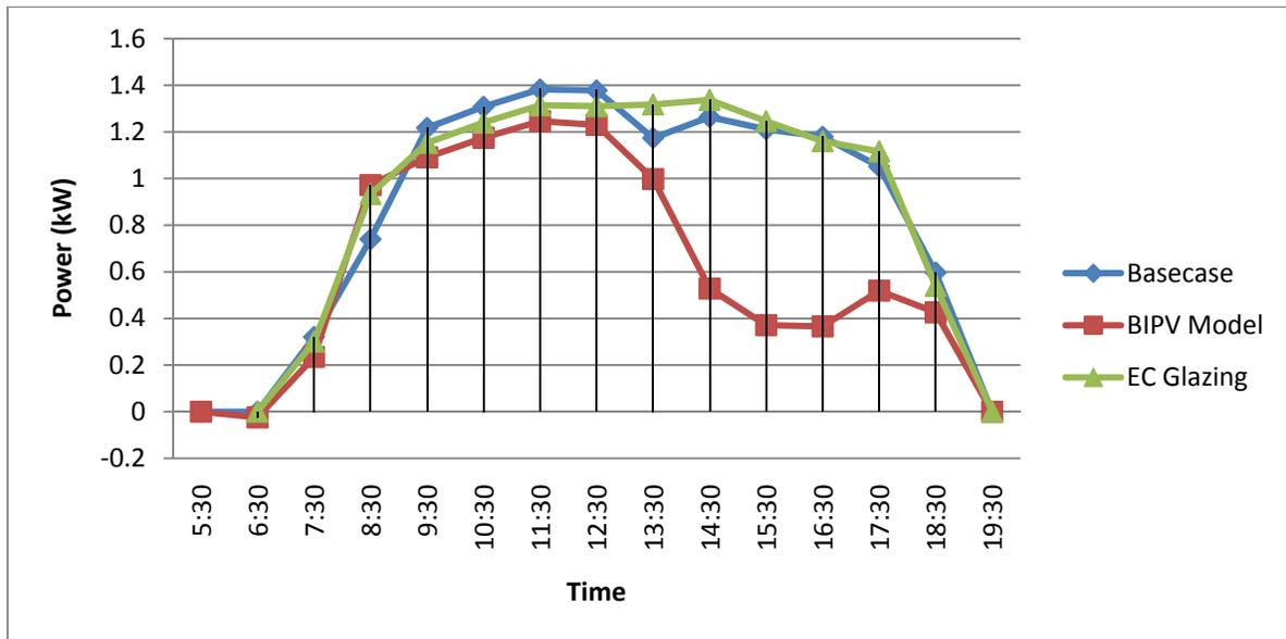
Figure A.12 Hourly Energy Consumption for all configurations for West façade in March 21 with glass of 0.27 shading coefficient and lighting sensor @ 2m
