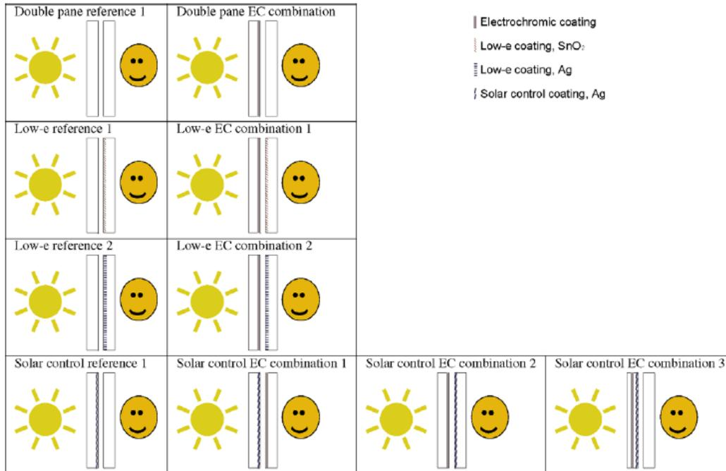
Figure 3.4 Window configurations used in the investigation (Jonsson and Roos, 2009)
