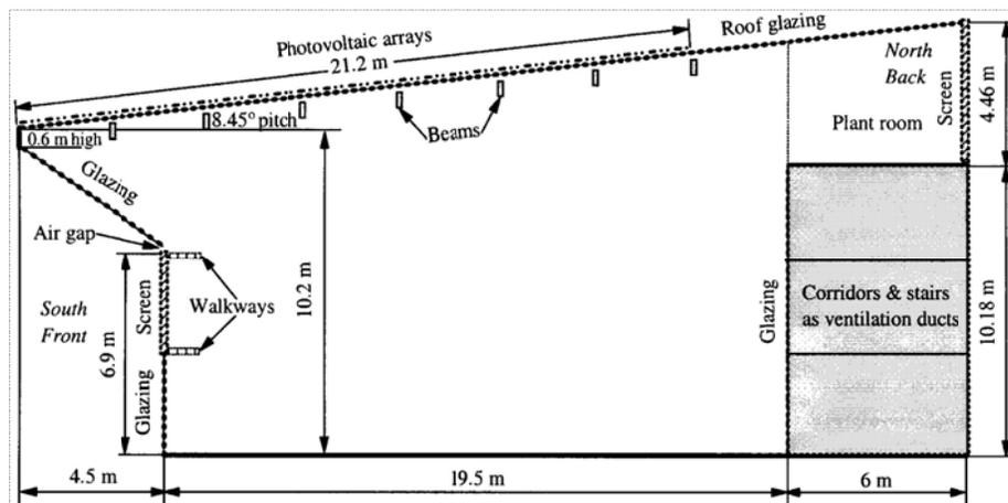
Figure 2.40 Schematic diagram of the atrium (Gan and Riffat, 2001)
