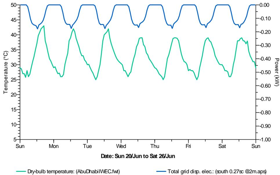
Figure 5.40 Effect of temperature on power output of PV for one week in June for South façade
