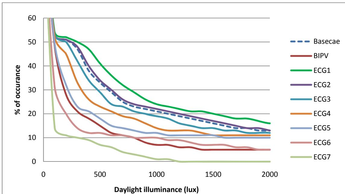
Figure 5.32 Yearly cumulative daylight illuminance distributions for East façade with light sensor @2m
