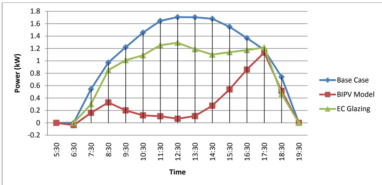
Figure A.3 Hourly Energy Consumption for all configurations for South façade in December 23 with glass of 0.6 shading coefficient and lighting sensor @ 2m
