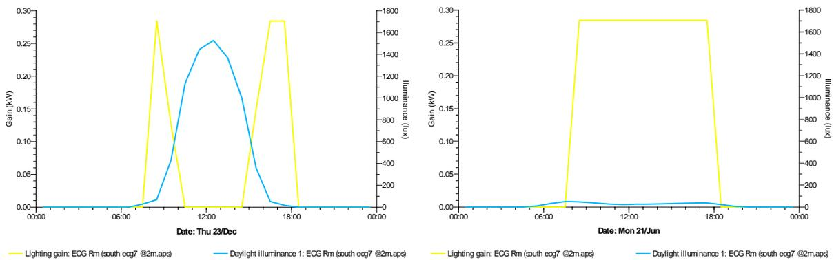
Figure 5.17 EC glazing model lighting gain and daylight illuminance for December 23 (left) and June 21 (right)
