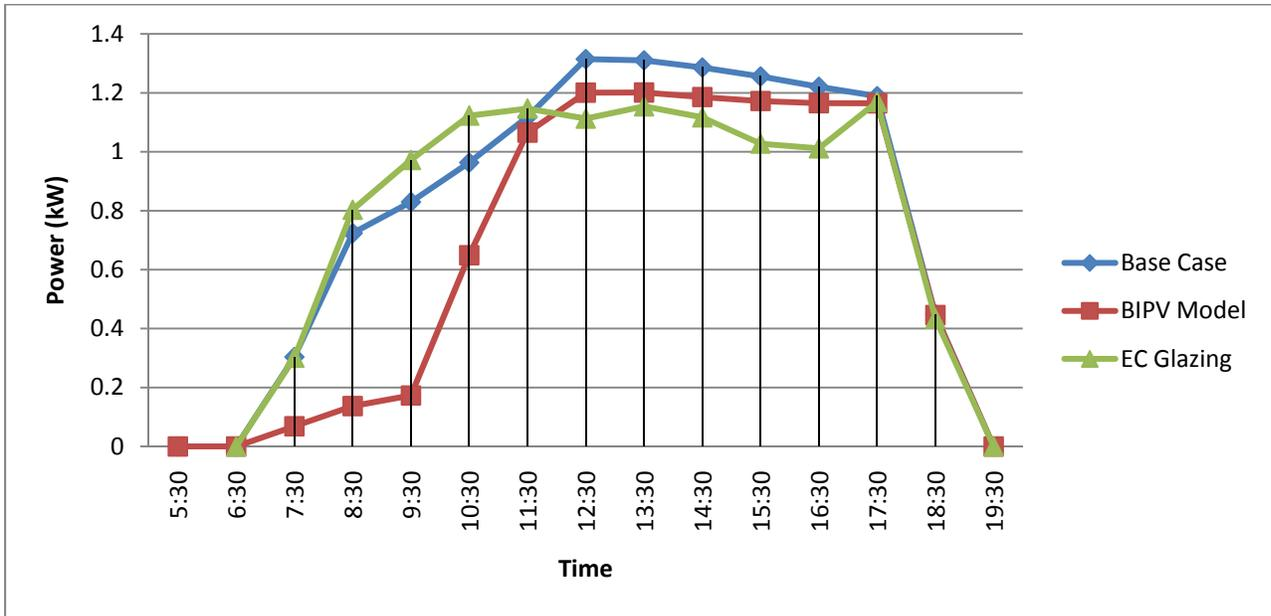
Figure A.11 Hourly Energy Consumption for all configurations for East façade in December 23 with glass of 0.27 shading coefficient and lighting sensor @ 2m
