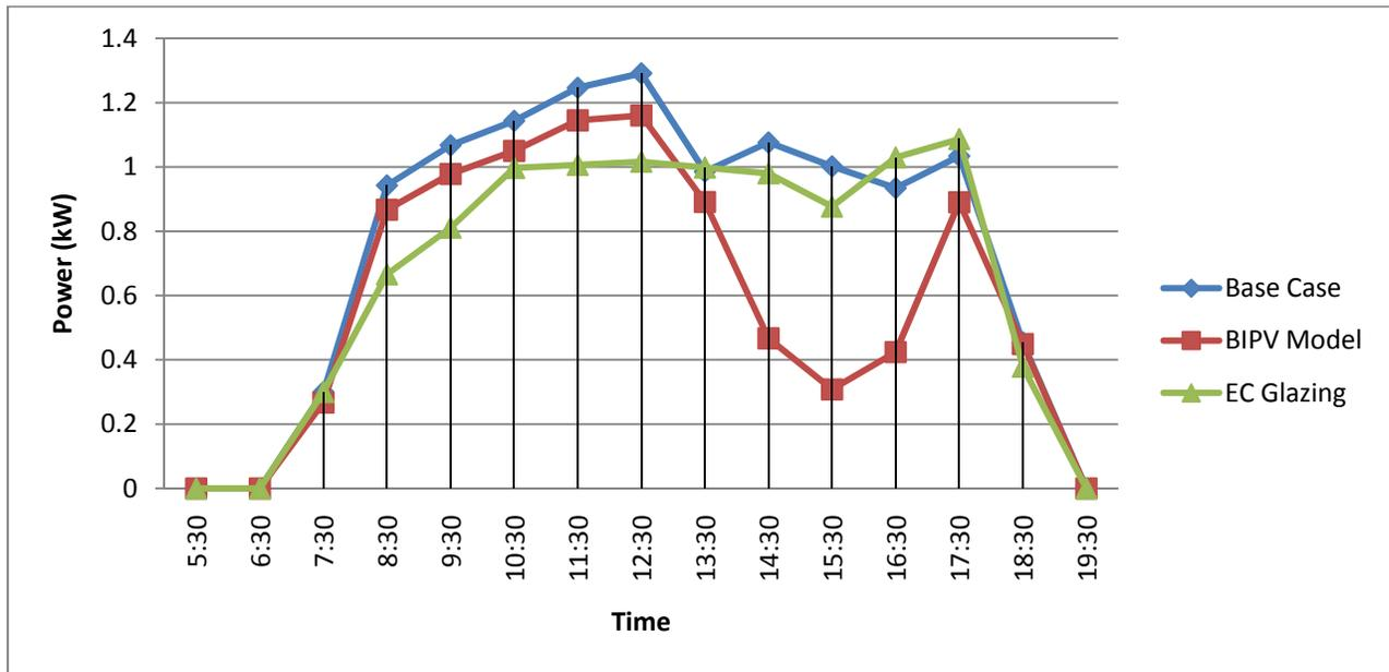
Figure A.15 Hourly Energy Consumption for all configurations for West façade in December 23 with glass of 0.27 shading coefficient and lighting sensor @ 2m
