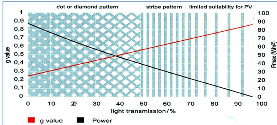
Figure 2.12 Semi-transparent modules: g value and power as a function of light transmission (RHC, 2008)
