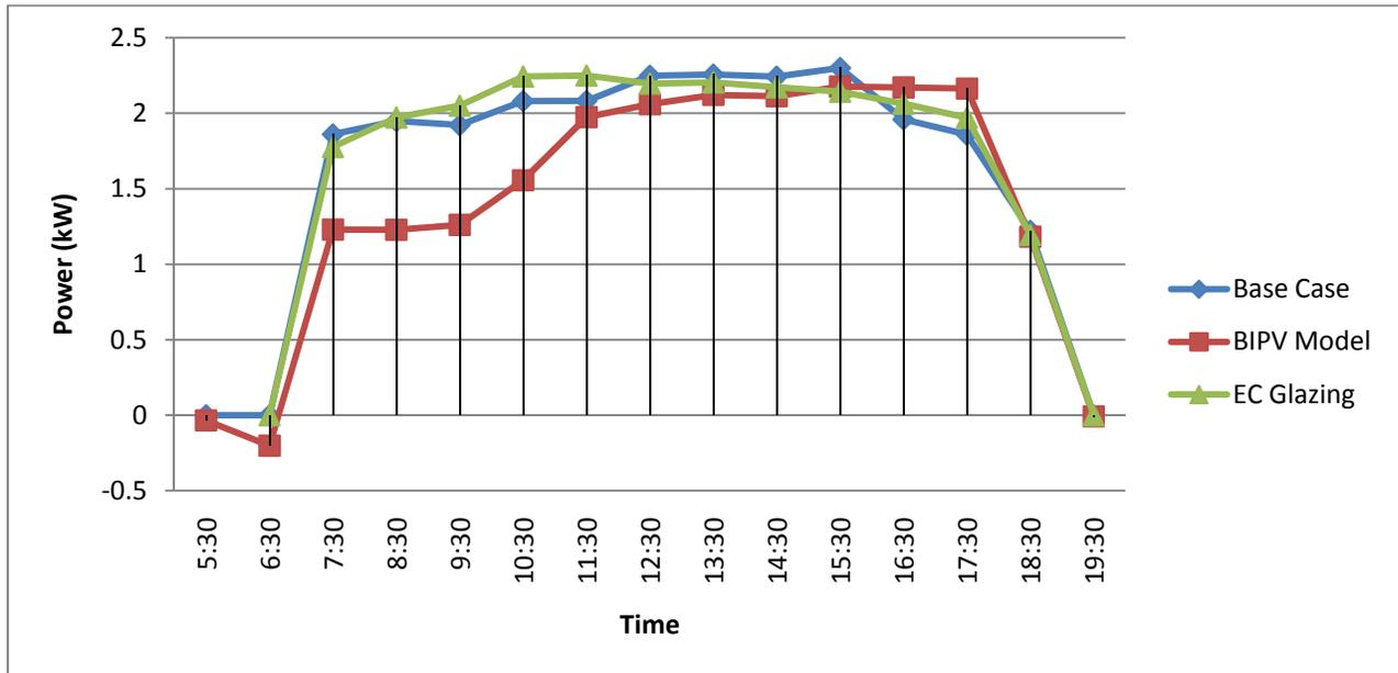
Figure A.9 Hourly Energy Consumption for all configurations for East façade in June 21 with glass of 0.27 shading coefficient and lighting sensor @ 2m
