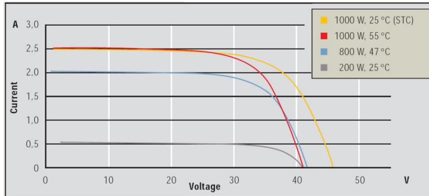
Figure 2.20 Intensity and temperature-dependent behavior (Wurth Solar, 2010)
