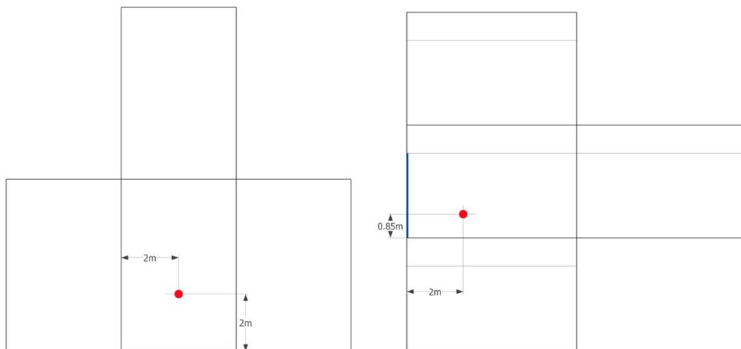
Figure 4.4 Plan (left) and side elevation (right) of lighting sensor at 2m from window
