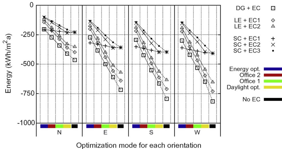
Figure 2.37 Cooling energy balance of studied window combinations for four orientations in Miami (Jonsson and Roos, 2009)
