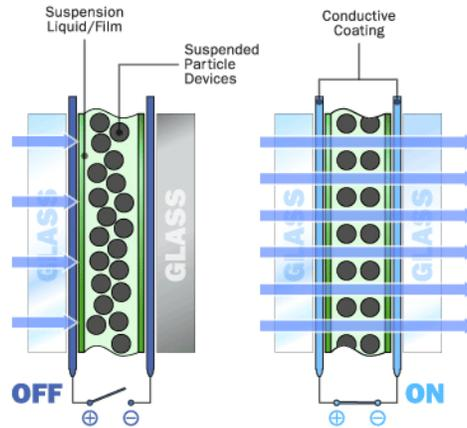
Figure 2.24 SPD Smart Windows working mechanism (Bonsor, 2010)
