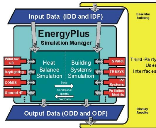
Figure 3.7 Overall EnergyPlus program structure (Crawley et al., 2000)
