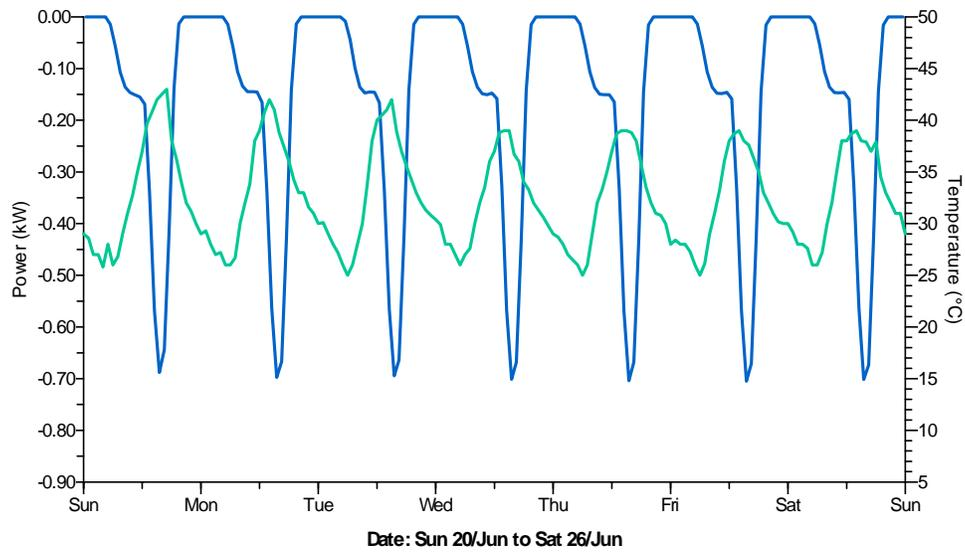
Figure 5.42 Effect of temperature on power output of PV for one week in June for West façade
