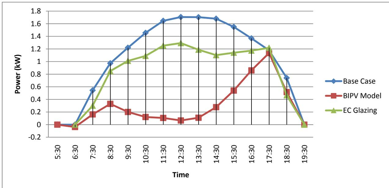
Figure A.2 Hourly Energy Consumption for all configurations for South façade in September 21 with glass of 0.6 shading coefficient and lighting sensor @ 2m
