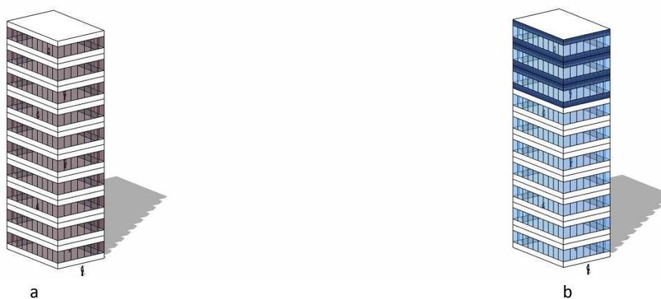
Figure 3.6 EC glazing utilized over all the floors (a); BIPV cells only on the top three levels (b)
