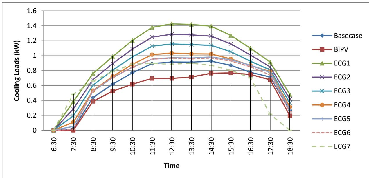
Figure 5.8 Total Cooling Loads for all configurations for South façade in March 21
