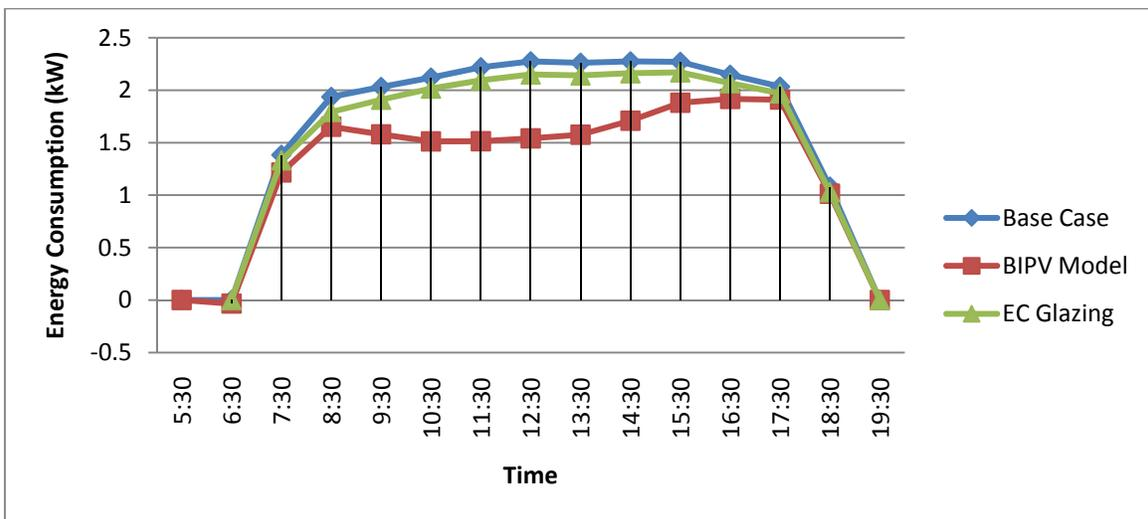
Figure 5.24 Hourly Energy Consumption for all configurations for South façade in September 21 with glass of 0.27 shading coefficient and lighting sensor @ 4m
