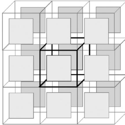
Figure 2.36 A 3 x 3 array of thermally linked rooms, with highlighted central room being used for air conditioning requirement analysis (Bahaj et al., 2008)
