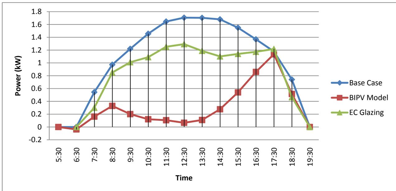
Figure A.5 Hourly Energy Consumption for all configurations for South façade in June 21 with glass of 0.27 shading coefficient and lighting sensor @ 4m
