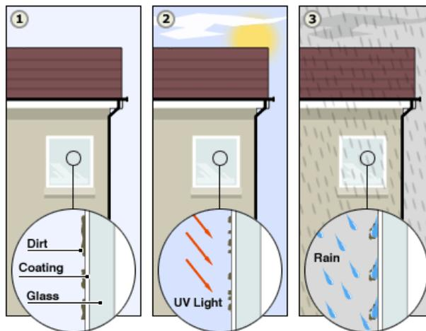
Figure 2.5 Photo-catalytic process in self-cleaning glass (Twist, 2009)
