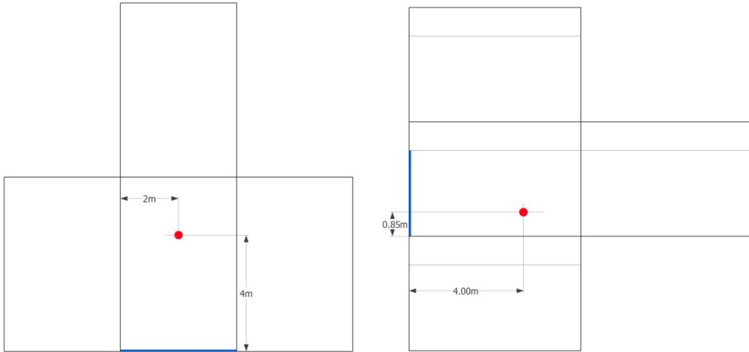
Figure 4.5 Plan (left) and side elevation (right) of lighting sensor at 4m from window
