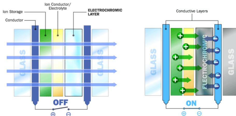
Figure 2.25 Layers of EC glazing and the working mechanism (Bonsor, 2010)
