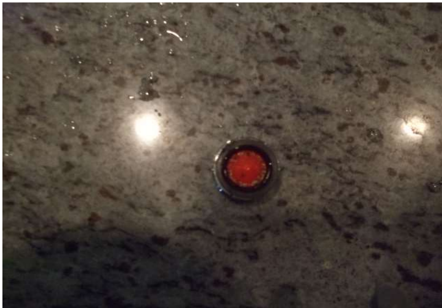
Figure A.4 Sediments accumulation on the faucet aerator
