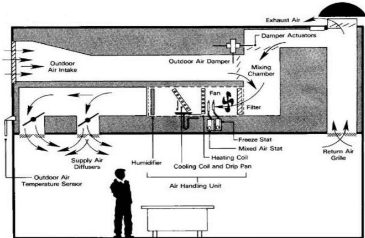
**Figure 2.1 : Typical layout of HVAC system components**
