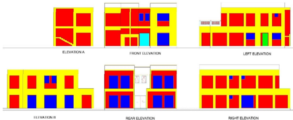
Figure 4.5: Elevations concrete to wall ratio
