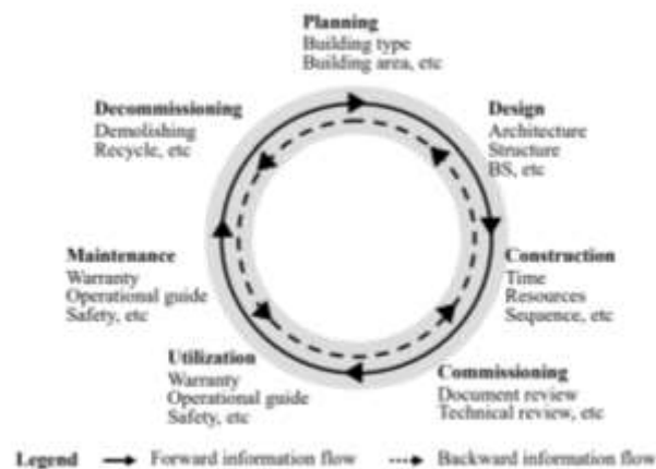
Figure 12: Information flow chart for construction projects
