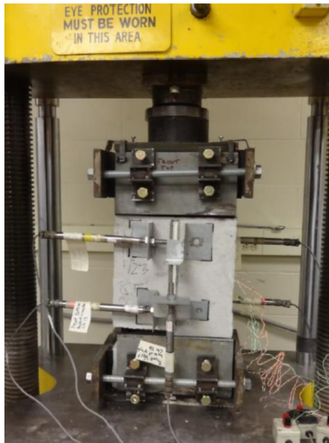
Fig. 2.7 – Push-off Test Setup
