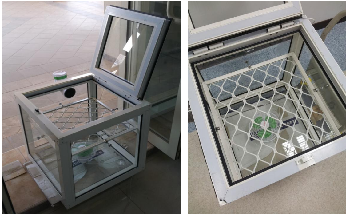
Figure 1 'the chamber' during and after venting between each wood sample assessment
