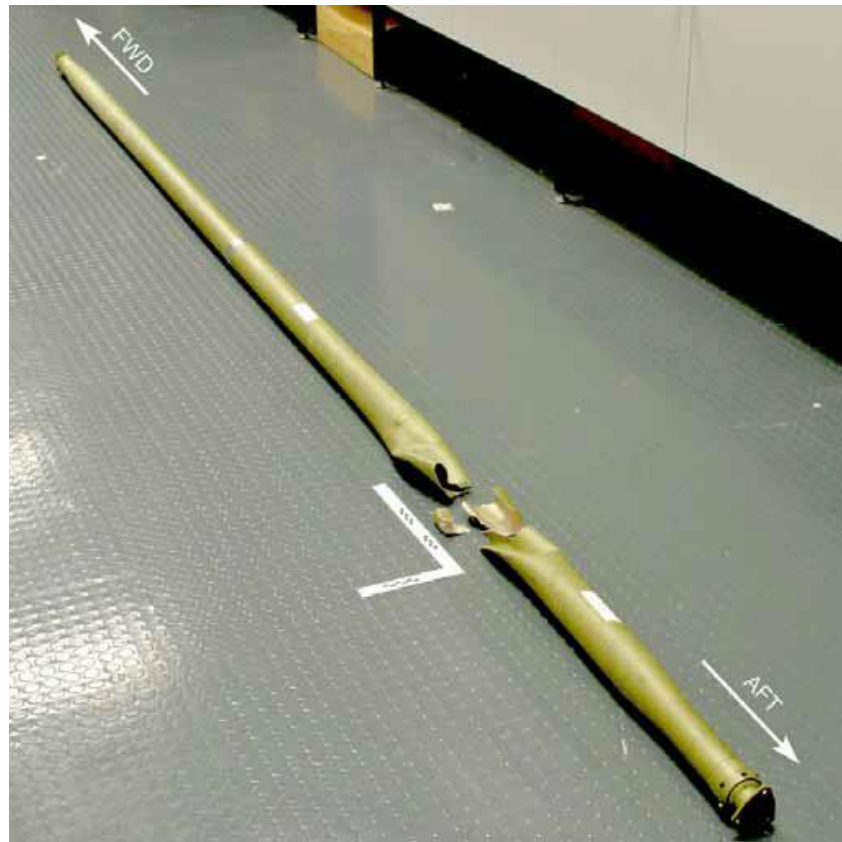
Figure 4 Damaged Tail Rotor Shaft Optical Examination (Source: “ATSB”2005)
