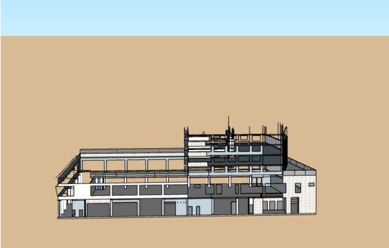
Figure 37; Construction of the pillars, floor slabs, and wall cladding.
