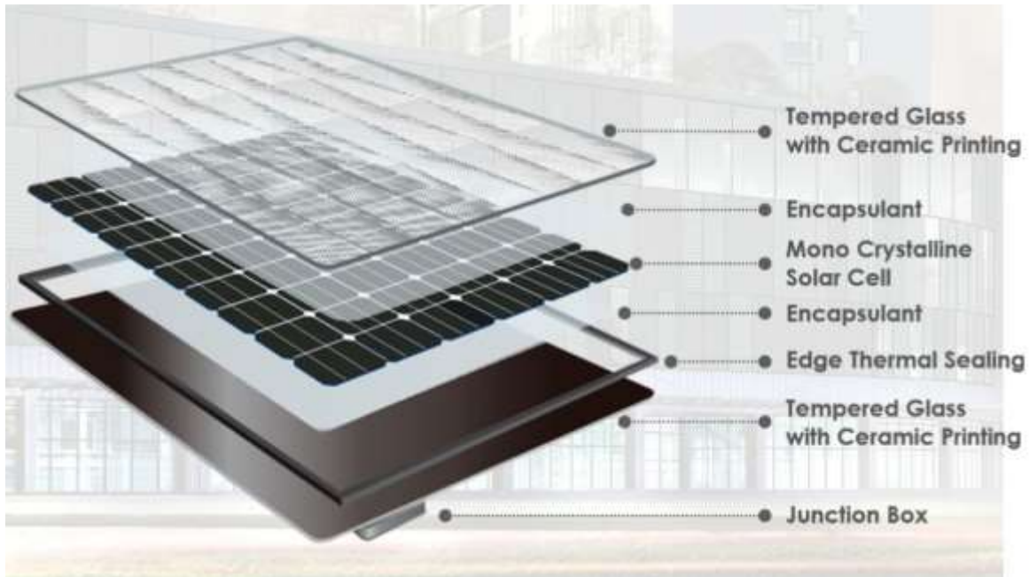
Figure 22; Components of an Aesthetic Energy Panels
