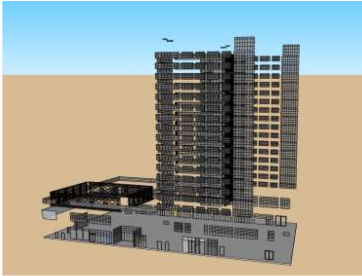
Figure 38; Replacing existing wall material with ACP. This involves changing building properties in the IESVE extension on Stech-up. As well as the allocation of different settings and characteristics like thermal performance.
