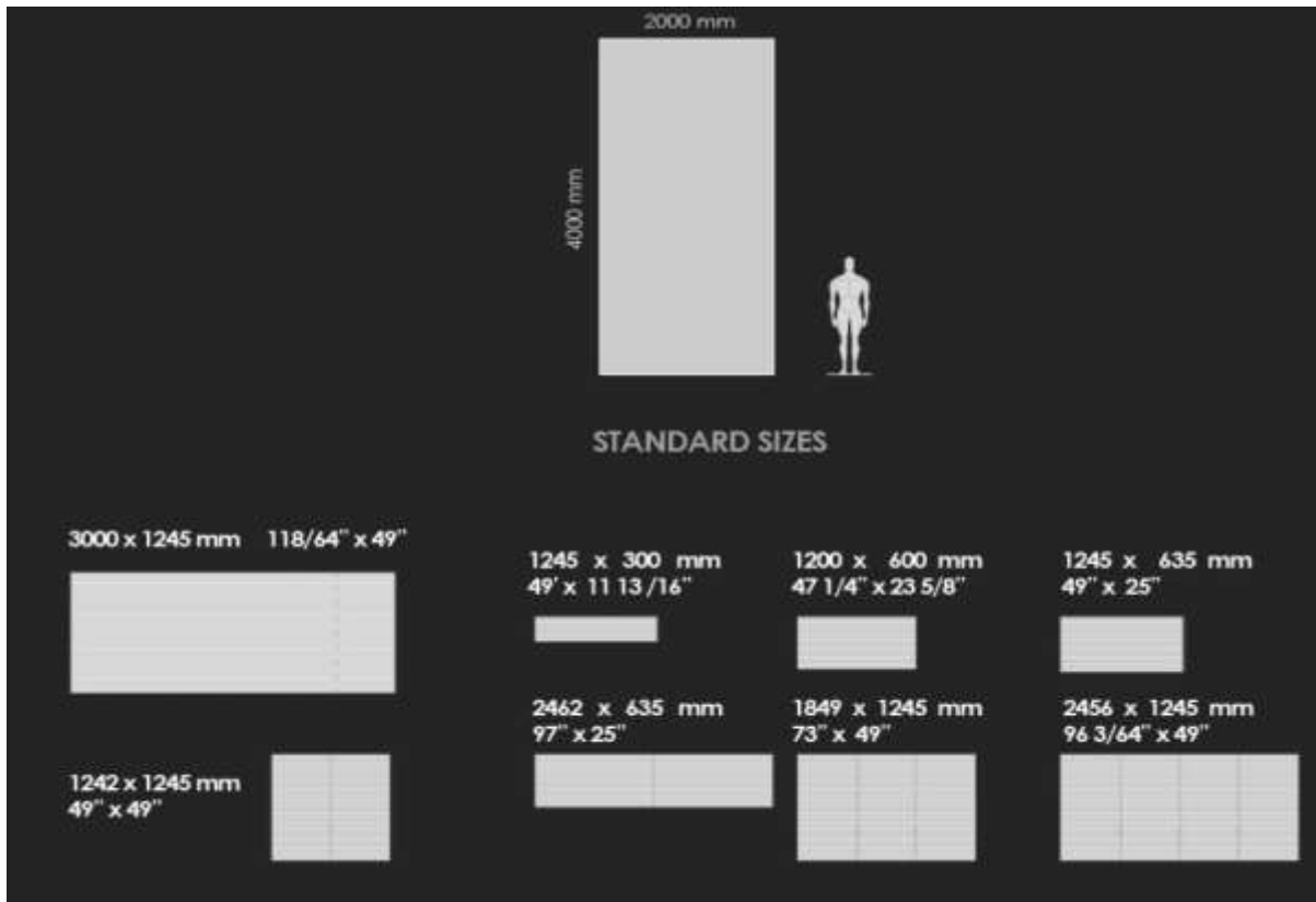
Figure 21; Standard sizes available in the market for Amorphous Photovoltaic Panels
