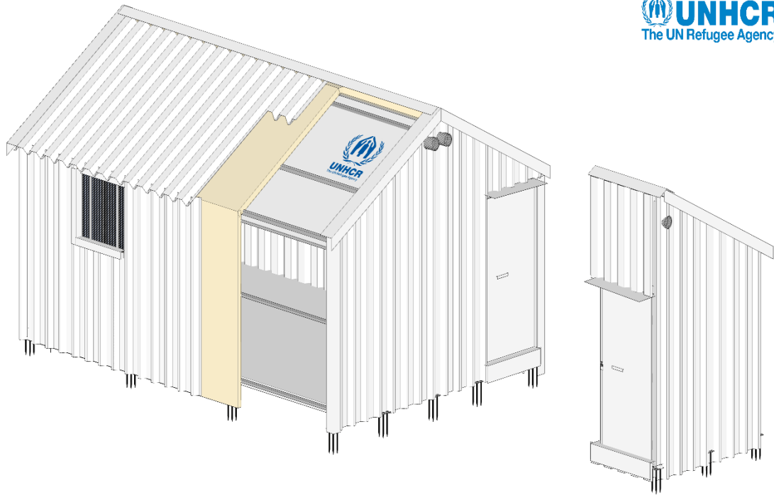
Figure 20: Diagram of the T-Shelter showing its layers and the possibility of adding a side entrance for privacy
