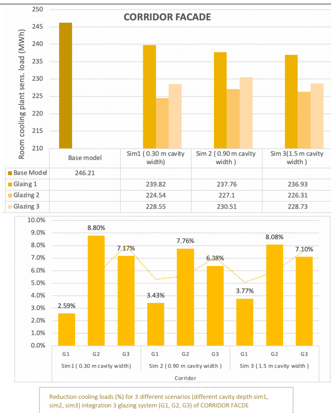
Fig. 71 Comparing the total annual cooling consumption MWh and the saving cooling reduction (%) between the 4 DSF types of the 1 st -strategy and comparison with the reference base case
