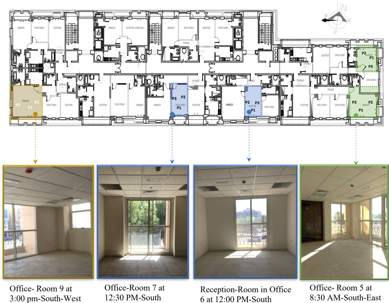
Fig. 51 The selected day-light measuring rooms in the 1 st floor of actual building and the (P1,P2,P3) indicate to the point positions of lighting measurements by EXTECT lux tool during field site. Source:(author)
