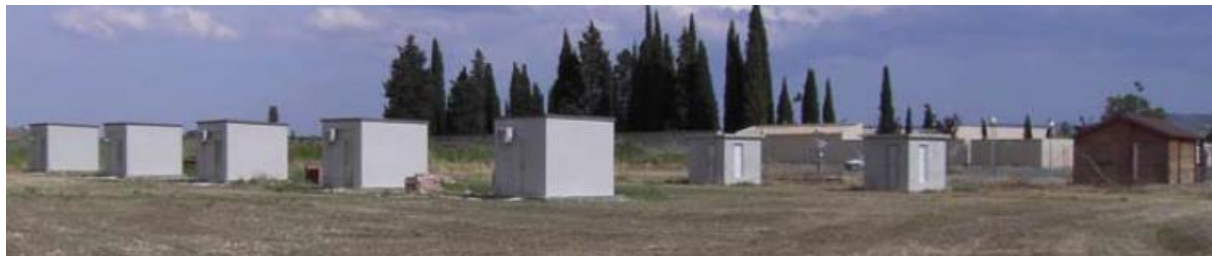
Figure 3.5: Photograph of cubicles built as typical Mediterranean building strategies tested different insulation materials (Source: Castell et al (2014))
