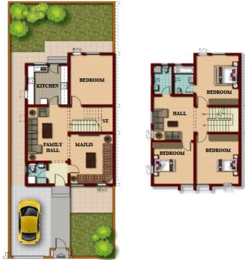
Figure 2.31: Housing unit T3M plan, Ground floor (left), First floor (right), (Source: Ministry of Housing, 2012).
