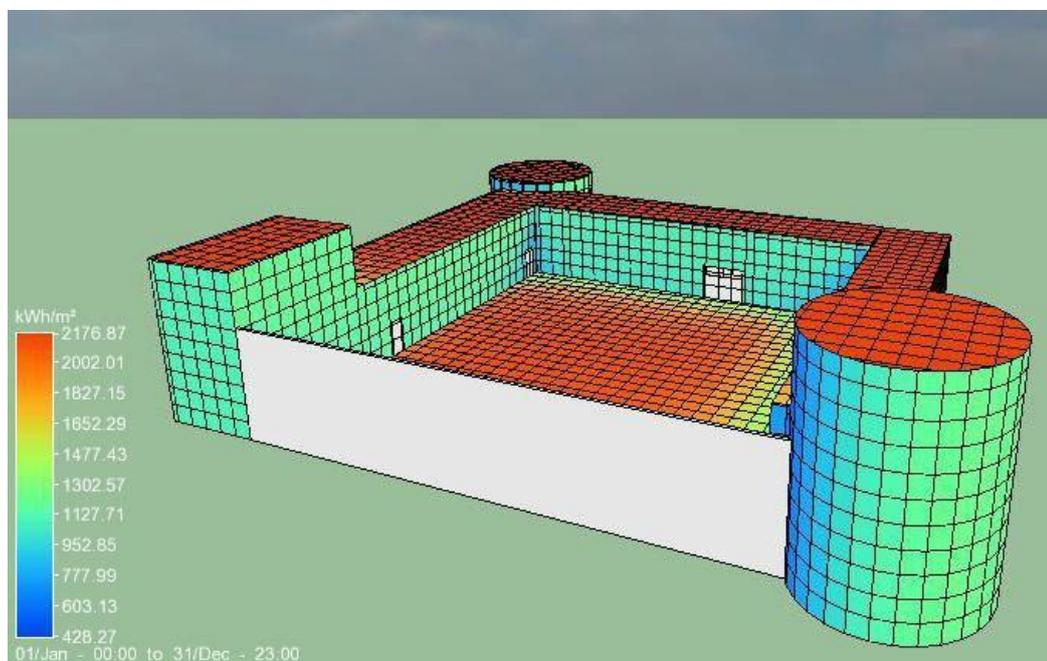
Figure 4.16 Base Simulation Model (IES-VE)
