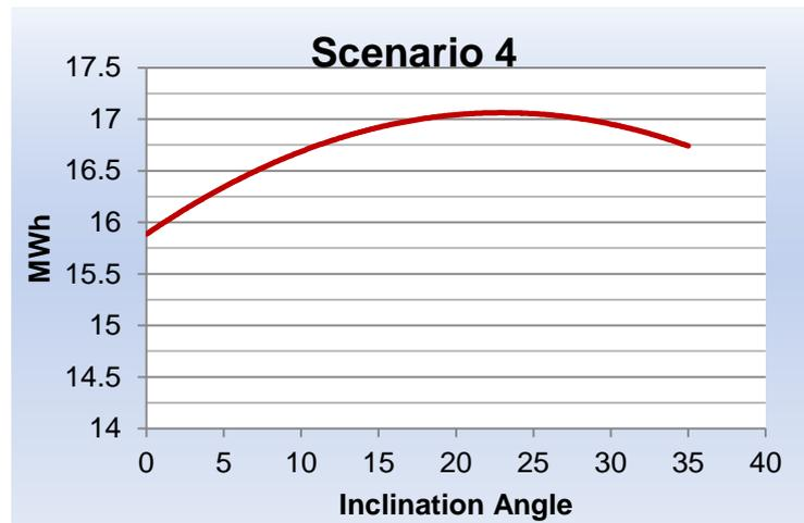
Figure 5.7 PV power production at various inclination angles (IES-VE)
