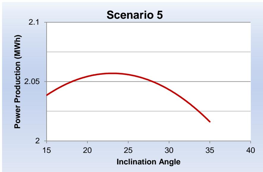
Figure 5.8 PV power production at various inclination angles (IES-VE)
