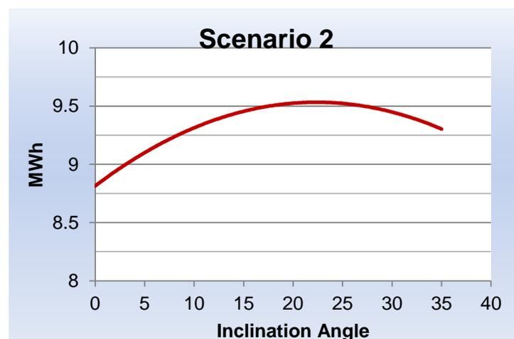
Figure 5.4 PV power production at various inclination angles (IES-VE)
