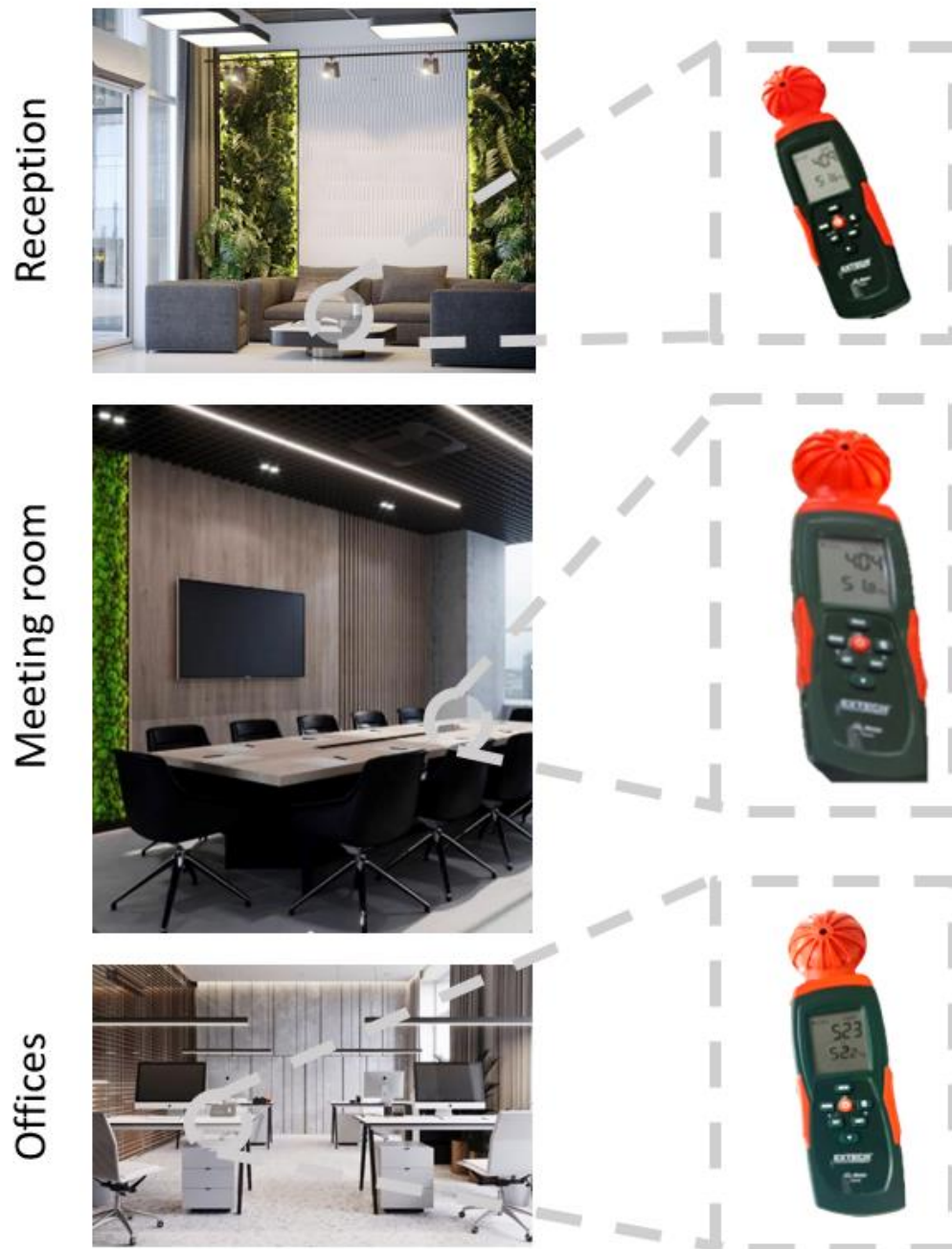
Figure 48: High-cost company 03 indoor environment CO2 meter results. (Source: Khaloud, 2023)
