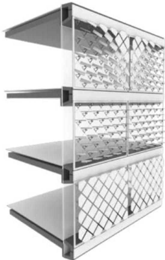
**Figure 2.28. Modular dynamic façade which allows different positioning for the shades/screen for various purposes (Nagy et al. 2016).**
