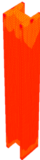
Fig. (4.8) Stresses of the Encased Column under Axial Compression Load
