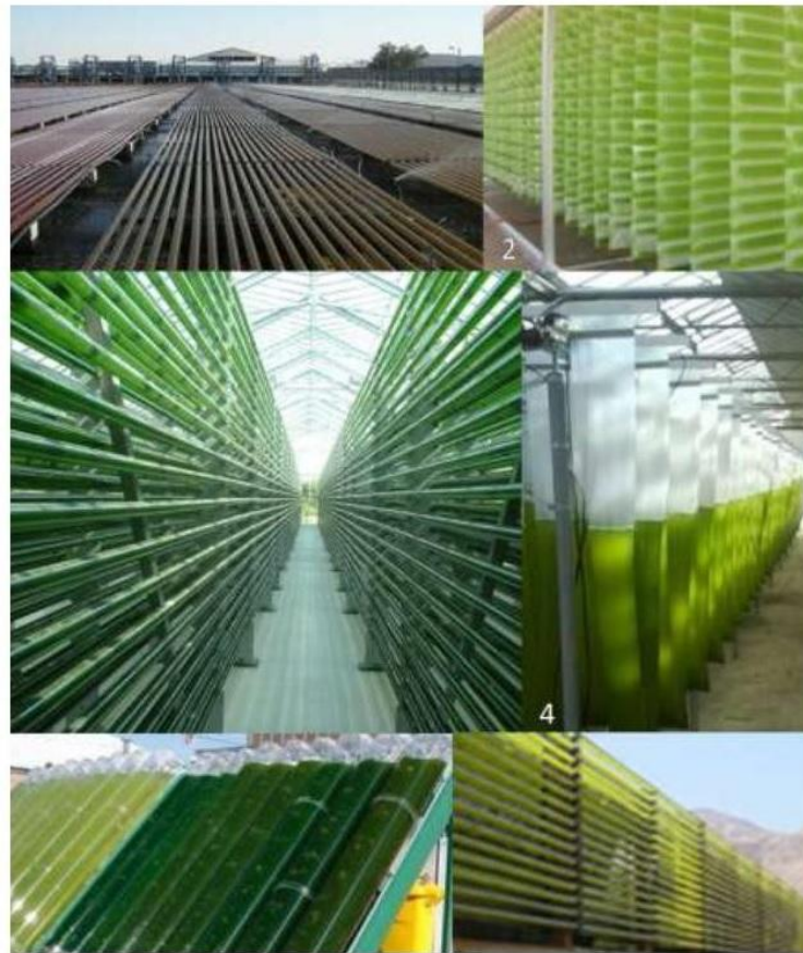
Figure 2.2: Microalgae cultivation in photobioreactors. Source: (CBDMT- Market and Business Intelligence, 2011)
