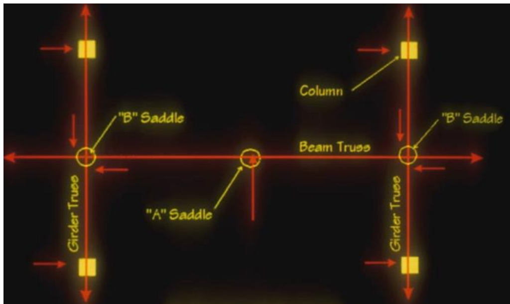
FIGURE 4.6: Schematic of Load application of orthogonal trusses (ACI-318, CEU)
