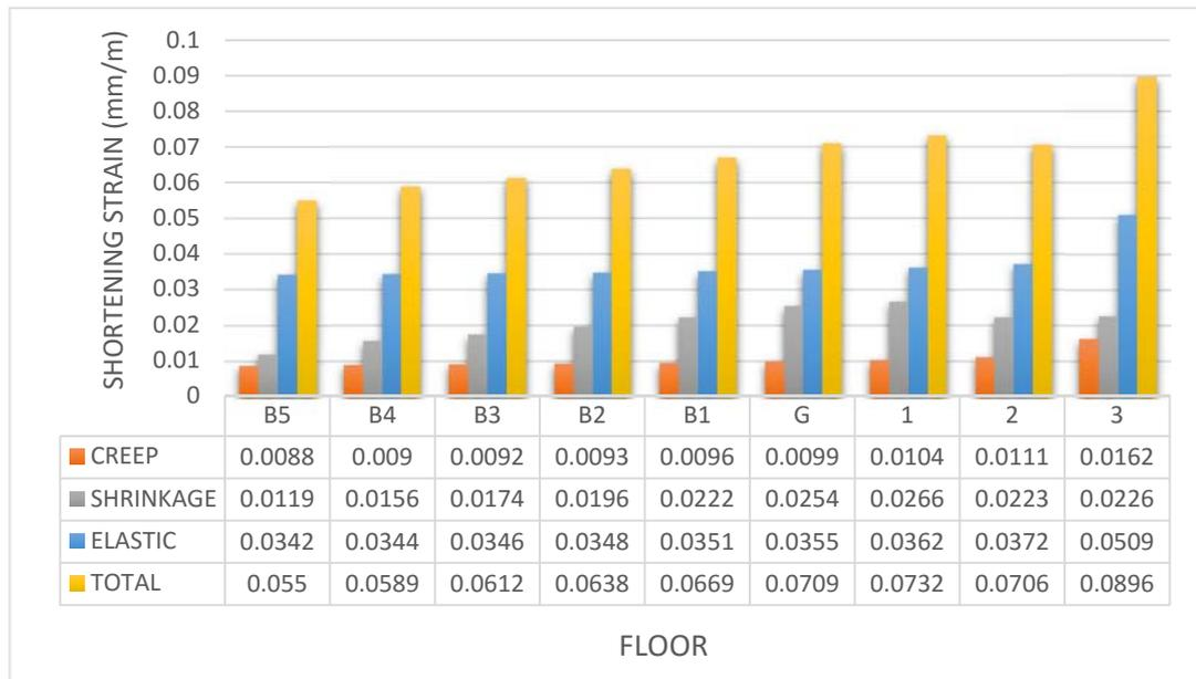
Fig.11 Strain of monitored **walls** below 4<sup>th</sup> floor due to adding floors 4<sup>th</sup> to 8<sup>th</sup>
