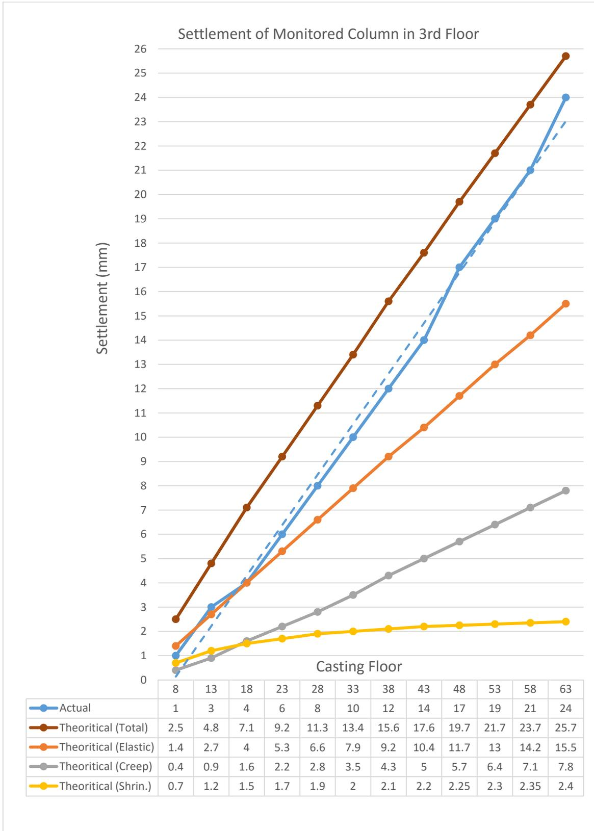
Fig.12 Actual & Theoretical Settlement of Monitored Column in 3<sup>rd</sup> Floor
