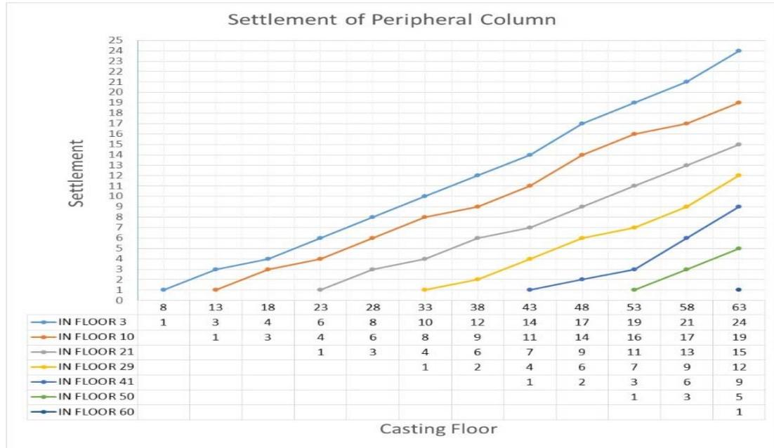
Fig.6 Site readings of peripheral column settlement
