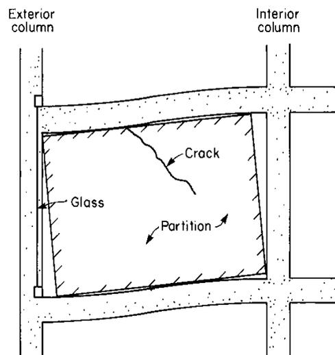
*Fig.22 Effects of tilted slab*
