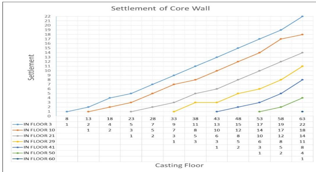
Fig.7 Site readings of core wall settlement
