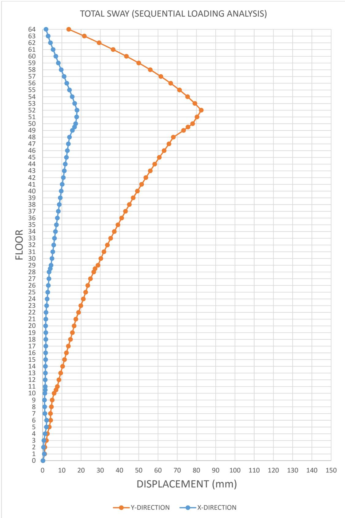
Fig.27 Total lateral sway of all floors (sequential loading analysis)
