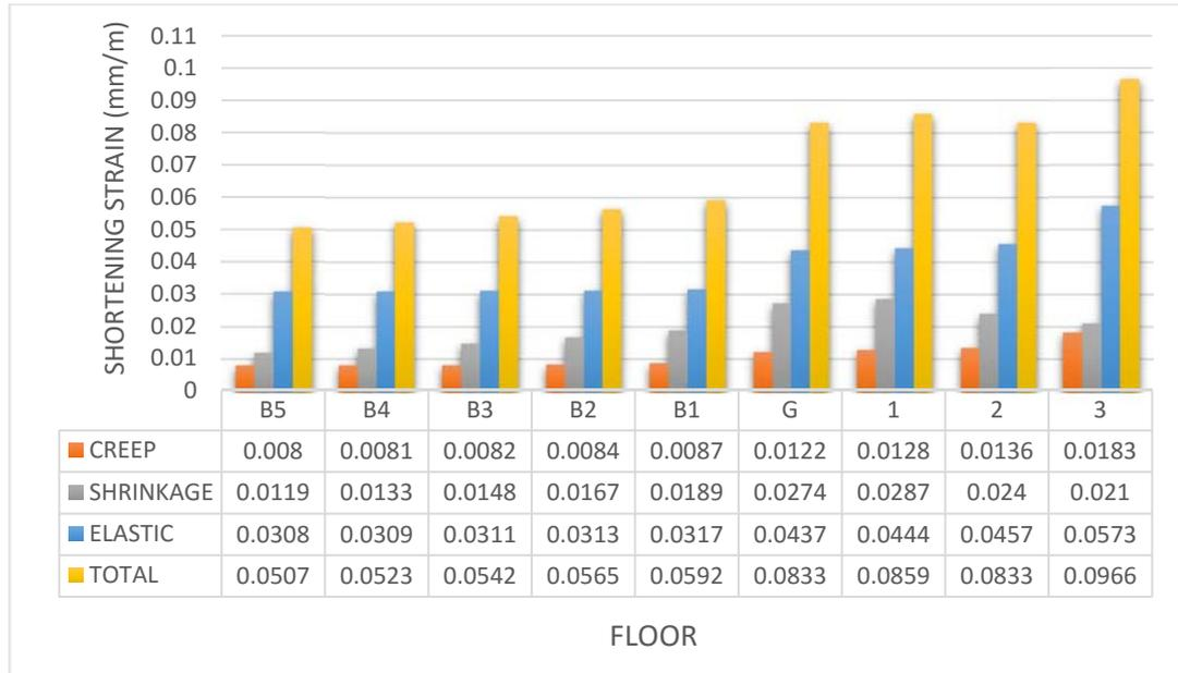
Fig.10 Strain of monitored **columns** below 4<sup>th</sup> floor due to adding floors 4<sup>th</sup> to 8<sup>th</sup>
