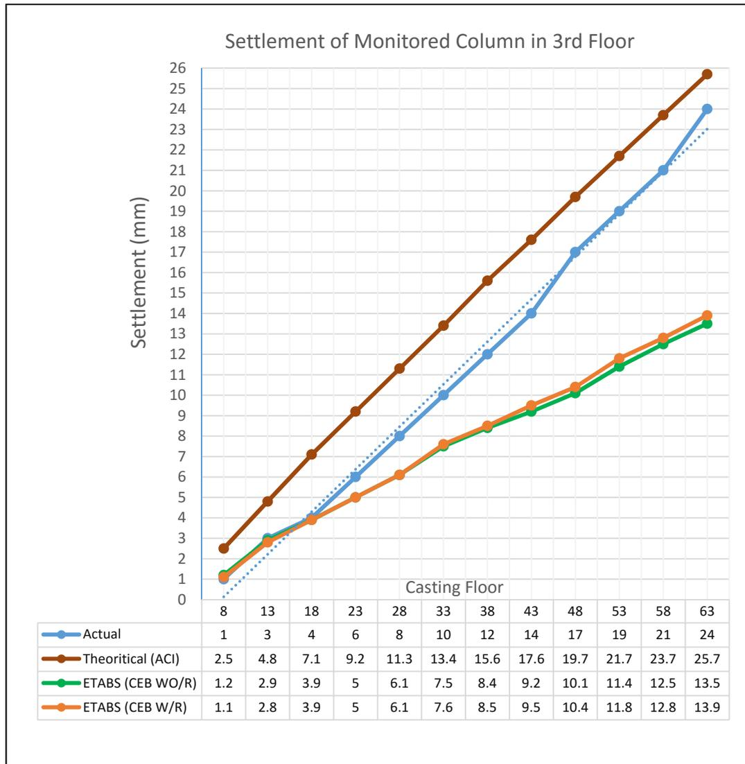
Fig.14 Actual, Theoretical and ETABS Settlement of Monitored Column in 3<sup>rd</sup> Floor
