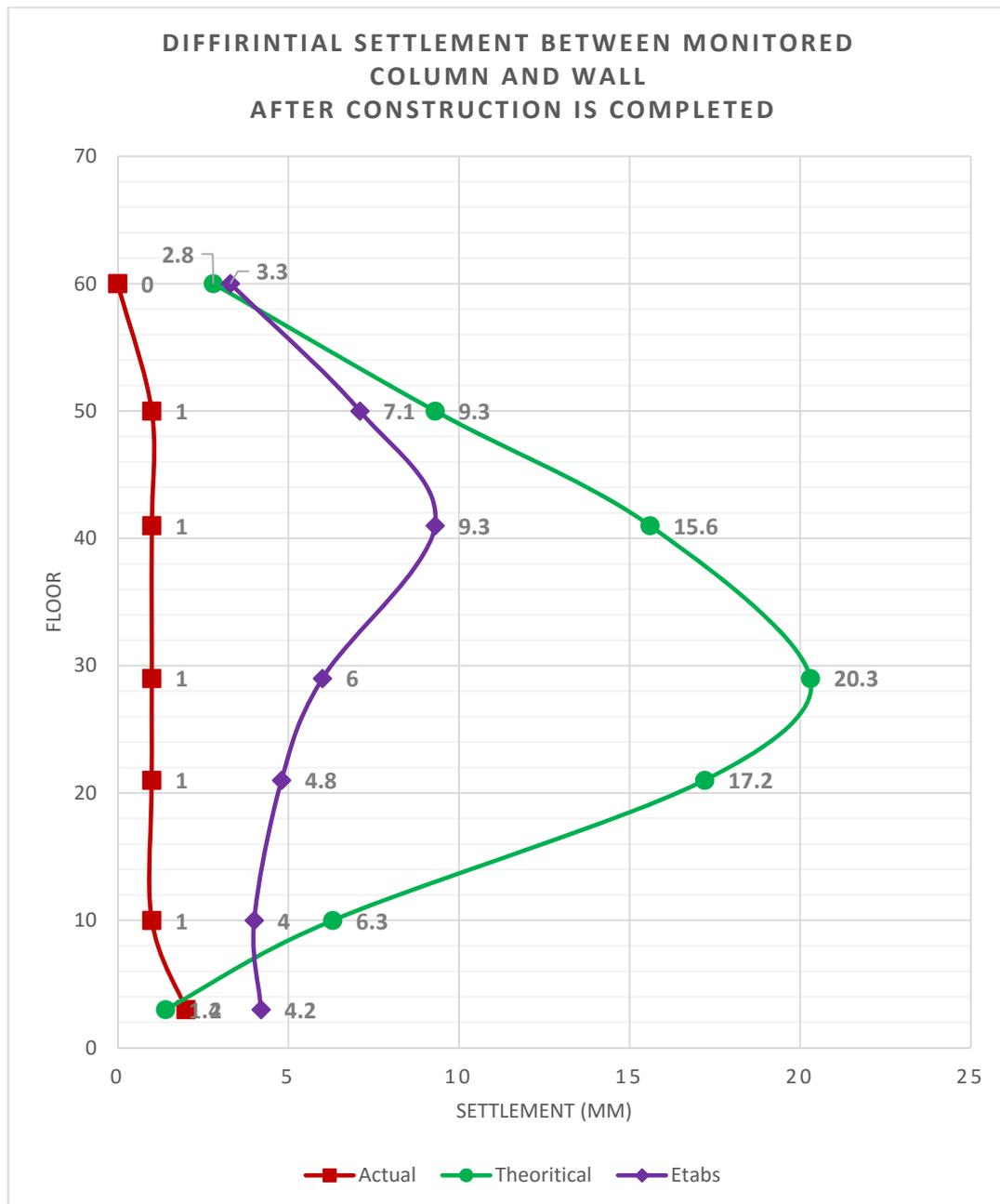
Fig.23 Differential settlement between monitored column and wall
