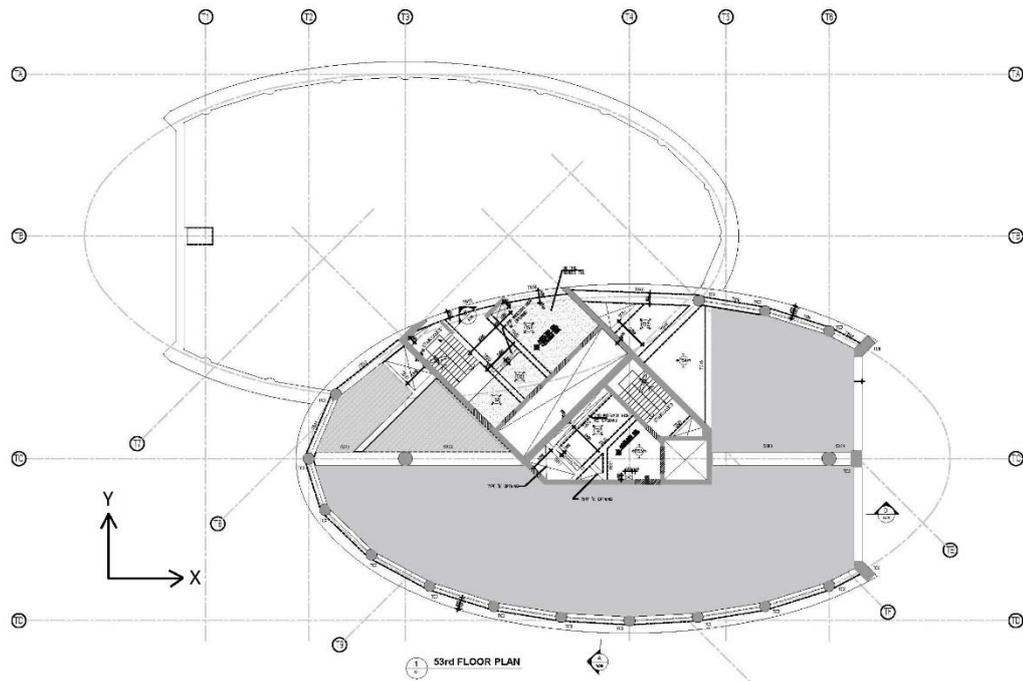
*Fig.24 Typical structural plan of the tower after the 52<sup>nd</sup> floor*
