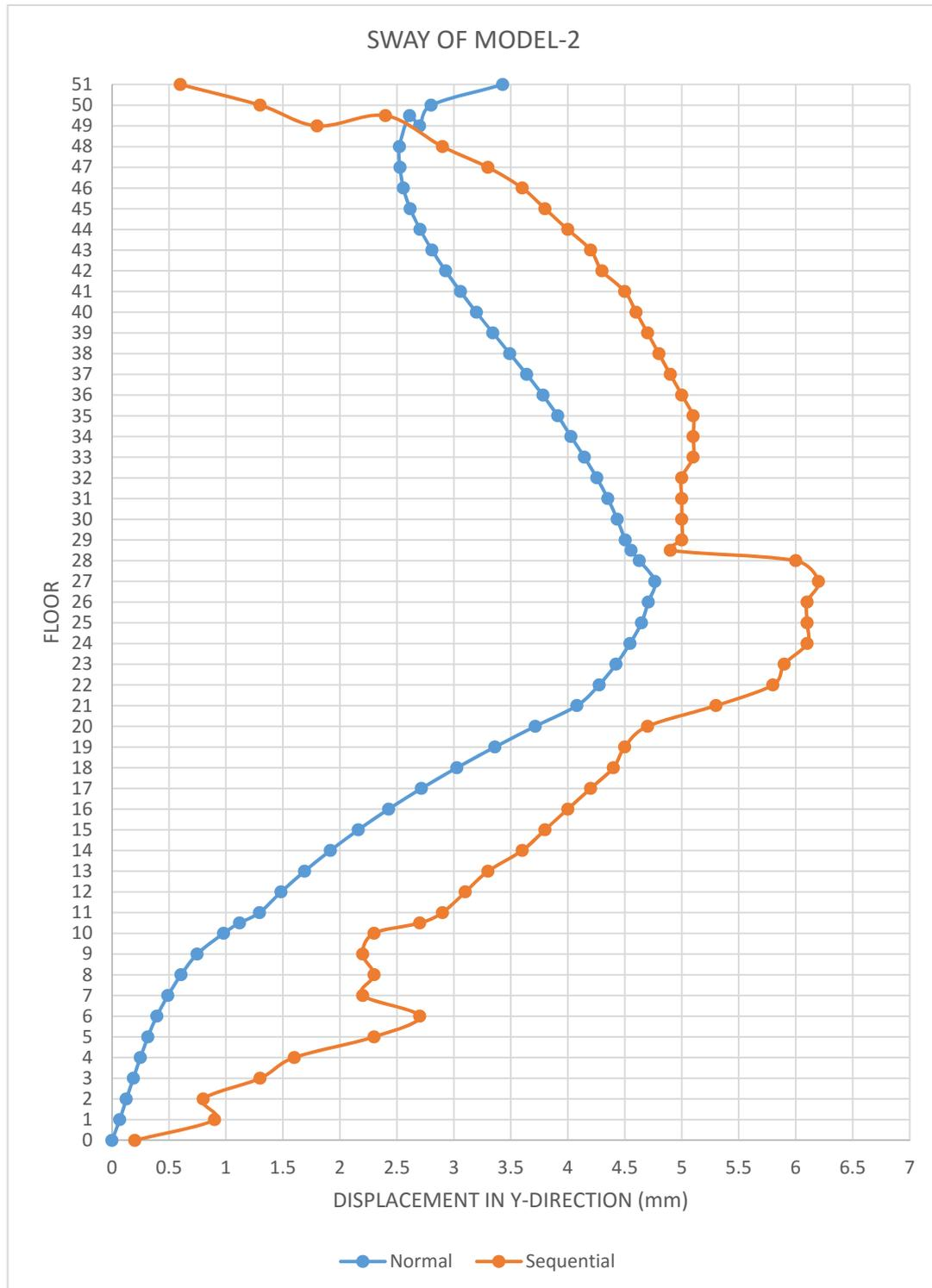
Fig.30 Normal and Sequential sway of model-2
