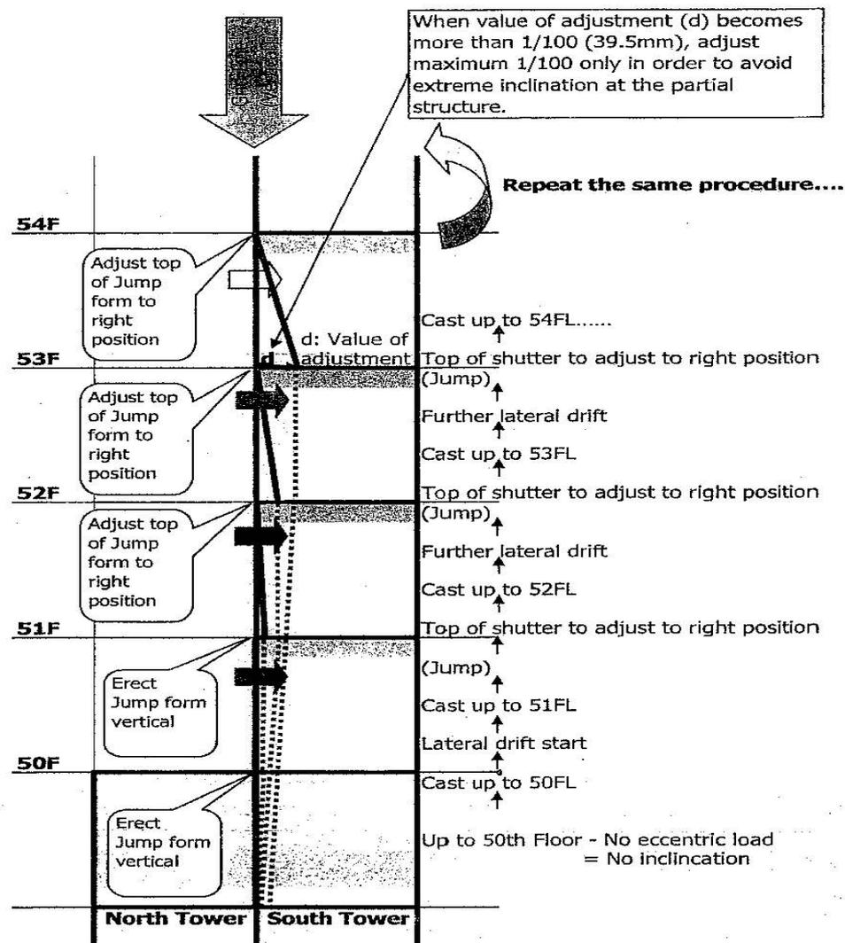
Fig.25 Method of vertical alignment used in the tower construction
