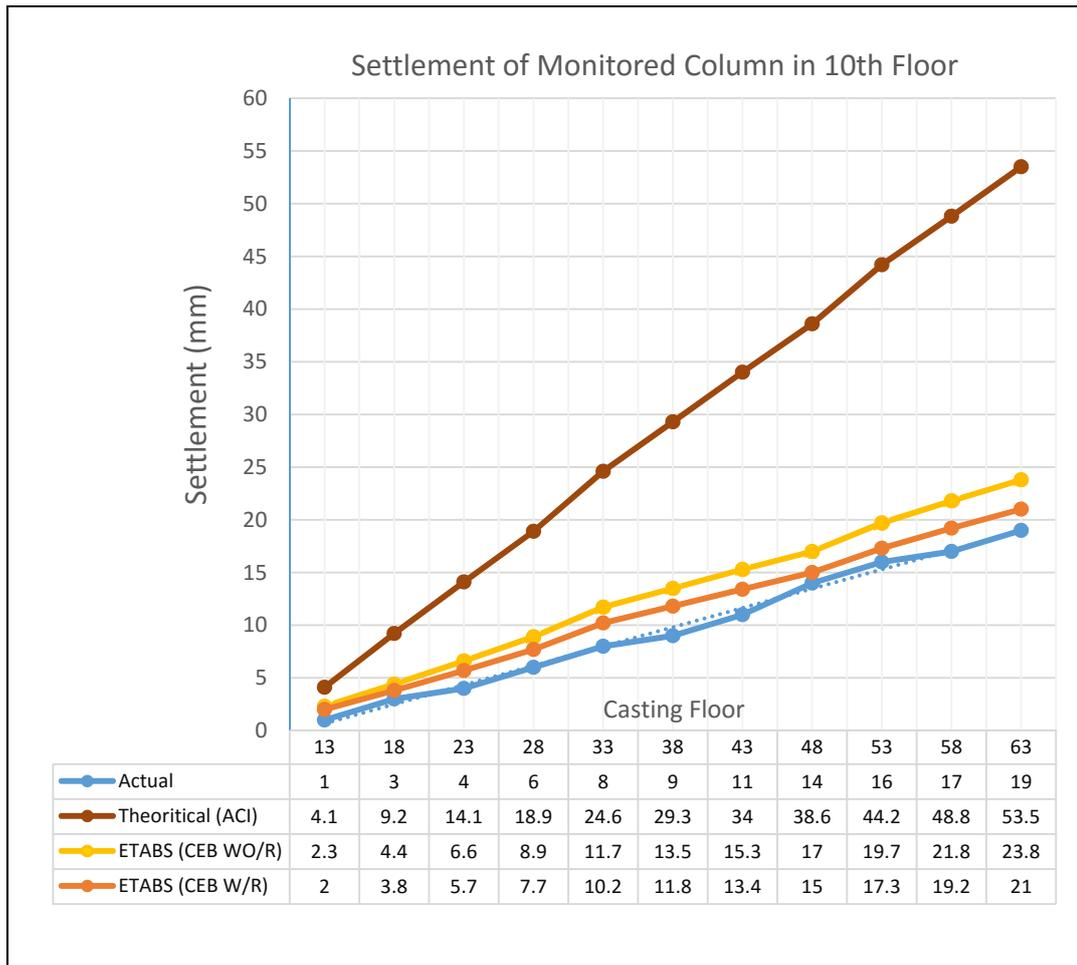
Fig.15 Actual, Theoretical and ETABS Settlement of Monitored Column in 10<sup>th</sup> Floor
