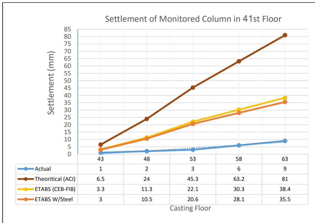
Fig.18 Actual, Theoretical and ETABS Settlement of Monitored Column in 41<sup>st</sup> Floor
