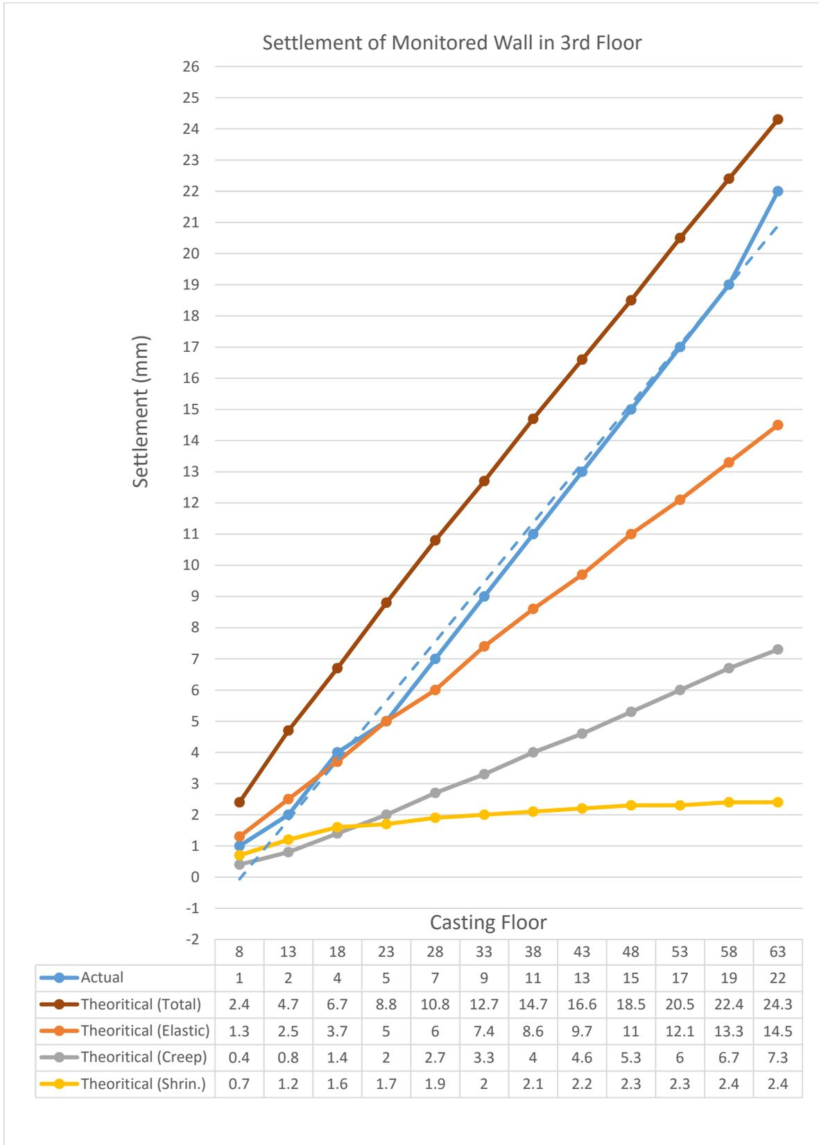
Fig.13 Actual & Theoretical Settlement of Monitored Wall in 3<sup>rd</sup> Floor
