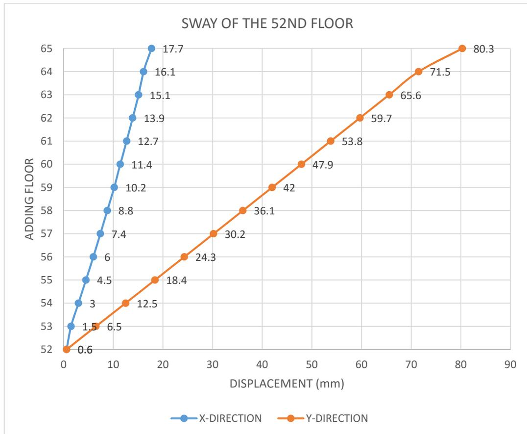
*Fig.29 Sequential sway of the separation floor*
