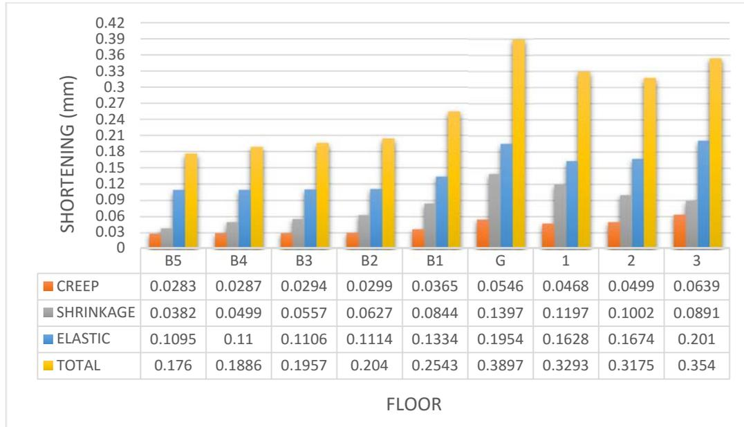
Fig.9 Shortening of monitored walls below 4<sup>th</sup> floor due to adding floors 4<sup>th</sup> to 8<sup>th</sup>
