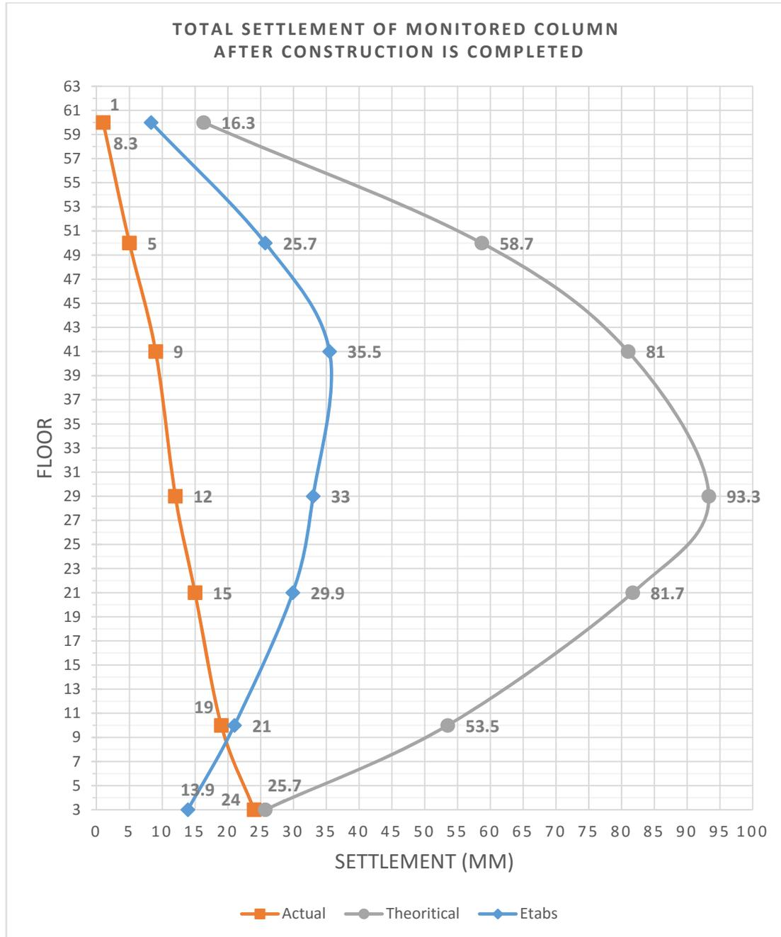
Fig.20 Total settlement of monitored column after completion of construction
