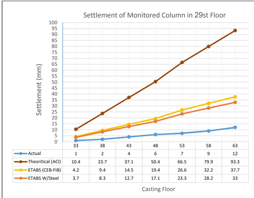
Fig.17 Actual, Theoretical and ETABS Settlement of Monitored Column in 29<sup>th</sup> Floor
