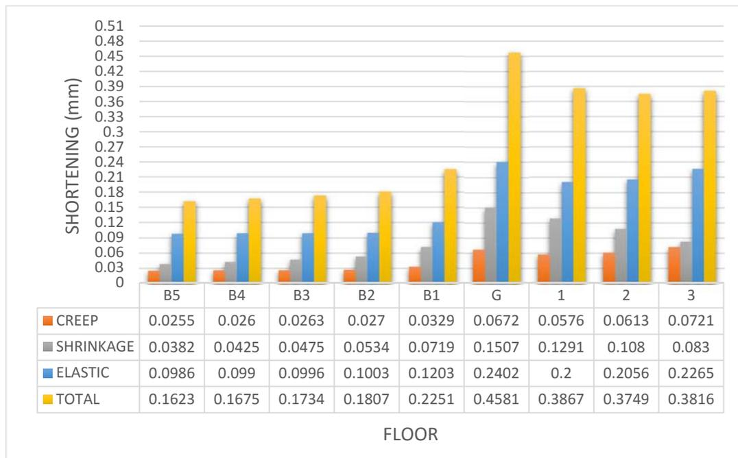
Fig.8 Shortening of monitored *columns* below 4<sup>th</sup> floor due to adding floors 4<sup>th</sup> to 8<sup>th</sup>
