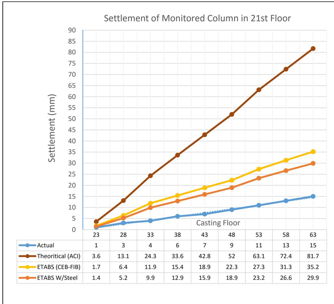
Fig.16 Actual, Theoretical and ETABS Settlement of Monitored Column in 21<sup>st</sup> Floor
