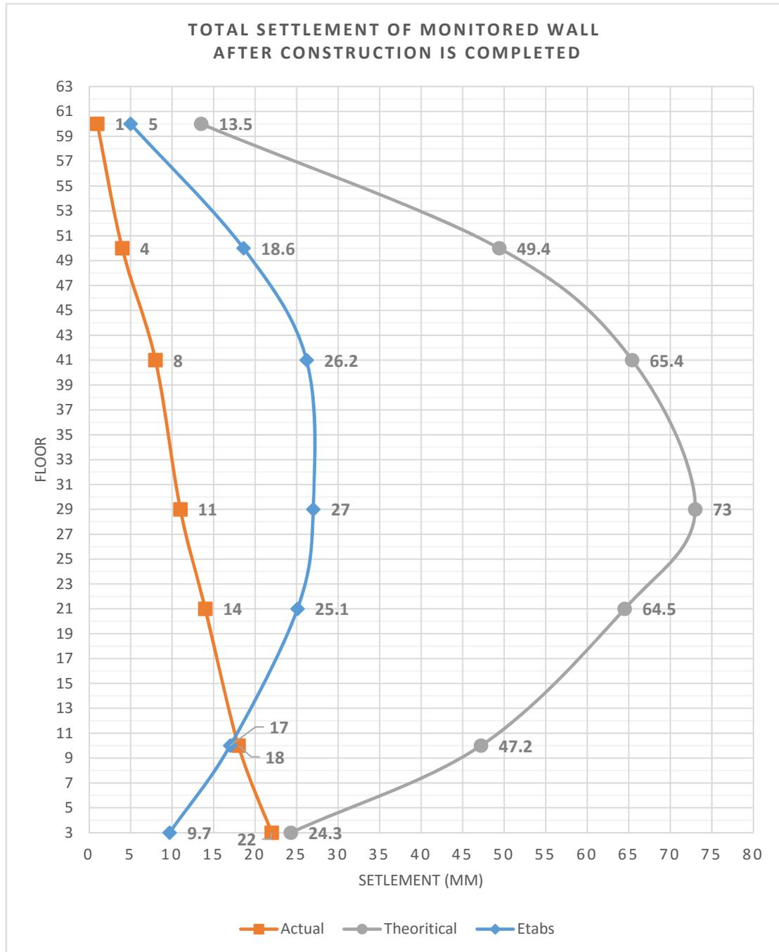
Fig.21 Total settlement of monitored wall after completion of construction
