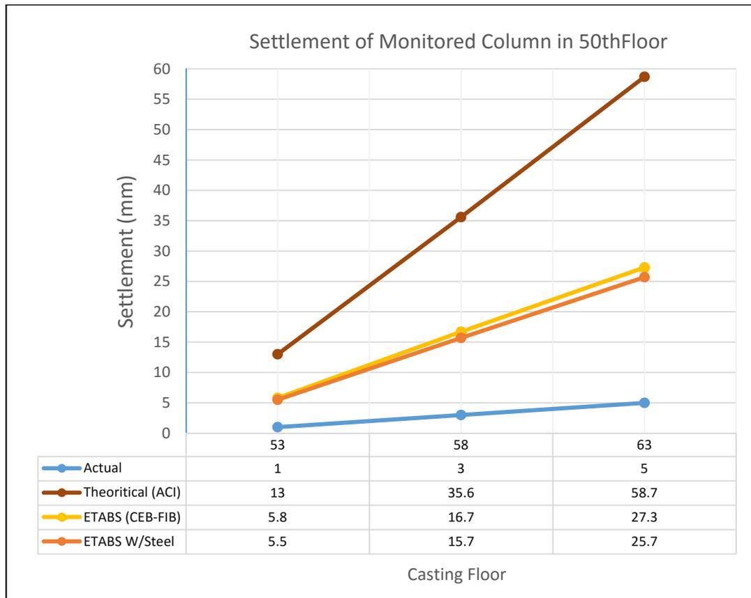
*Fig.19 Actual, Theoretical and ETABS Settlement of Monitored Column in 50<sup>th</sup> Floor*
