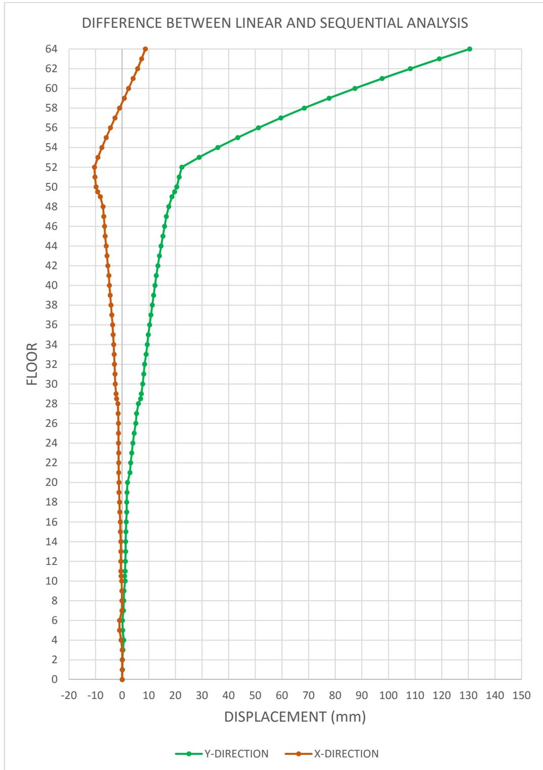
Fig.28 Difference between normal linear and sequential analysis lateral sway
