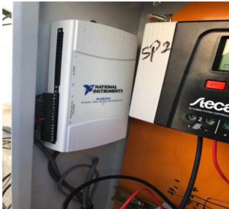
Figure 4.5: Data logger fixed in the testing setup
