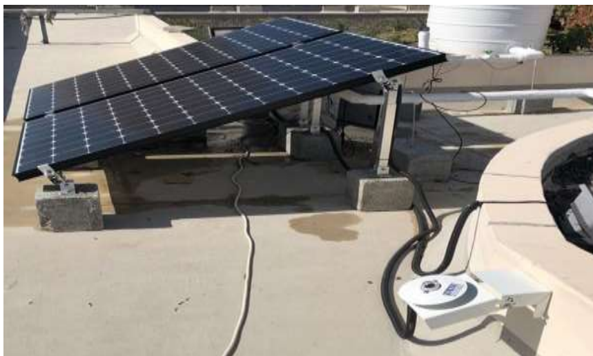
Figure 4.2: Pyranometer installation at the site
