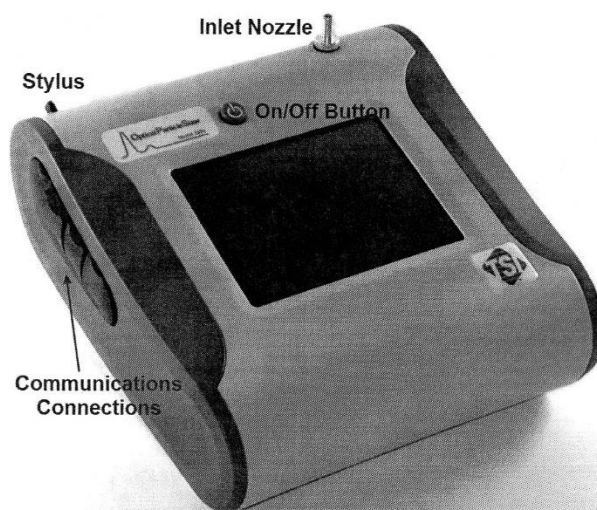
Figure R-1: Different views demonstrating OPS Model 3330 parts (TSI Inc. 2012)
