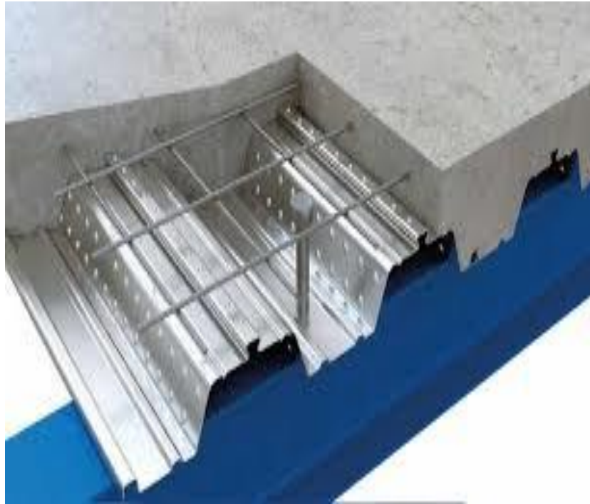
Figure 48: Shape of Deck slab reinforcement and concrete
