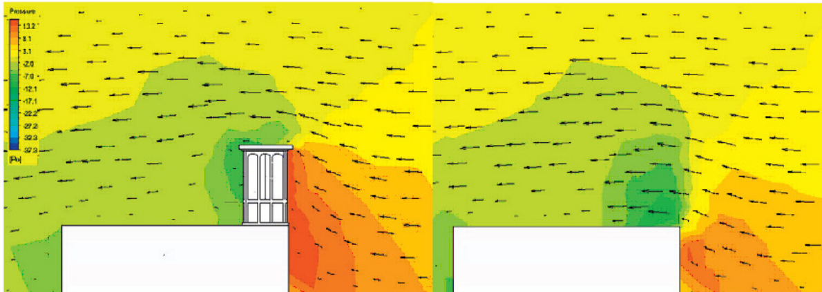
Figure 5.6 Variation in air pressures outside wind tower (Hughes et al 2012)
