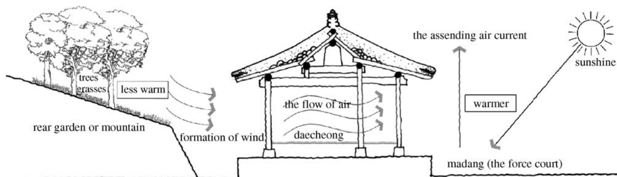
Figure 2.1 Wind flowing from cooler to warmer areas (Kim 2006)
