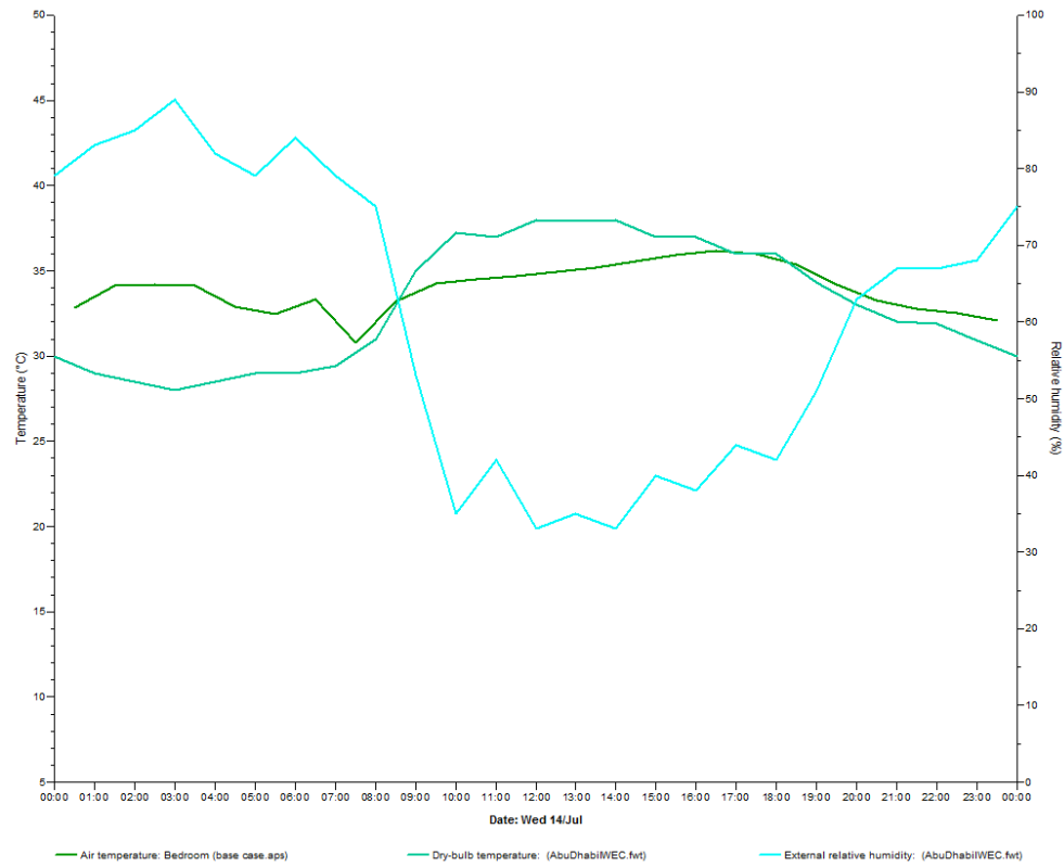
Figure 4.9 External relative humidity and external and internal temperature conditions for 14 July
