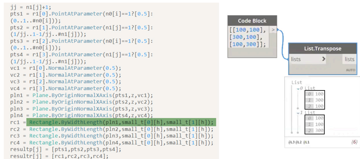
Figure 76: The script error that resulted in creating non-uniform patterns in Dynamo 2.0.3 (author)
