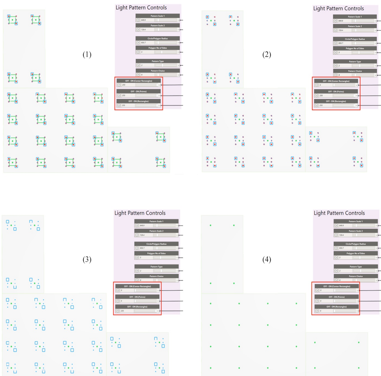
Figure 89: Explanation of the three on/off sliders for the light pattern controllers in Dynamo 2.0.3 (author)
