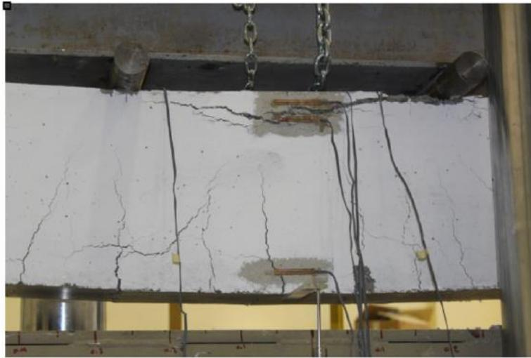
Figure 23: Beam at failure mode
