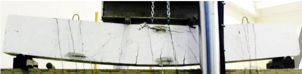
Figure 15: the beam under applied load
