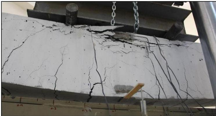
Figure 25: Cracking patterns of Actual OPCC beam
