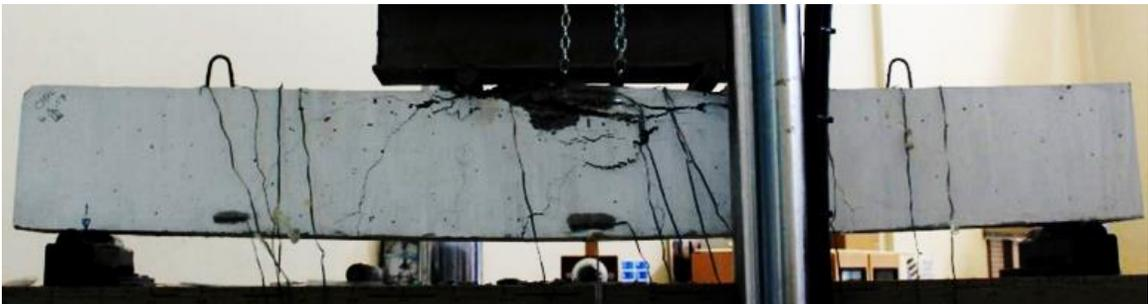
Figure 16: the beam after applied load
