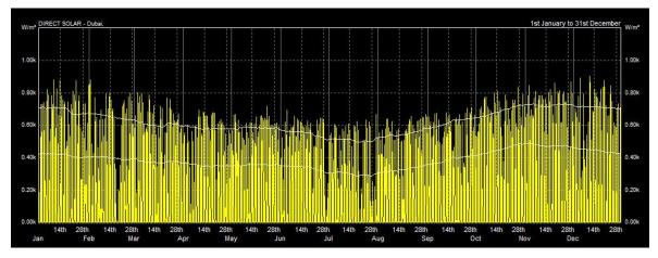
Figure 4.5 Direct Solar Diagram (Ecotect)
