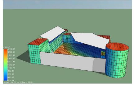
Figure 5.6 Combination of the central shade and the terrace shade (IES-VE)
