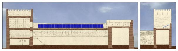
Figure 4.27 Proposed Monocrystalline PV panels at Northern Wing's Terrace (Author)
