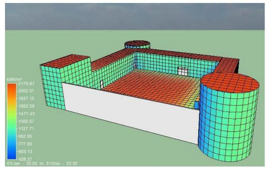
Figure 4.16 Base Simulation Model (IES-VE)
