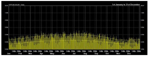
Figure 4.6 Diffused Solar Diagram (Ecotect)
