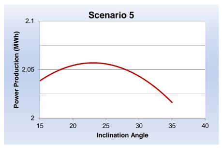
Figure 5.8 PV power production at various inclination angles (IES-VE)
