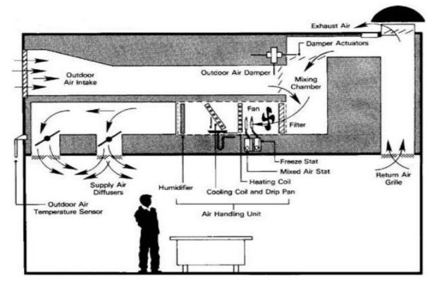
Figure 2.1 : Typical layout of HVAC system components
