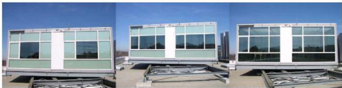
Figure 1: Photographs of the Fraunhofer ISE test facility with the three window configurations (left: small window, middle: medium window, right: large window). The rooms can be rotated fully in order to be more or less independent on seasons to set up a defined (Wienold et al. 2008).
