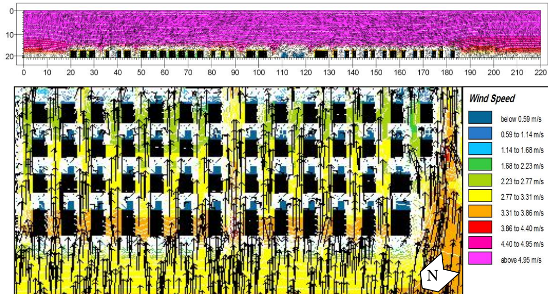
Figure 37: Airflow increases due to increase the distance between buildings
