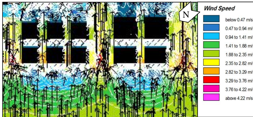
Figure 31: Drive the ventilation by wind speed
