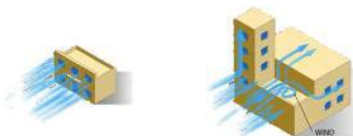
Figure 5: Wind Pressure on Buildings (DM, 2009).
