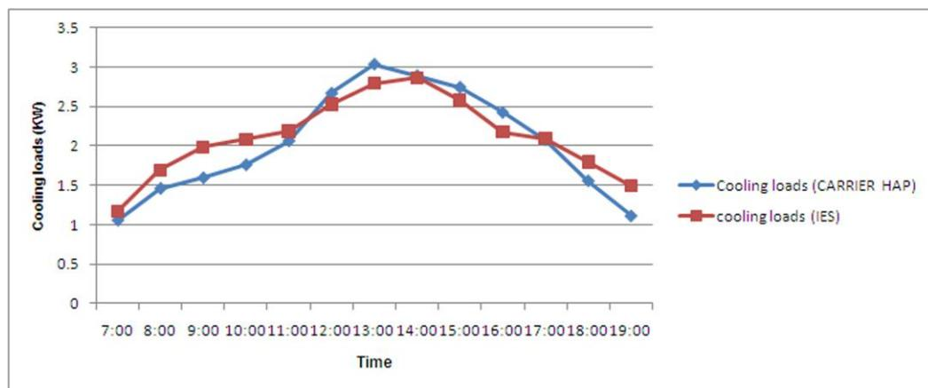
Figure 4.33. CARRIER HAP and IES cooling loads.
