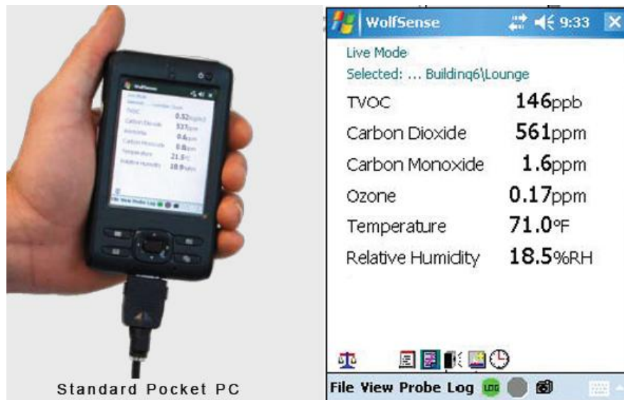
Figure 3.7: PCC and its screen display (Wolf Sense, 2009).
