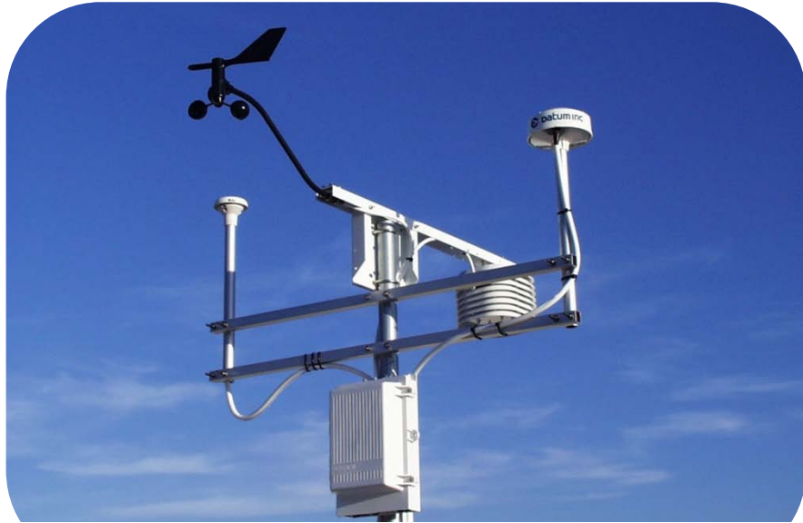
Figure 37 - A typical weather station showing an anemometer and wind vane
