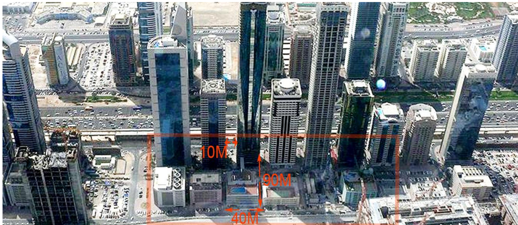
Figure 4.44 Rectangular plots of SZR (40mx90m) use front 30X30m as tower and leave only 10 meter as separation distance to neighbor. While 60 meter in the backside usually used as parking lots or facilities areas.
