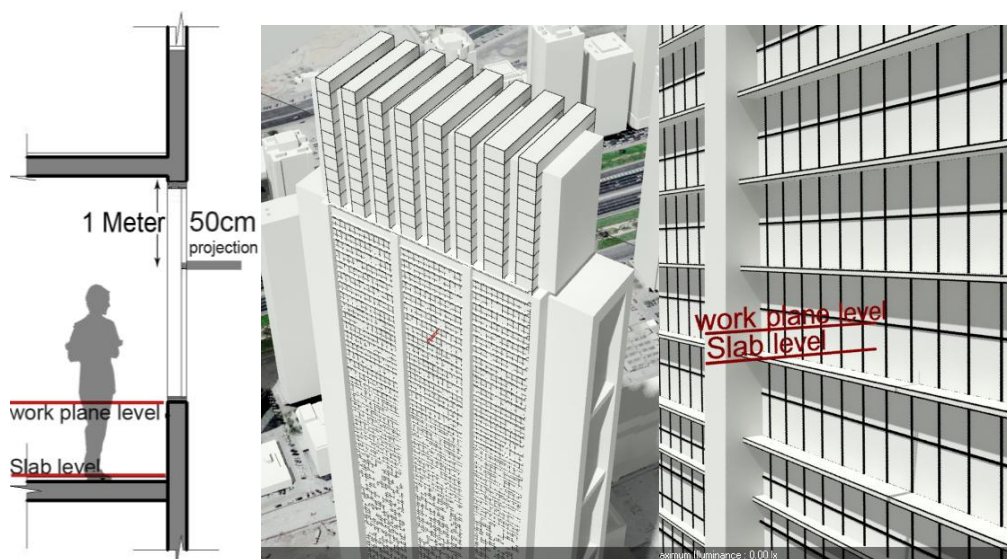
Figure 4.17 Test S.3 daylight illuminance falling on South surface of The Index Tower with a 50 cm projection 1 meter below slab level (1.2 meter above work plane level).
