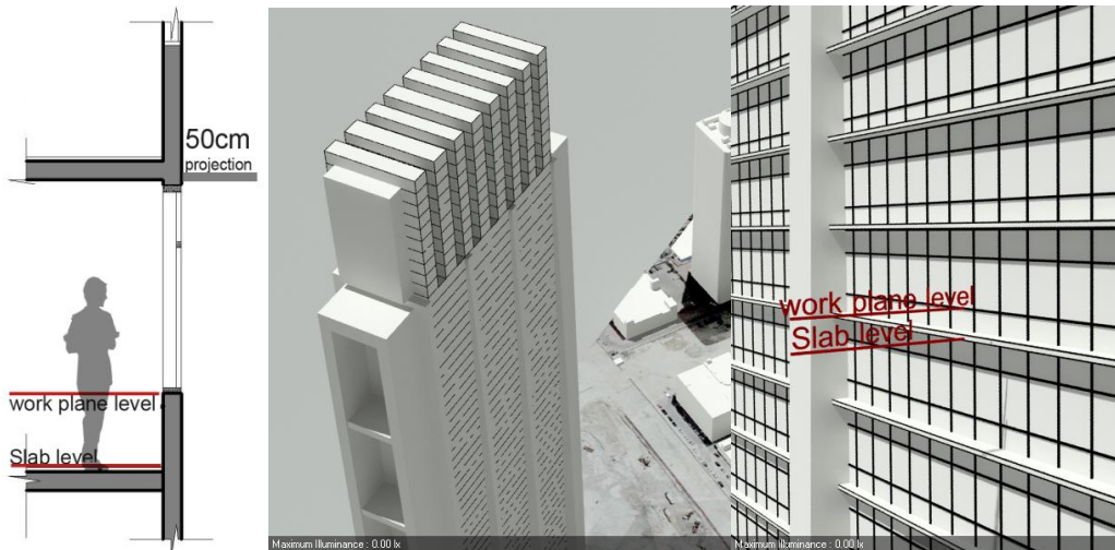
Figure 4.7 Test N.2 daylight illuminance falling on North surface of The Index Tower with 50cm projection from slab level.
