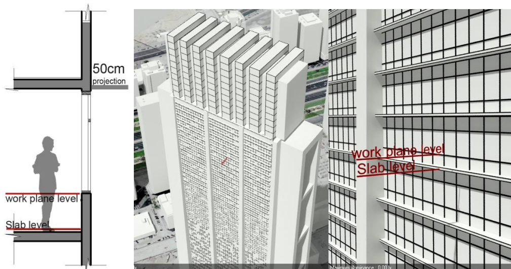
Figure 4.16 Test S.2 daylight illuminance falling on South surface of The Index Tower with a 50 cm projection from slab level.
