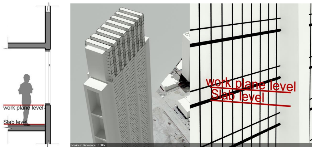
Figure 4.2 Test N.1 daylight illuminance falling on North surface of The Index Tower without shading protections In this test , the light meter is placed on plane north façade without having any protection treatments Figure(4.2). Figures (4.3-5) show the average illumination falling on vertical north surfaces at 3 different times 9:00 am, 12:00 pm and 04:00pm in four seasonal months (March, June, September and December). Data are separated into three groups, Direct, Indirect and Total illumination.
