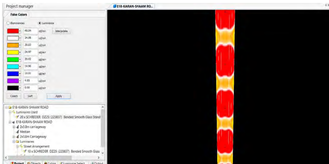
Figure 5.7: HPS lighting system false color rendering
