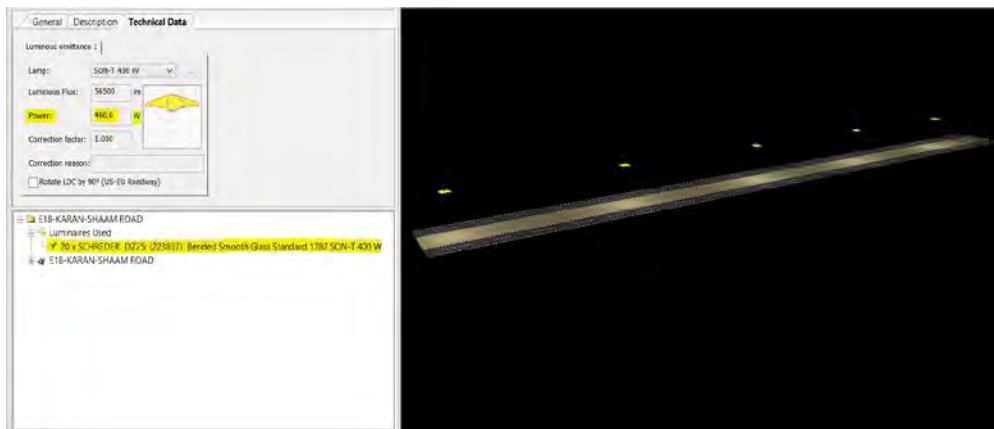
Figure 4.10: Technical specifications of HPS lighting system (Source : Author through DIALux, 2017)
