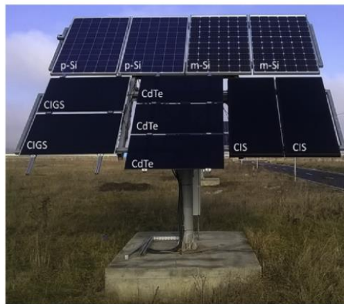
Figure 2.24 Platform P2 with five types of PV modules. (Visa, et al., 2016)
