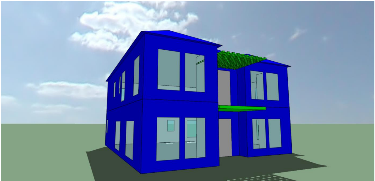
Figure 6.9 Computer model for the villa using IES-VE software.
