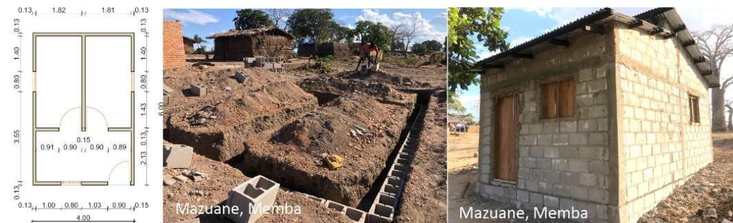
Figure 4.3-43. Cement Blocks walls permanent shelter in Mazuane, Memba. (Shelter Cluster, 2021).
