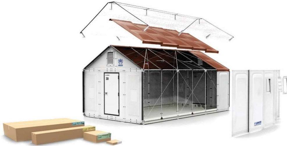
Figure 4.5-7. RHU Flat Packed, Exploded perspective showing the unit components, (UNHCR and IKEA, 2016)
