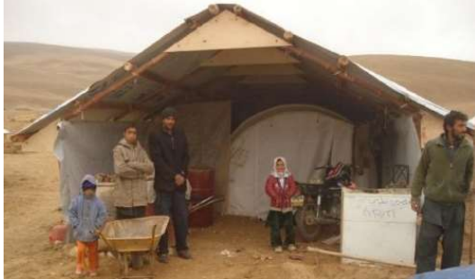
Figure 5.9-24. Bamboo frame covered with plastic sheet built around the existing tents., (UNHCR, 2016)
