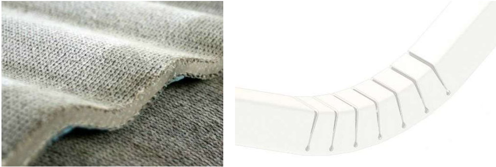
Figure 5.9-6. The use of innovative materials of both Concret textile and easy bendable metallic frames, (Wang, 2019)
