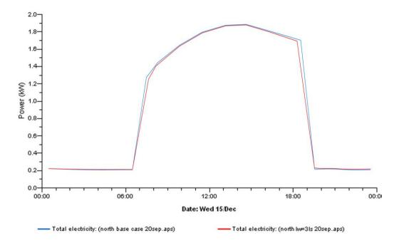
Figure D.1. Hourly energy consumptions (KW) for the louver AR=3 for North orientation on 15<sup>th</sup> of Dec.
