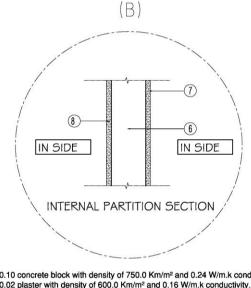
6) 0.10 concrete block with density of 750.0 Km/m<sup>2</sup> and 0.24 W/m.k conductivity.
