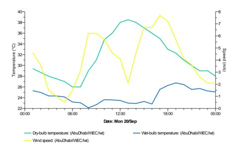
Figure 4.25. Dubai relative temperature and wind speed on Mon 20<sup>th</sup> of Sep. (IES weather database).
