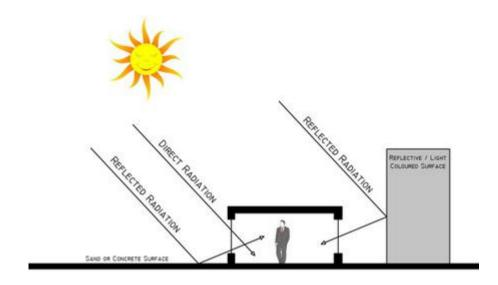
Figure.1.2. Natural daylight can reach the building interior by two main ways, direct solar radiation and diffuse solar radiation. (<u>http://www.aia.org</u>).
