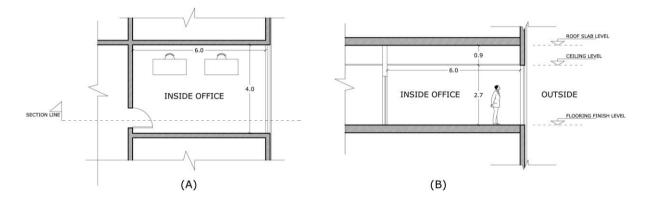
Figure.4.10. (a) typical office units plan, (b) typical office units section.
