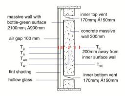
Fig.2.15. Schematic diagram of the structure and locations shading device of the Trombe wall. (Chen et al, 2005).
