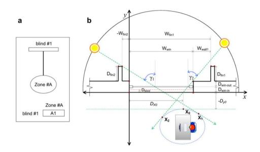
Figure.2.3. Azimuth sun angle analysis with Venetian blind and occupant position, (a) control method for one blind with one controlled zone, (b) minimum and maximum surface solar azimuth angle in horizontal plan. (Koo, Yeo and Kim, 2010).
