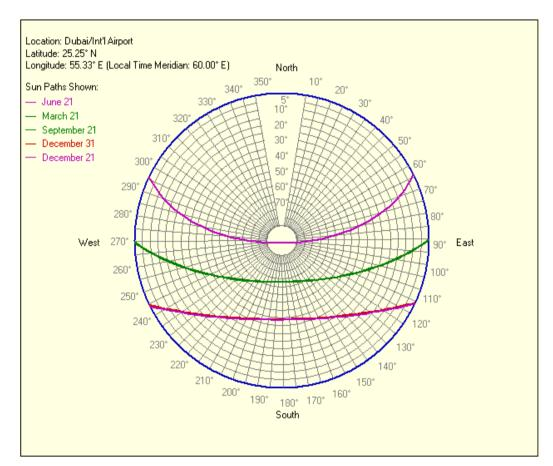
Figure.4.18. Sun path diagram of Dubai. (IES weather database).
