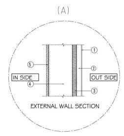
1) 0.004m aluminim with density of 2800.0 Kg/m<sup>2</sup> and 160.0 W/m.k conductivity.
