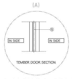
15) 0.040m tember door with density of 419.0 Kg/m² and 0.14 W/m.k conductivity. Not. The CIBSE U-Value for all this materials layers is 2.1608 W/m².k.
