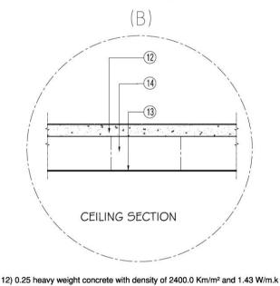
conductivity. 13) 0.004m aluminium ceiling with density of 2800.0 Kg/m<sup>2</sup> and 160.0 W/m.k conductivity. 14) 0.60 cavity. Not. The CIBSE U-Value for all this materials layers is 0.1932 W/m<sup>2</sup>.k.
