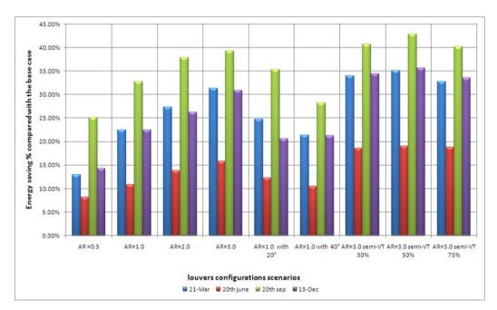
Figure 5.4. Energy saving reduction for louvers scenario compared with the base case for the South orientation.
