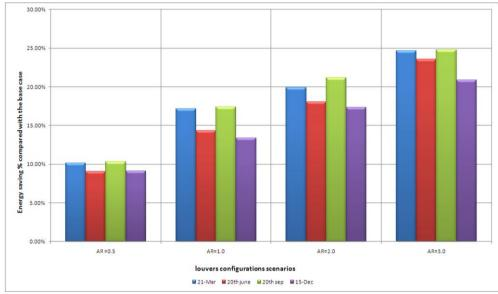
Figure 5.9. Energy saving reduction for louvers scenario compared with the base case for the West orientation.
