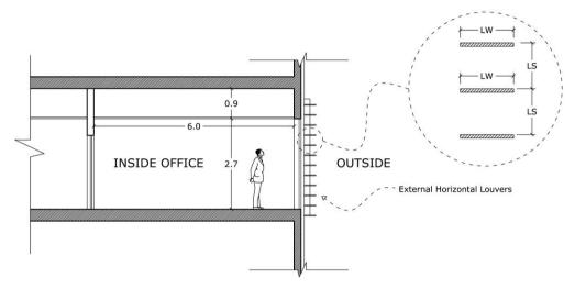
Figure 4.31 The ratio between the louvers spacing distance (LS) and louvers width (LW).
