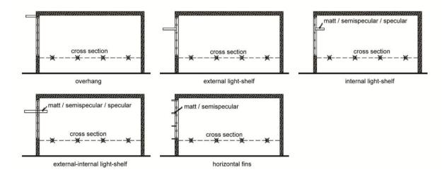
Fig.2.11. Different shading system applications were tested by Aghemo et al (2006).
