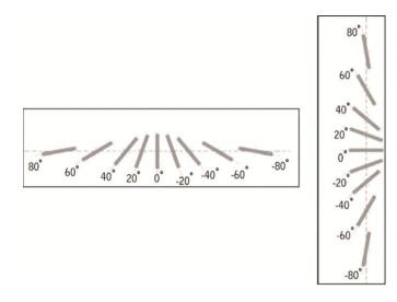
Figure 2.6. Different louvers angles were tested in this thesis. (Hammad and Abu-Hijleh, 2010)
