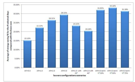
Figure 5.6. Average annual energy saving for louvers scenario compared with the base case for the South orientation.
