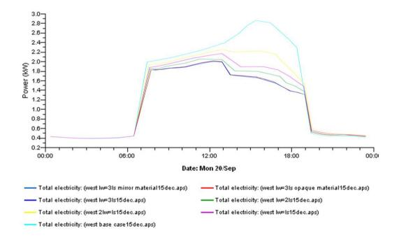
Figure 5.15. Hourly energy consumptions (KW) for all scenarios for the West orientation on 20<sup>th</sup> of Sep.
