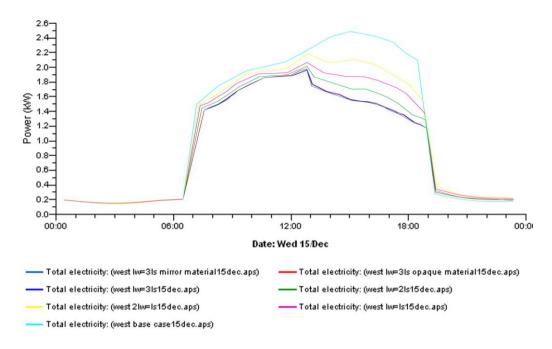
Figure C.1. Hourly energy consumptions (KW) for all scenarios for West orientation on 15<sup>th</sup> of Dec.
