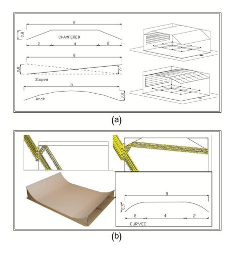
Fig.2.10. Ceiling geometry shape with louvers shading models, (a) Virtual model test, (b) physical model test. (Freewan et al, 2008).
