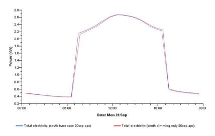
Figure 5.2. Total energy consumptions (KW) for the base case and the light dimming system without louvers shading.
