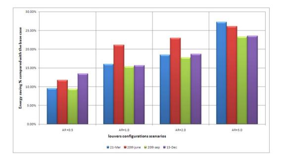
Figure 5.7. Energy saving reduction for louvers scenario compared with the base case for the East orientation.
