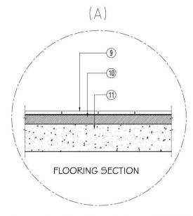
09) 0.04m granite with density of 2100.0 Kg/m<sup>2</sup> and 1.70 W/m.k conductivity.
