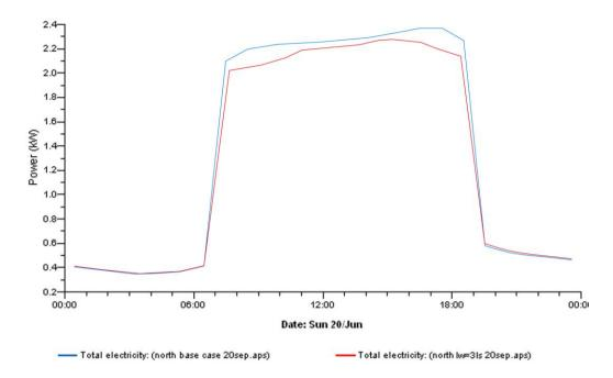
Figure D.3. Hourly energy consumptions (KW) for the louver AR=3 for North orientation on  $20^{th}$  of Jun.
