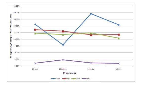
Figure 5.12. Energy saving% for louvers AR=3 compared with the base case for the West, East and South orientations during the four seasons.
