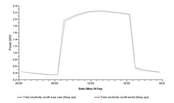
Figure D.4. Hourly energy consumptions (KW) for the louver AR=3 for North orientation on 20<sup>th</sup> of Sep.
