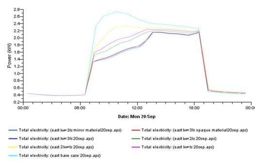
Figure B.4. Hourly energy consumptions (KW) for all scenarios for East orientation on 20<sup>th</sup> of Sep.
