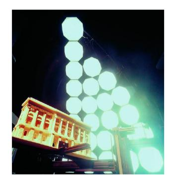
Figure 3.1. Artificial sky dome with scaled model used to test the shading device performance. (Aghemo et al, 2007).
