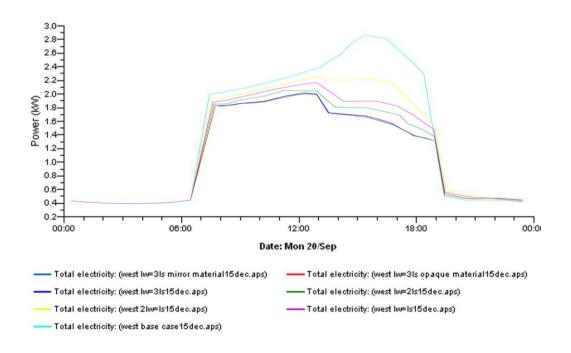
Figure C.4. Hourly energy consumptions (KW) for all scenarios for West orientation on 20<sup>th</sup> of Sep.
