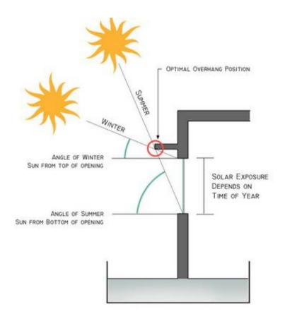
Figure.2.5. Ideal basic shading strategy for external fixed shading device in deferent seasons. (<u>http://www.aia.org</u>).
