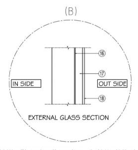
16) 0.006m pilkington glass with transmittance valu of 0.44 and 0.33 and exterior reflictance and 0.15 inside reflectance.
