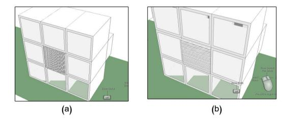
Figure.4.11. Office unit, virtual model on IES. (a) Vertical external louvers installation for the East and West façade, (b) horizontal external louvers installation for the south façade.
