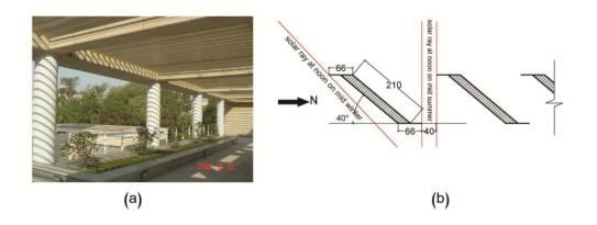
Fig.2.13. Rooftop shading application, (a) existing photo, (b) dimensions of roof shading device. (Meng and Zhang, 2006).
