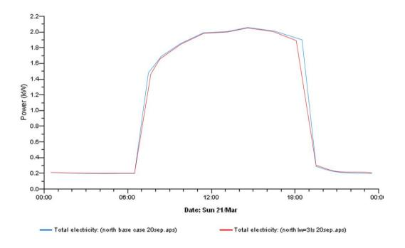
Figure D.2. Hourly energy consumptions (KW) for the louver AR=3 for North orientation on 21<sup>st</sup> of March.
