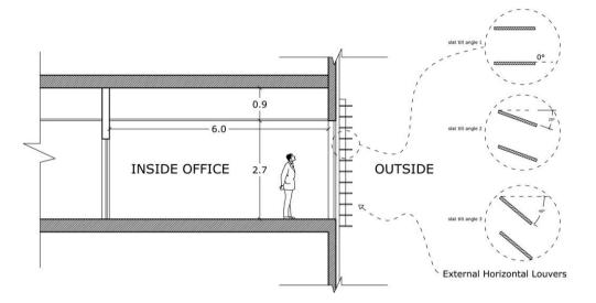
Figure 4.32. Louvers slate tilt angles.
