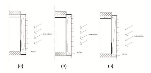
Fig.2.9. Movable shading system in three configurations as a thermal solution in hot season, (a) closed natural conviction, (b) open natural conviction, (c) forced conviction. (Baldinelli, 2008).
