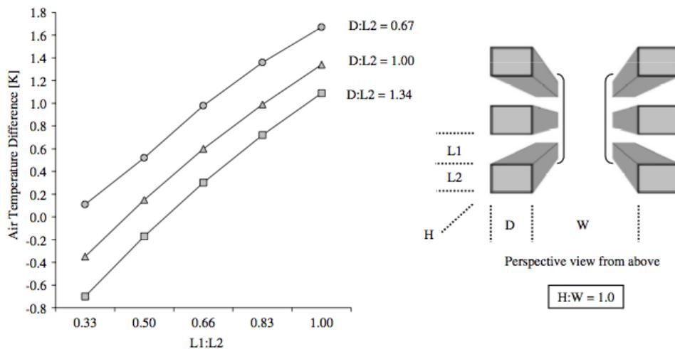
**Figure 2.2** A graph illustrating the impact of geometry on air temperature for aspect ratio of 1.0 (Shashua-Bar et al., 2004)
