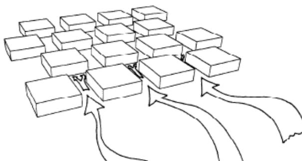
**Figure 2.8** Staggered and offset street layout breaks down the wind velocity (Golany, 1996)
