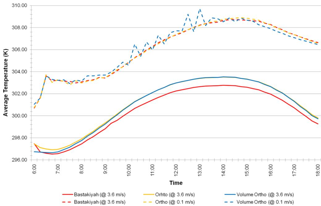
**Figure 5.5** Daily average temperature (m/s) for Bastakiyah, Ortho, and Volume Ortho configurations in September for both 3.6m/s and 0.1m/s initial wind speed scenarios.
