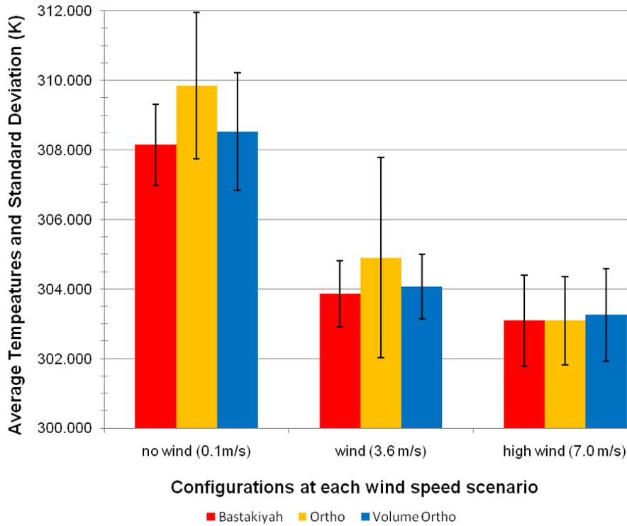
**Figure 5.13** Comparison of average temperature and standard deviation in all three wind scenarios (0.1m/s, 3.6m/s, and 7m/s)
