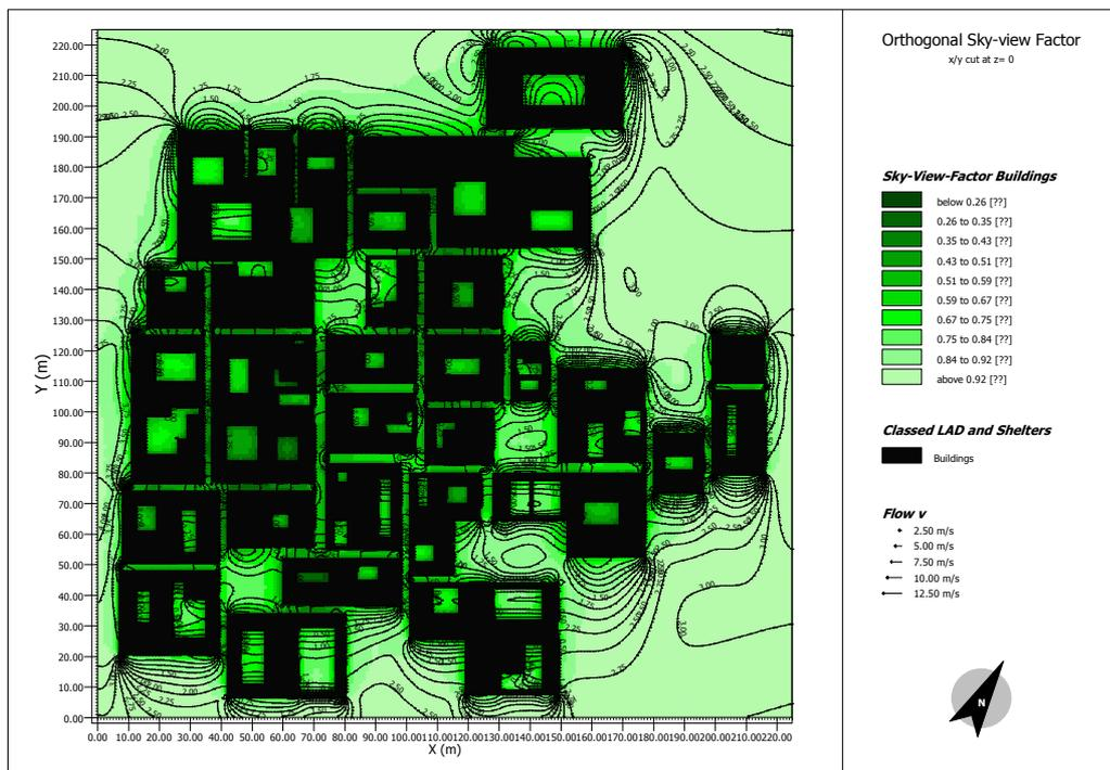
Figure 5.15 Orthogonal configuration sky-view factor gradient
