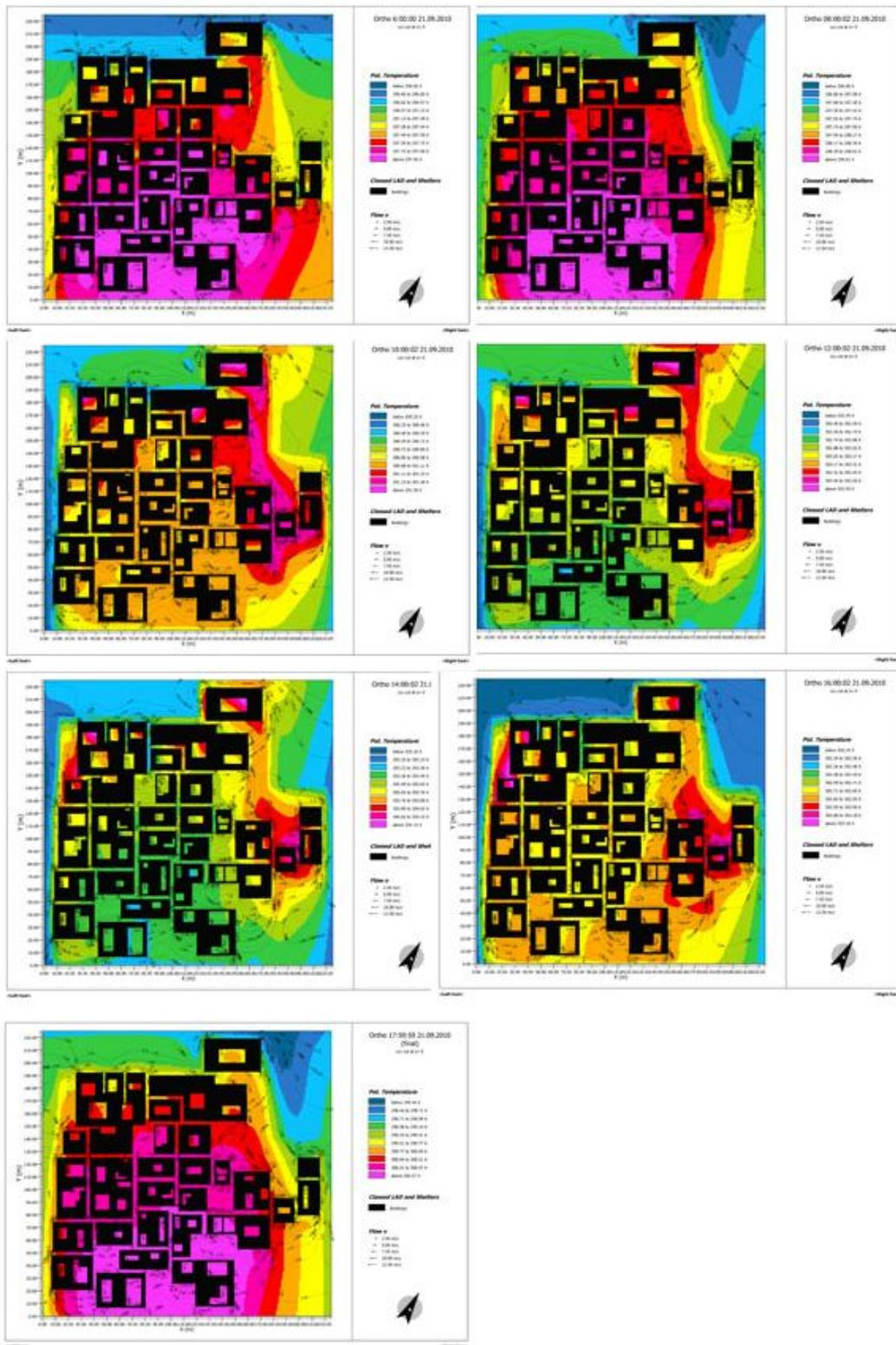
**Figure F.5** Temperature gradient for Orthogonal in September and initial wind speed 3.6m/s
