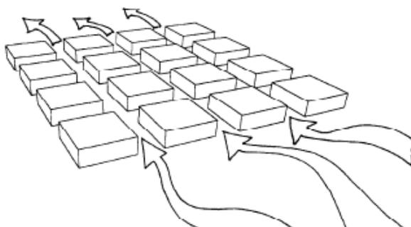
**Figure 2.7** Grid layout allows for wind penetration deep within the layout (Golany, 1996)
