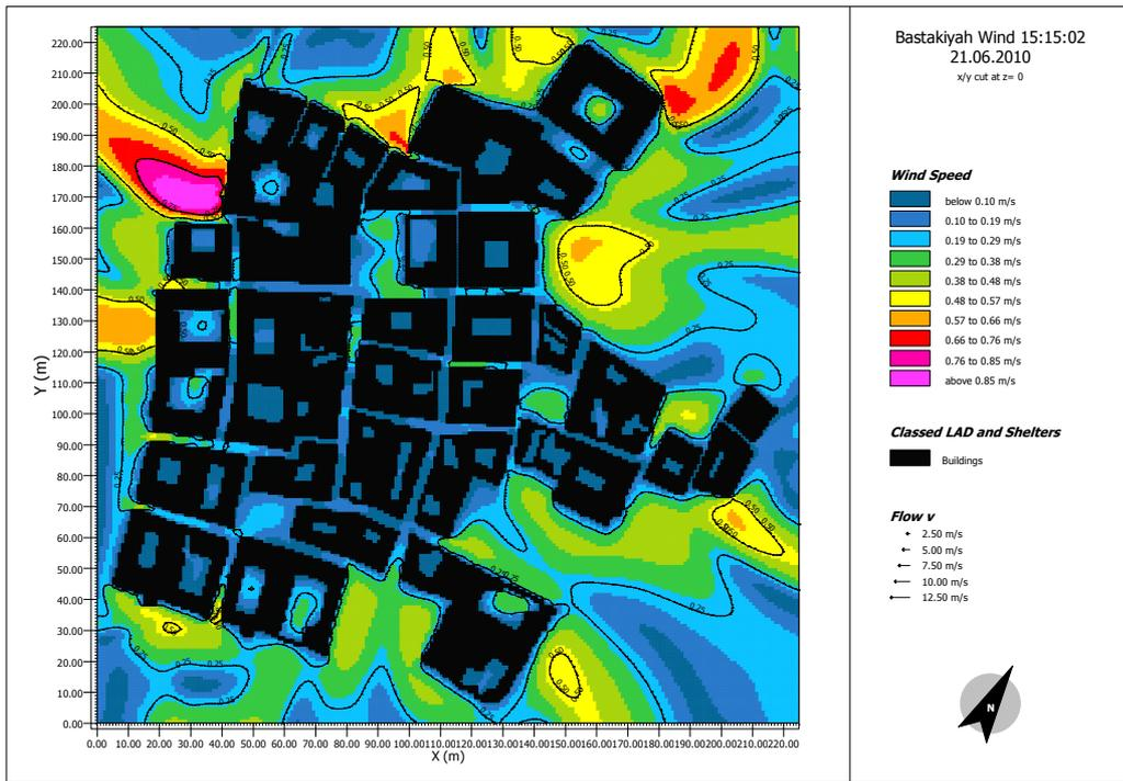
**Figure 5.23** Snapshot of wind behavior in Bastakiyah at 15:15 in June in absence of wind (0.1 m/s)
