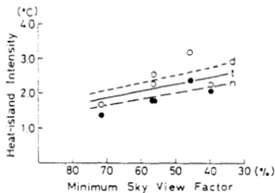
**Figure 2.15** Graphs showing the relationship between minimum sky view factor and heat island intensity (Yamashita et al., 1986)
