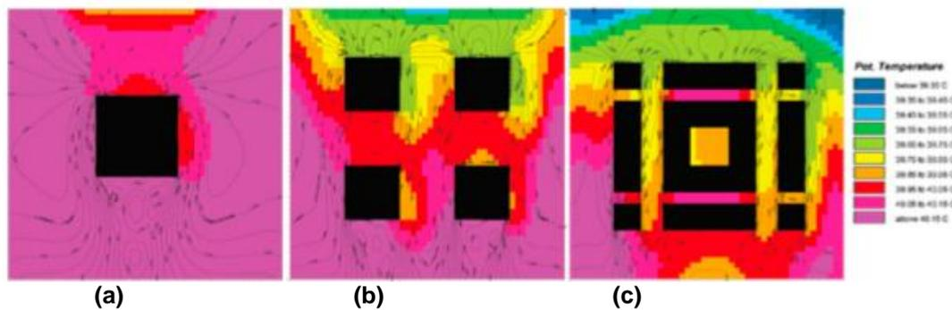
**Figure 2.3** ENVI-met simulation results for (a) single high rise building, (b) four block mid-rise buildings, (c) dense courtyard block (Thapar and Yannas, 2008)
