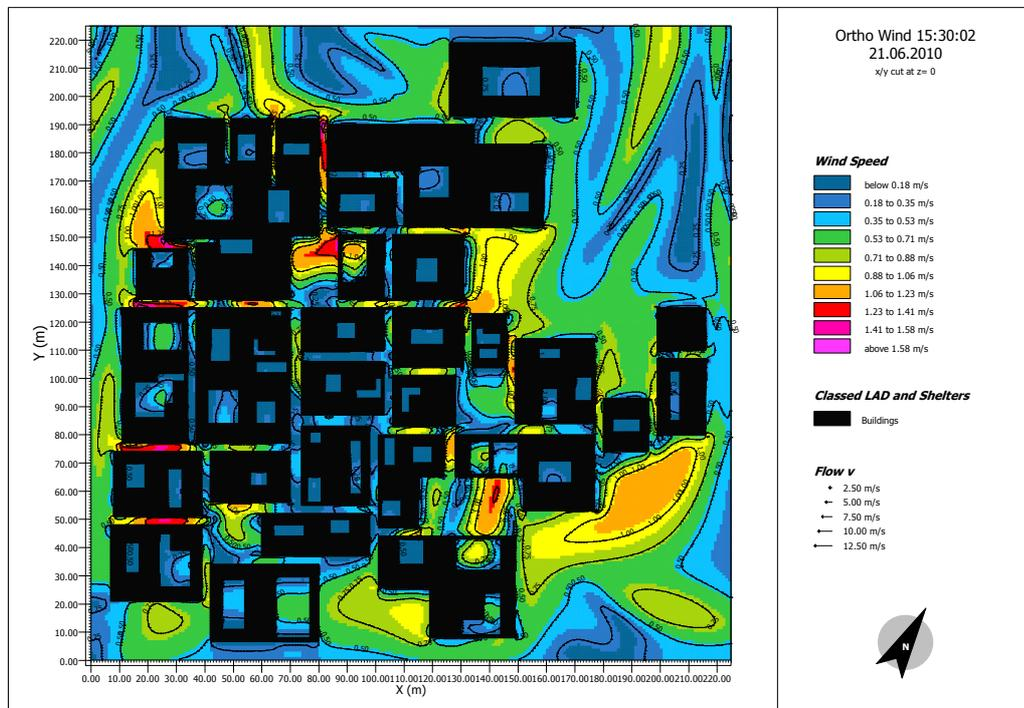
Figure 5.26 Snapshot of wind behavior in Orthogonal configuration at 15:30 in June in absence of wind (0.1 m/s).
