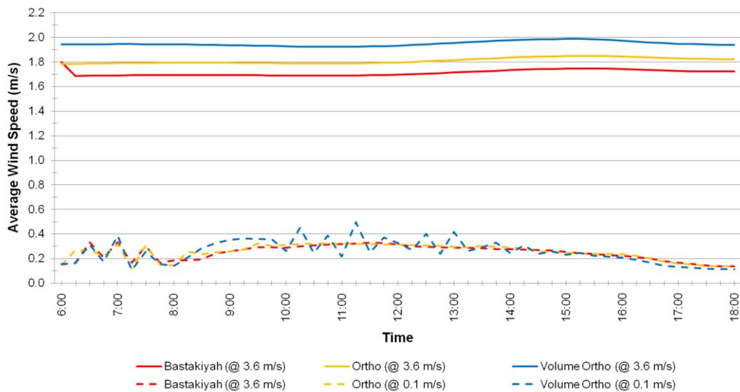
**Figure 5.6** Daily average wind speed (m/s) for Bastakiyah, Ortho, and Volume Ortho configurations in September for both 3.6m/s and 0.1m/s initial wind speed scenarios.
