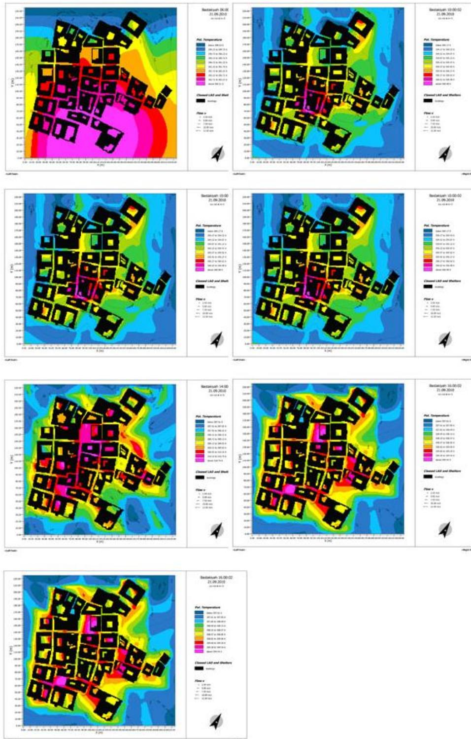
**Figure G.2** Temperature gradient for Bastakiyah in September and initial wind speed 0.1m/s
