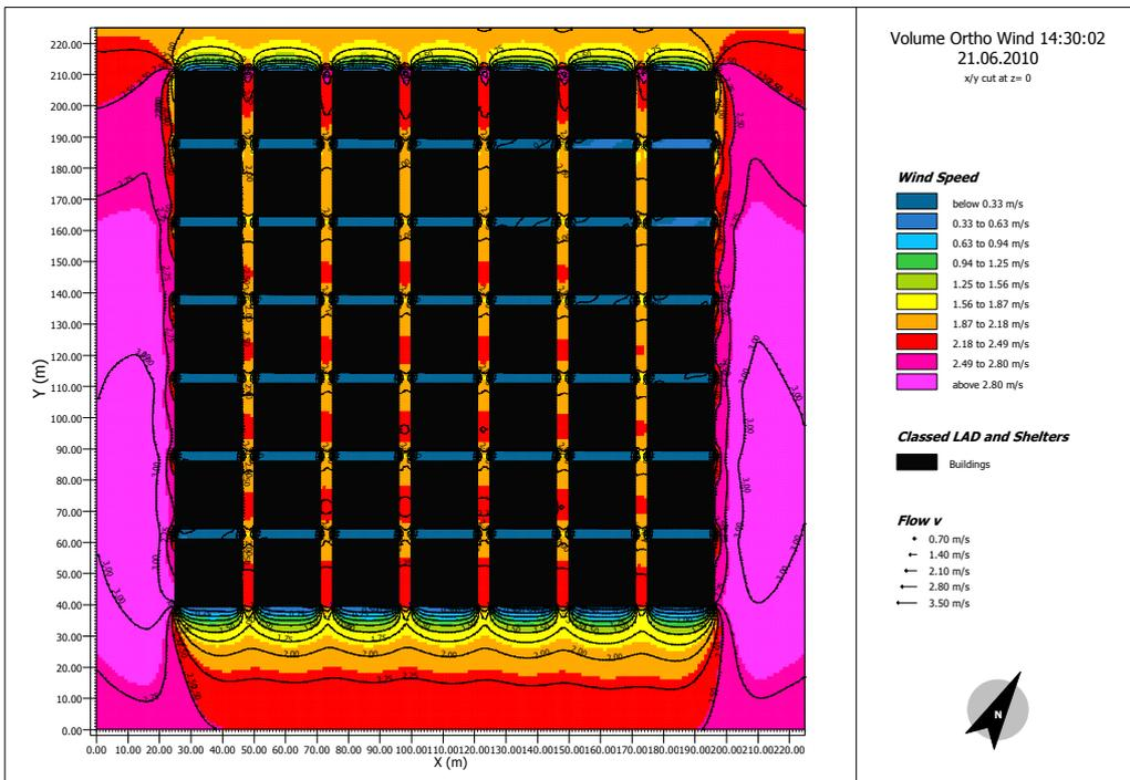
**Figure 5.20** Snapshot of wind contours in Volume Ortho at 14:30 in June showing the distribution of wind throughout the configuration (initial wind at 3.6m/s)
