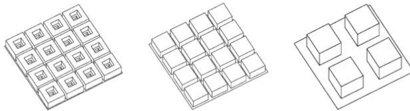
**Figure 2.5** Axonometric of the investigated urban forms (left to right: 3 floor courtyards, three floor micro pavilion, six floor pavilion) (Ratti et al., 2003)
