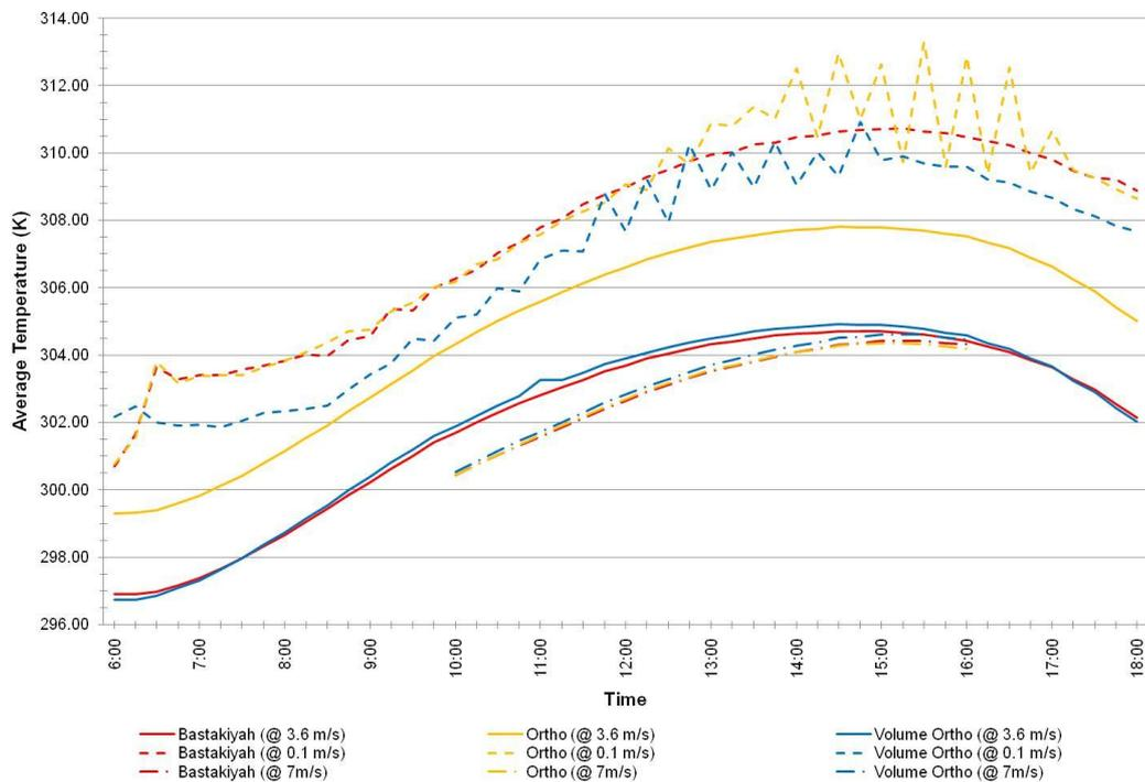
**Figure 5.12** Average temperature trends for the three configurations in three initial wind speed scenarios (0.1, 3.6, and 7 m/s) in June from 10:00-16:00
