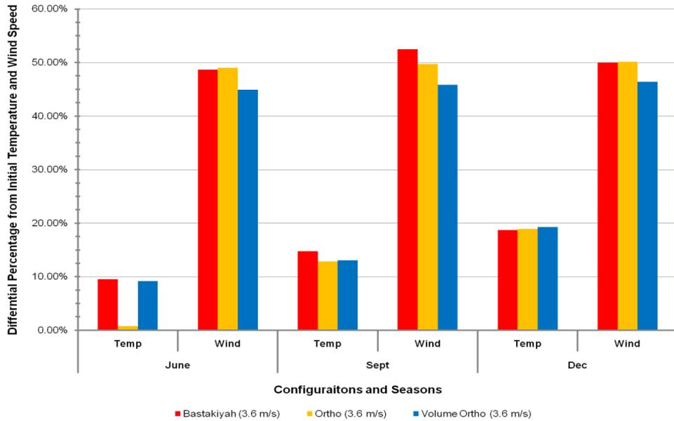
**Figure 5.11** Differential percentages from initial temperature and wind input for Bastakiyah, Ortho, and Volume Ortho configurations in the three seasons for initial wind speed of 3.6m/s.
