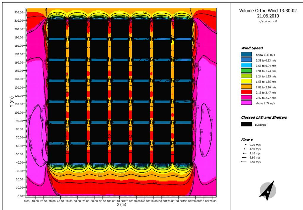
**Figure 5.28** Snapshot of wind behavior in Volume Ortho configuration at 13:30 in December with initial wind speed of 3.6m/s
