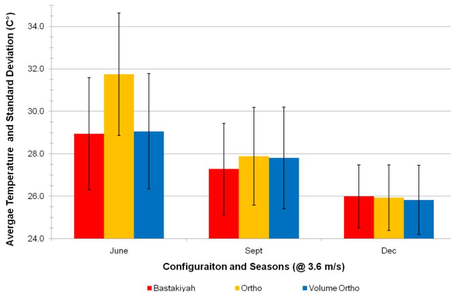
**Figure 5.7** Average temperatures and standard deviations for Bastakiyah, Ortho, and Volume Ortho configurations in the three seasons for initial wind speed of 3.6m/s.
