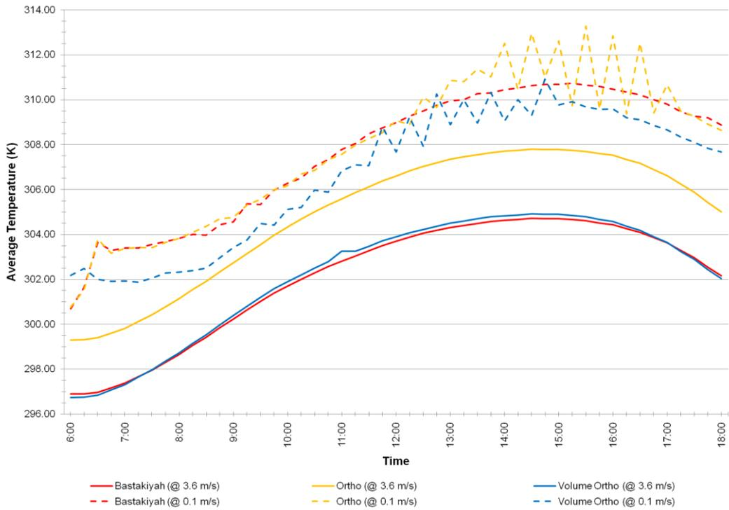
**Figure 5.1** Daily average temperatures (K) for Bastakiyah, Ortho, and Volume Ortho configurations in June for both 3.6m/s and 0.1m/s initial wind speed scenarios
