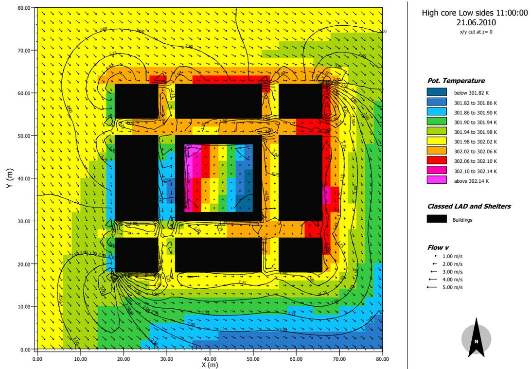
**Figure 4.1 (a)** Simulation results for a model with high courtyard block (10m) and low surrounding blocks (6m)
