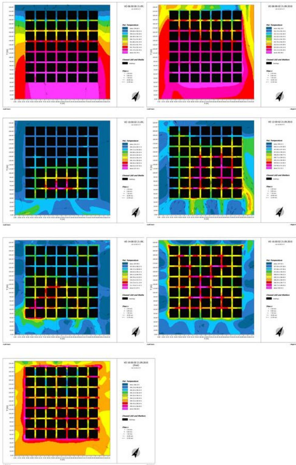
**Figure G.8** Temperature gradient for Volume Ortho in September and initial wind speed 0.1m/s
