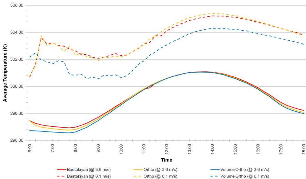
**Figure 5.3** Daily average temperatures (K) for Bastakiyah, Ortho, and Volume Ortho configurations in December for both 3.6m/s and 0.1m/s initial wind speed scenarios
