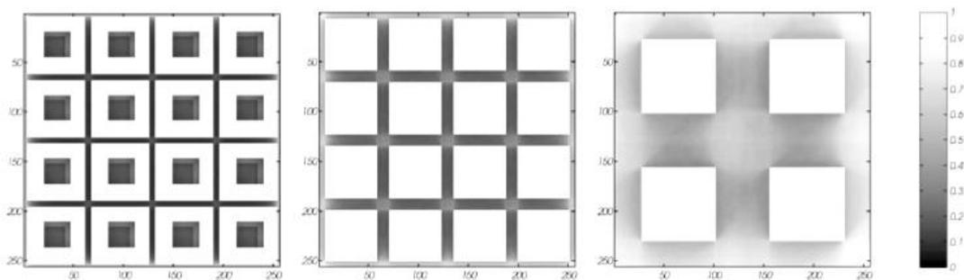
**Figure 2.6** Sky view factors from street level for the three urban configurations (Ratti et al., 2003)
