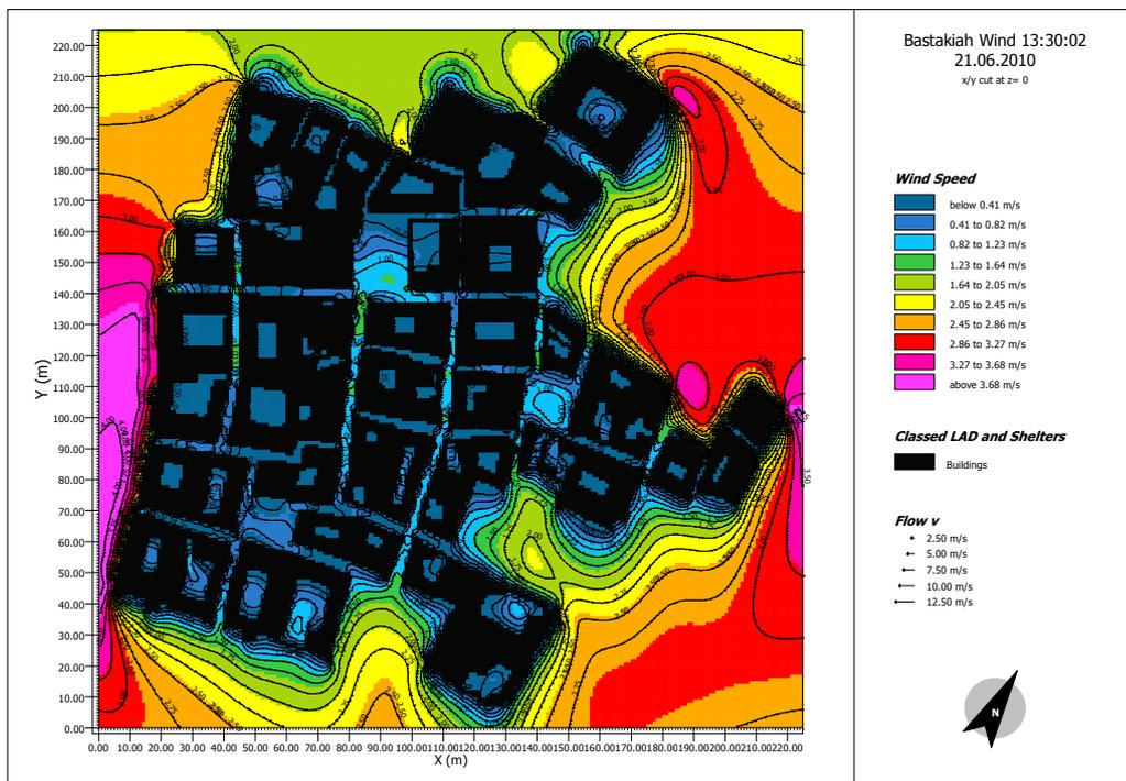
**Figure 5.27** Snapshot of wind behavior in Bastakiyah configuration at 13:30 in December with initial wind speed of 3.6m/s
