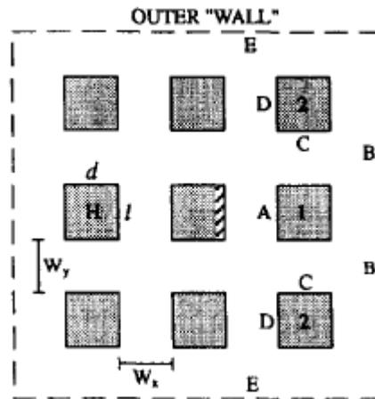
**Figure 2.17** A sketch defining the parameters of the simulated model ( $H$ = height of the structure,  $W$ = spacing between structures,  $d$ = depth of the structure,  $l$ = length of the structure (Mills, 1997)
