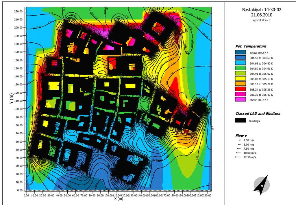
**Figure 5.17** Snapshot of temperature gradient in Bastakiyah at 14:30 in June showing a difference in temperature values across the configuration (initial wind speed at 3.6m/s).
