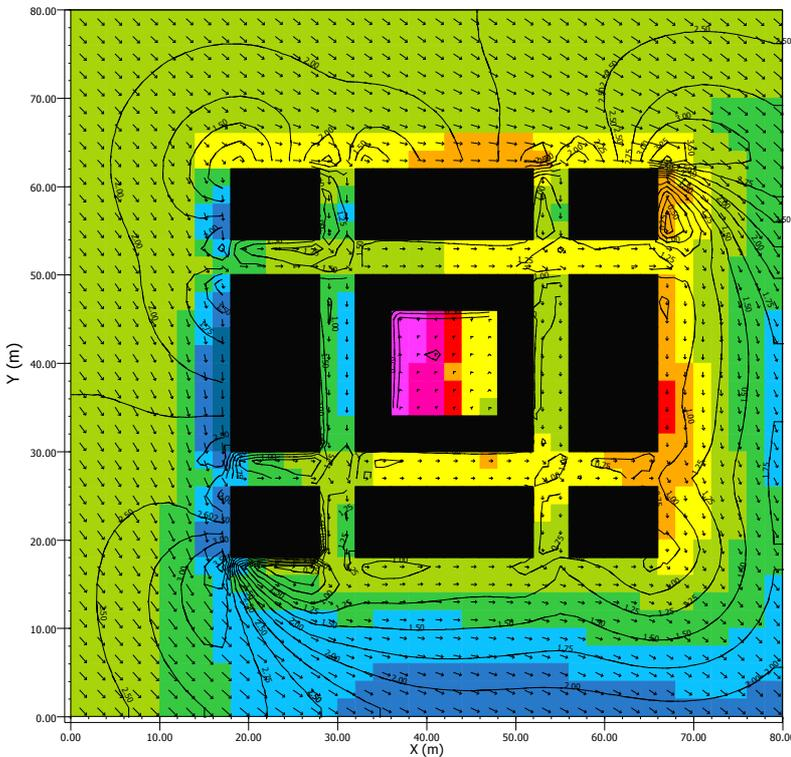
Figure 4.2 (b) Simulation results for thicker courtyard wall
