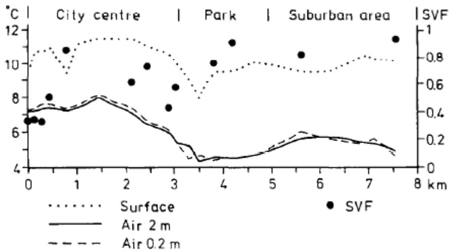
**Figure 2.16** Graph showing air and surface temperature with regards to SVF and distance from city center (Eliasson, 1996)
