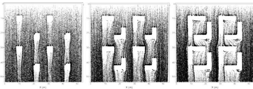
**Figure 2.10** ENVI-met air flow results from different directions at different heights of the RSB form (Okeil, 2010)
