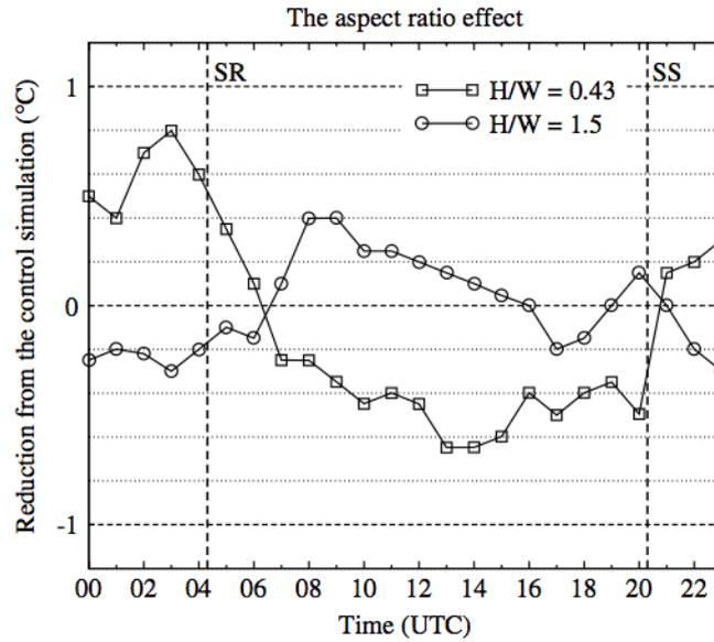
**Figure 2.13** Graph showing the difference in behavior of two aspect ratios with respect to their temperature reduction values from a control simulation (Hamdi and Schayes, 2008).
