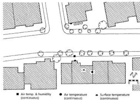
**Figure 2.18** Illustration showing the location of measurements in **(a)** deep canyon in the old city fabric and in **(b)** shallow canyon in a modern city fabric (Johansson, 2006)
