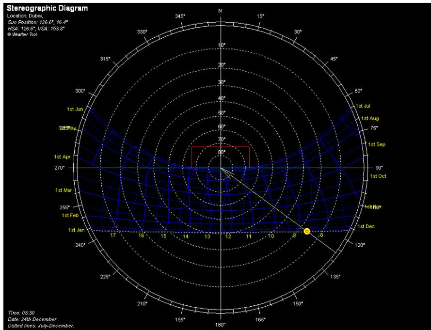
Figure 3.4 Stereograph for solar position in Dubai, UAE (Ecotect)
