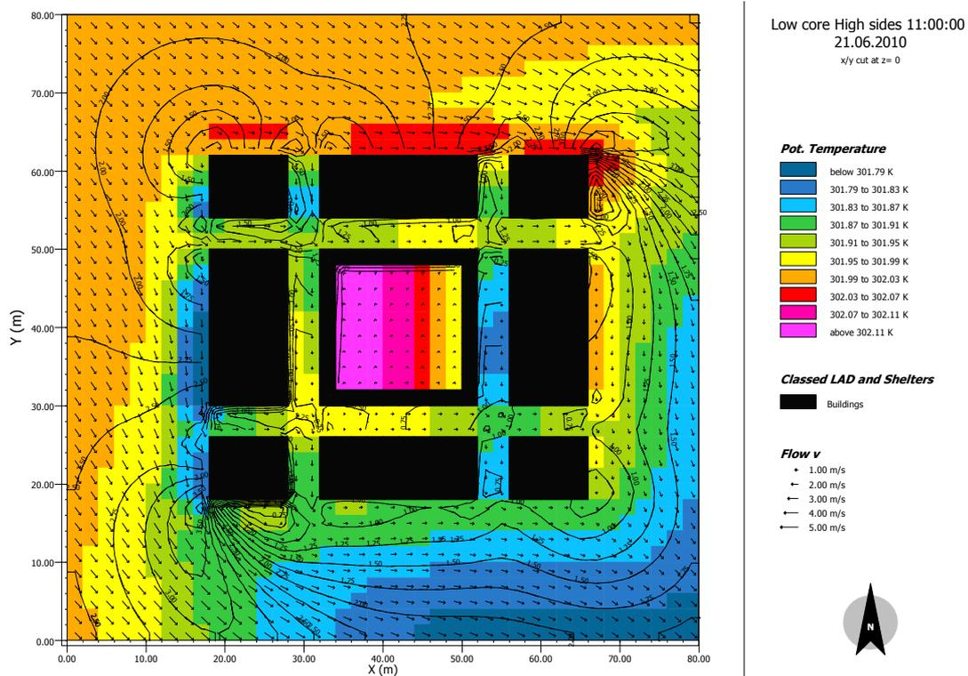
**Figure 4.1 (b)** Simulation results for a model with low courtyard block (6m) and high surrounding blocks (10m)
