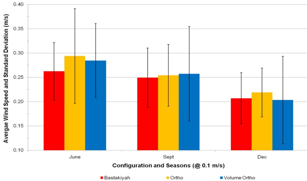
**Figure 5.10** Average wind speeds and standard deviations for Bastakiyah, Ortho, and Volume Ortho configurations in the three seasons for initial wind speed of 0.1 m/s.
