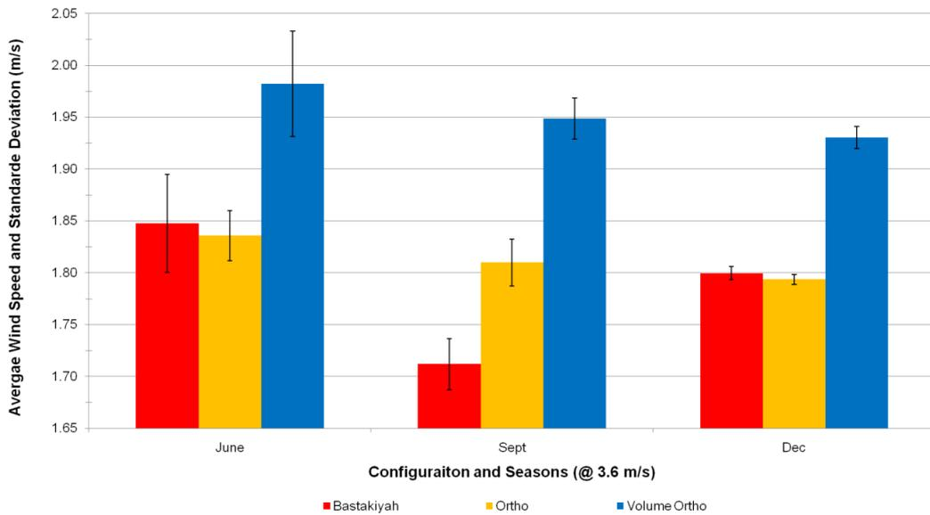
**Figure 5.8** Average wind speeds and standard deviations for Bastakiyah, Ortho, and Volume Ortho configurations in the three seasons for initial wind speed of 3.6m/s.
