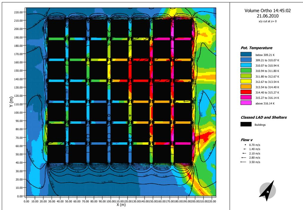
**Figure 5.22** Snapshot of temperature variation in Volume Ortho at 14:45 in June in absence of wind (0.1 m/s) showing the distribution of temperature in one part of the configuration.
