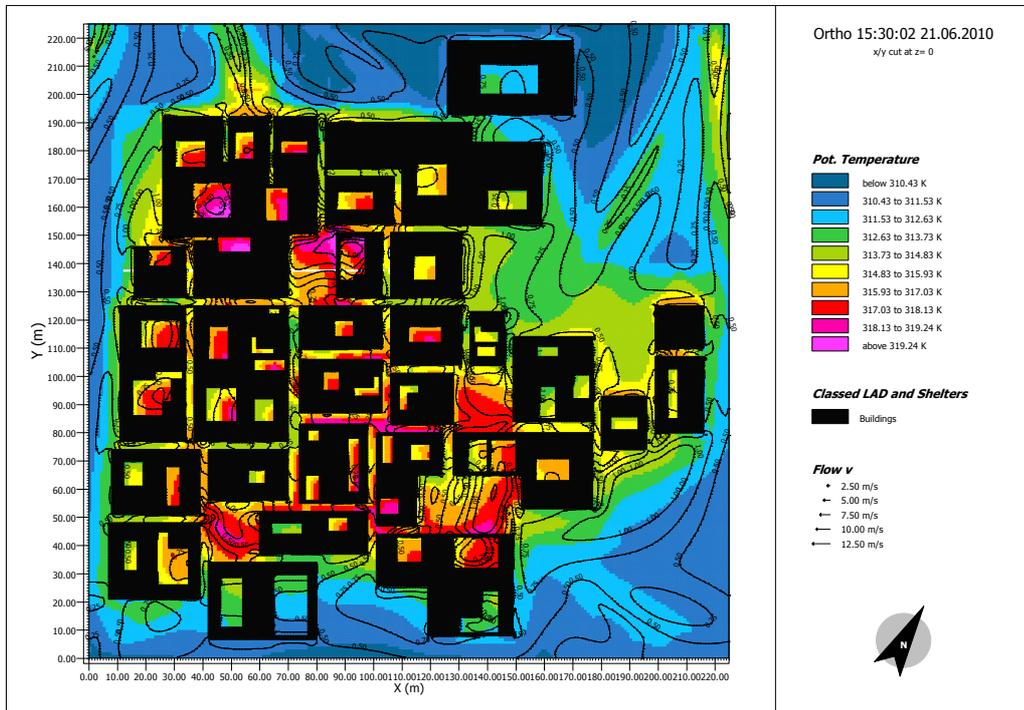
Figure 5.25 Snapshot of temperature variation in Orthogonal configuration at 15:30 in June in absence of wind (0.1 m/s).
