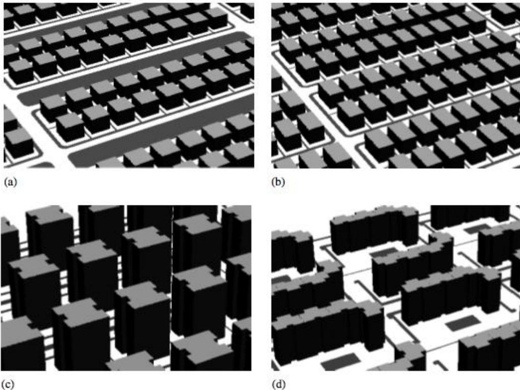
**Figure 2.1** Diagram to illustrate the different investigated aspect ratios **(a)**  $H/W = 0.25$ , **(b)**  $H/W = 0.5$ , **(c)**  $H/W = 1.0$ , **(d)**  $H/W = 2.0$  (Shashua-Bar et al., 2004)
