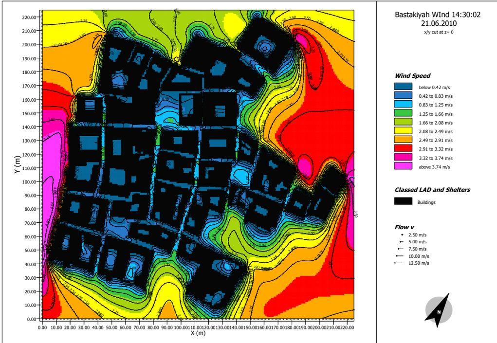
**Figure 5.19** Snapshot of wind contours in Bastakiyah at 14:30 in June showing the distribution of wind throughout the configuration (initial wind at 3.6m/s).
