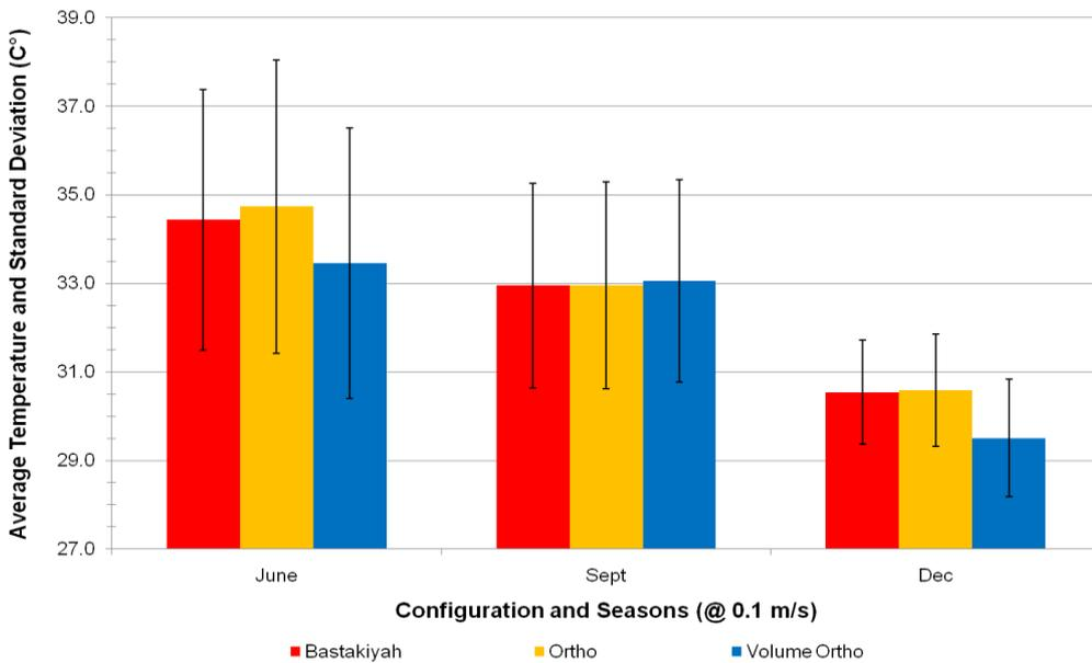
**Figure 5.9** Average temperatures and standard deviations for Bastakiyah, Ortho, and Volume Ortho configurations in the three seasons for initial wind speed of 0.1 m/s.
