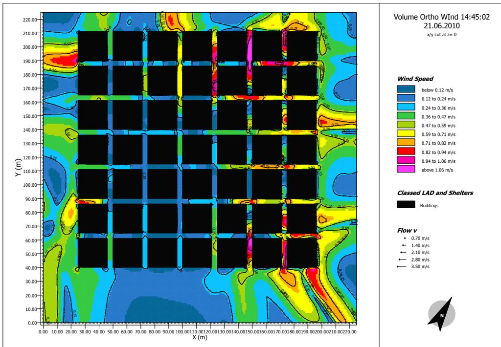
**Figure 5.24** Snapshot of wind behavior in Volume Orto at 14:45 in June in absence of wind (0.1 m/s).
