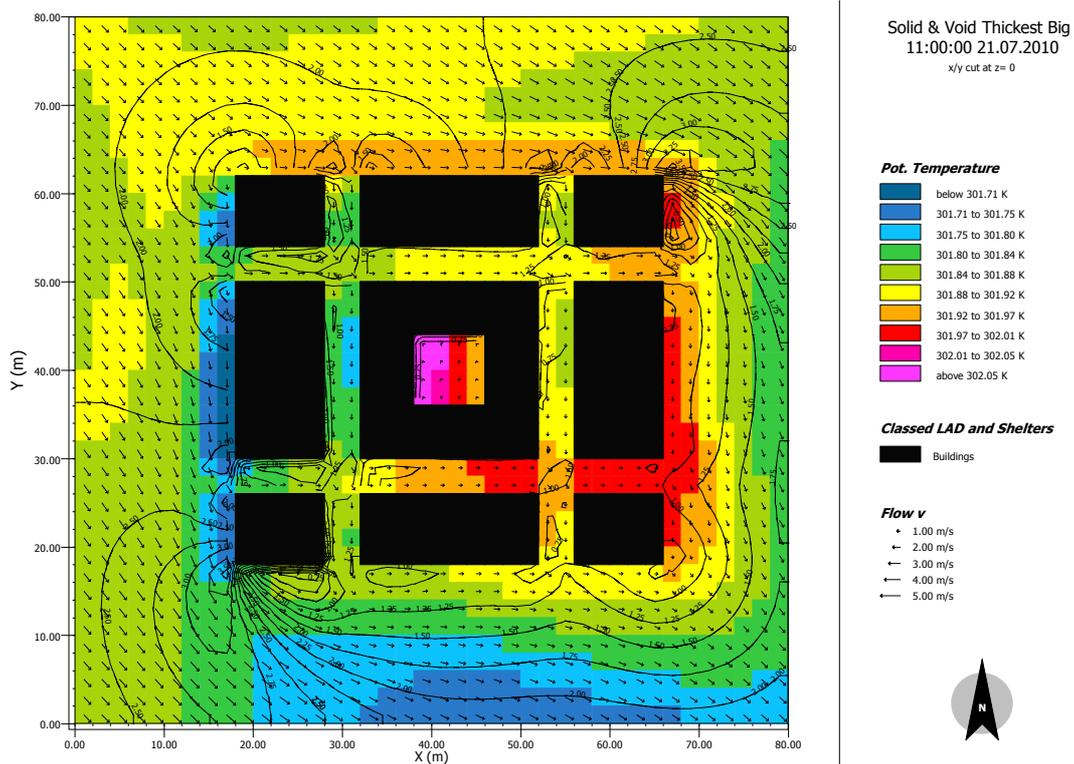
**Figure 4.2 (c)** Simulation results for thickest courtyard walls
