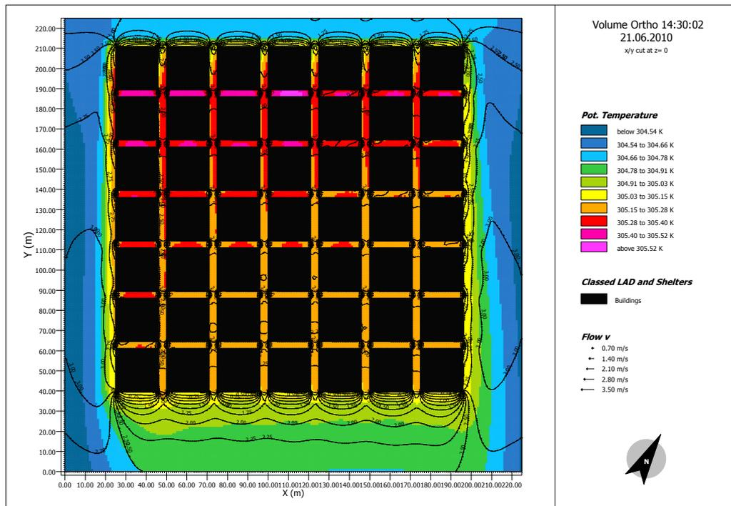
**Figure 5.18** Snapshot of temperature gradient in Volume Ortho at 14:30 in June showing high temperature occurring throughout the entire configuration (initial wind speed 3.6m/s).
