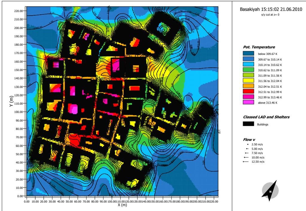
**Figure 5.21** Snapshot of temperature variation in Bastakiyah at 15:15 in June in absence of wind (0.1 m/s) showing the distribution of temperature throughout the configuration.
