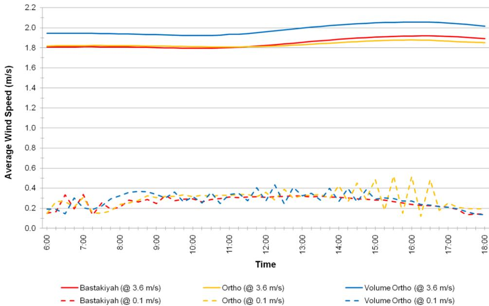
**Figure 5.2** Daily average wind speeds (m/s) for Bastakiyah, Ortho, and Volume Ortho configurations in June for both 3.6m/s and 0.1m/s initial wind speed scenarios.
