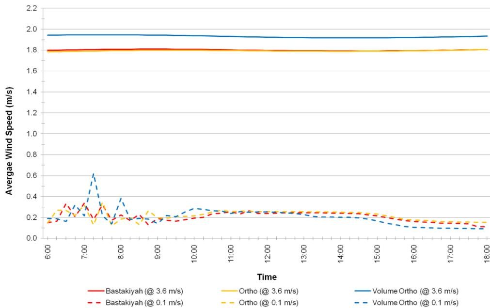
**Figure 5.4** Daily average wind speed (m/s) for Bastakiyah, Ortho, and Volume Ortho configurations in December for both 3.6m/s and 0.1m/s initial wind speed scenarios.
