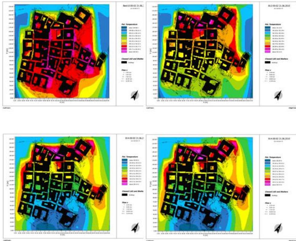
**Figure H.1** Temperature gradient for Bastakiyah in June and initial wind speed 7.0m/s
