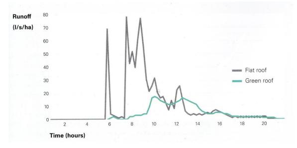
Figure3.1: runoff comparison between extensive green roof and conventional roof. (Dennett. & Kingsbury ,2008).
