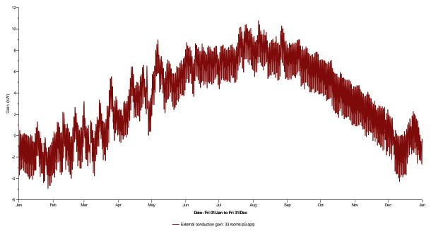
Figure 6.7: External conduction gain (case 2).
