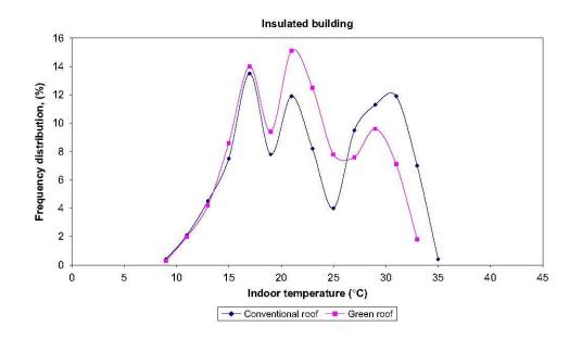
Figure 3.2: Distribution frequencies of green roof and conventional roof. (Santamourisa et al., 2007).
