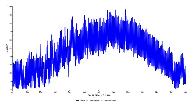
Figure 6.3: Cooling plant sensible load of the 16<sup>th</sup> floor(case 1).
