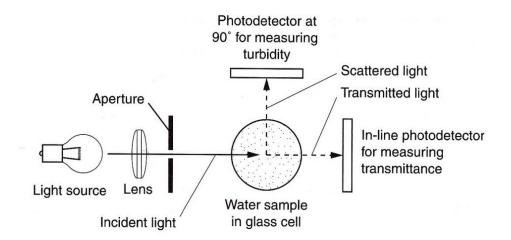
Figure4.1: Measuring turbidity and absorbance by spectrophotometer. (Crittenden, et al., 2005).
