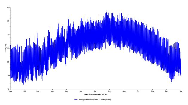
Figure 6.9: Cooling plant sensible load of the 16<sup>th</sup> floor(case 3).
