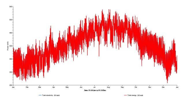
Figure 6.8: Total electricity and total energy consumption (case 3).
