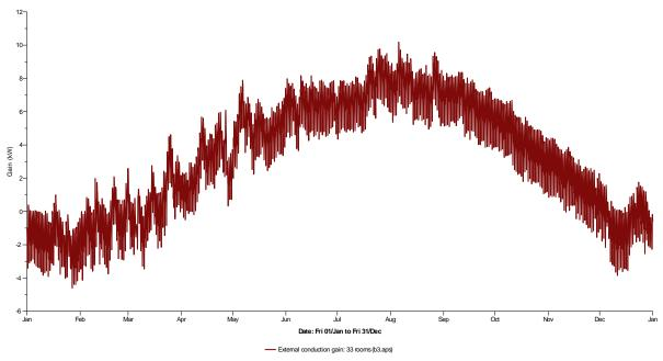
Figure 6.10: External conduction gain (case 3).
