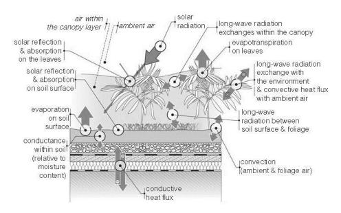
Figure 2.3: Green roof energy balance. (Theodosiou, 2009).
