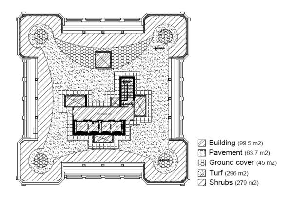
Figure 5.5: Green roof plan.
