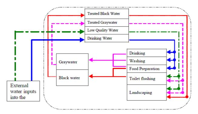
Figure 1.1: Water closed loop to be installed in a residential building. (Bakir,2001).
