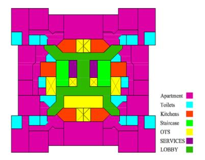
Figure 5.14: Thermal zoning diagram at typical floor.
