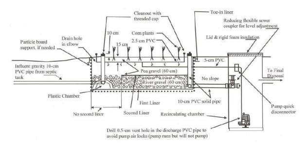
Figure 1.2: Section at recirculating vertical flow constructed wet land. (Garcia-Perez et al., 2011).
