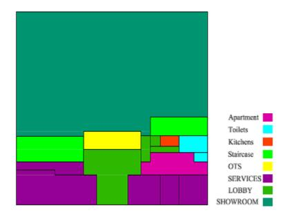
Figure 5.13: Thermal zoning diagram at ground floor.
