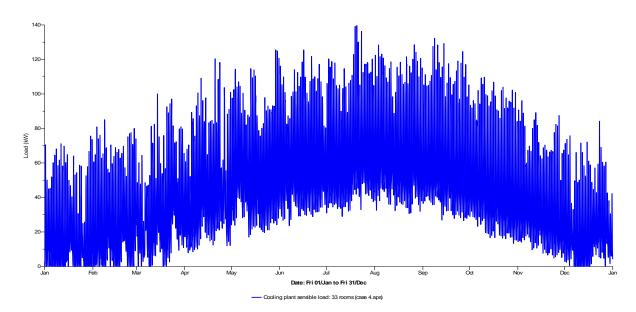
Figure 6.12: Cooling plant sensible load of the 16<sup>th</sup> floor(case 4).
