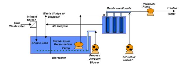
Figure 1.3: Membrane Bioreactors systems.(Fitzgerald, 2008).
