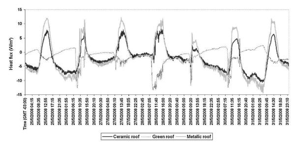
Figure 2.2: Heat flux in different types of roof. (Parizotto& Lamberts, 2011)
