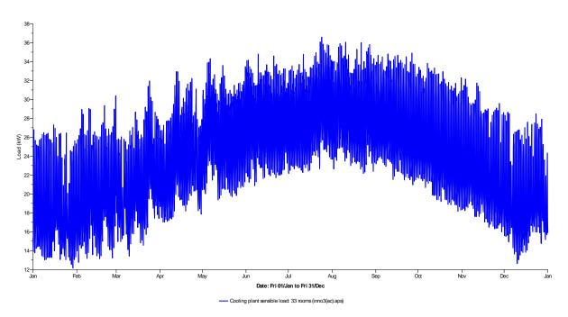
Figure 6.15: Cooling plant sensible load of the 16<sup>th</sup> floor(case 5).
