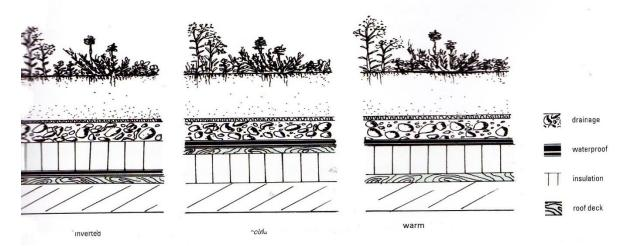
Figure 3.4: Roof construction types according to the insulation layer location. (Dennett, &Kingsbury, 2008).
