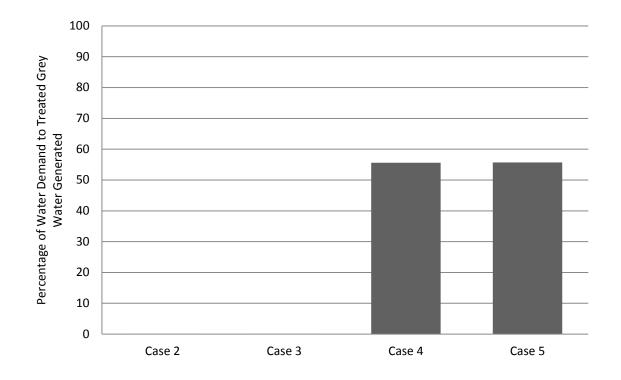
Figure 6.28: Percentage of water demand to treated grey water generated.
