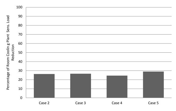
Figure 6.20: percentage of cooling load reduction of all cases.
