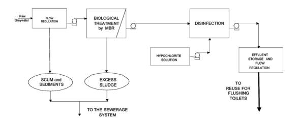
Figure 1.4: Membrane Bioreactors systems. (Friedler& Hadari, 2006).
