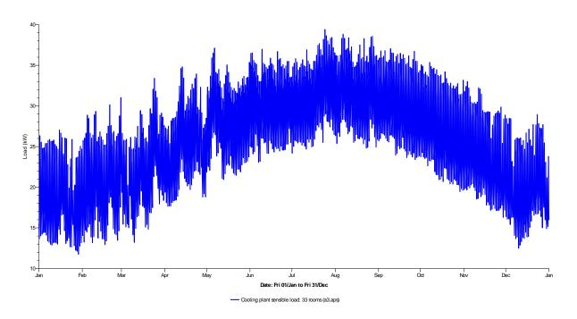
Figure 6.6: Cooling plant sensible load of the 16<sup>th</sup> floor(case 2).
