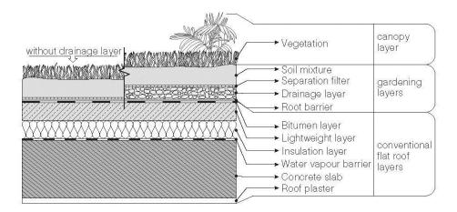
Figure 3.3: Typical structure for green roof. (Theodosiou, 2009).
