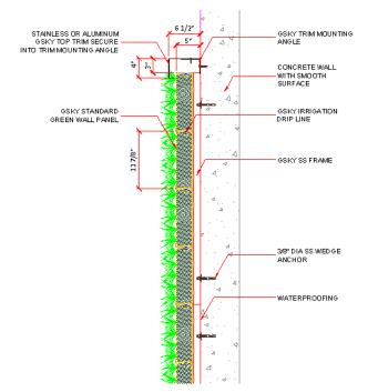
Figure 5.8: Green walls section. (GSKY Green Wall Panels, 2010).
